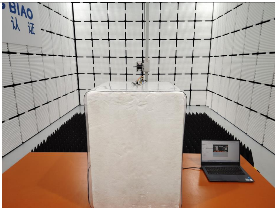
Radiated Emission Above 1GHz
