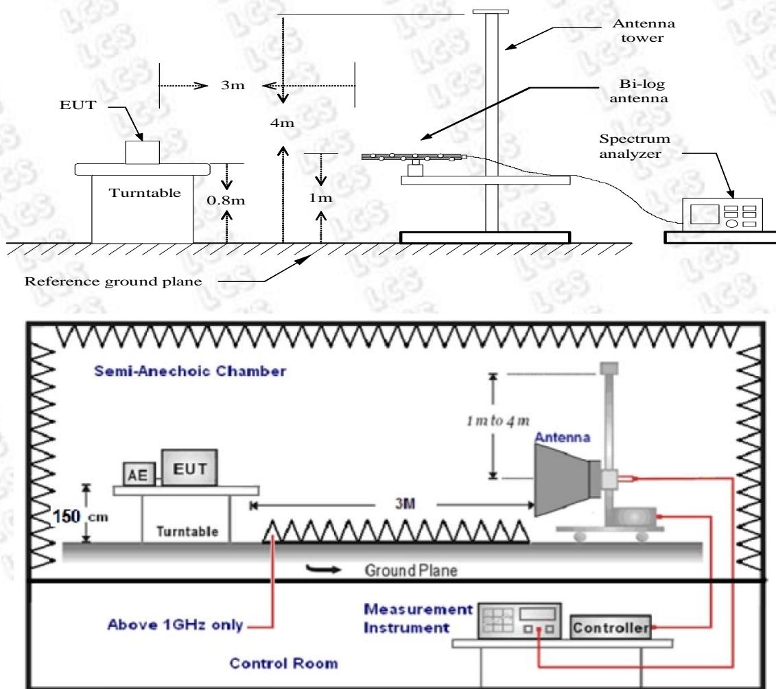
Above 10 GHz shall be extrapolated to the specified distance using an extrapolation factor of 20 dB/decade from 3m to 1.5m.
