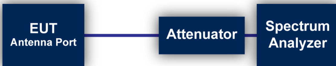
Figure 2: Direct Connection at the Antenna Port Test
