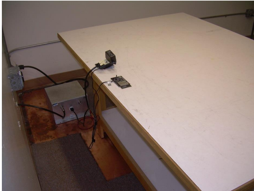
Photograph 7 – Back View Conducted Emissions Worst-Case Configuration
