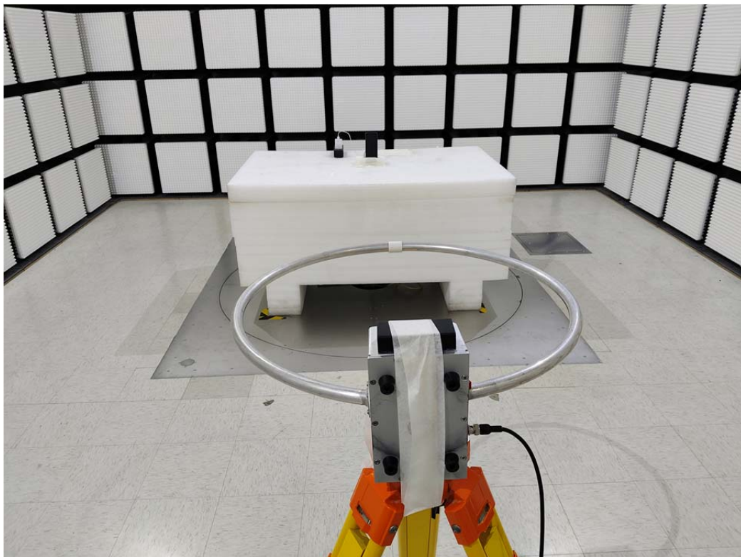
Radiated Emission 9 kHz-30 MHz Ground-parallel View
