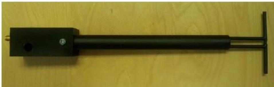
**Figure 1 – MVG COMOSAR Validation Dipole**
