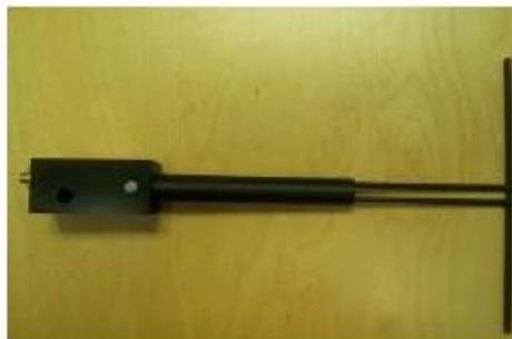
**Figure 1 – MVG COMOSAR Validation Dipole**
