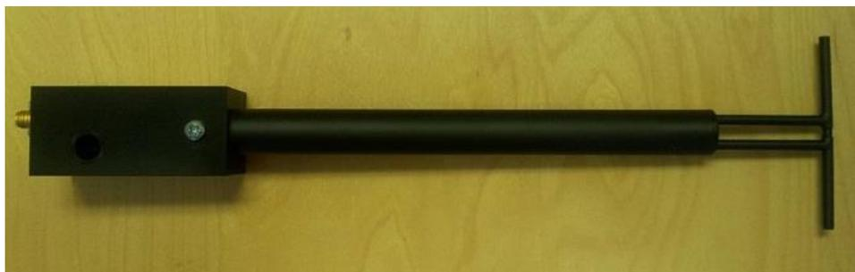
**Figure 1 – MVG COMOSAR Validation Dipole**
