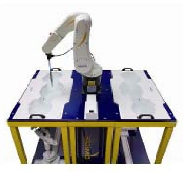
The EUT under test operating at the maximum power level is placed in the phone holder, under the phantom, which is filled with head simulating liquid. The E-Field probe measures the electric field inside the phantom. The OpenSAR software computes the results to give a SAR value in a 1g or 10g mass.
