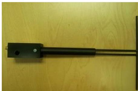
**Figure 1 – MVG COMOSAR Validation Dipole**
