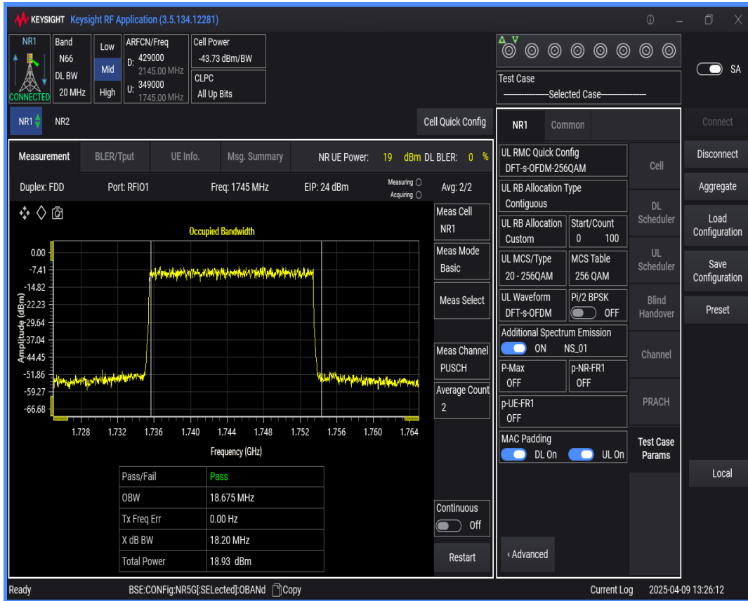
n66 SCS=15kHz DFT_QAM256 BW=40MHz Channel=349000 RB=216@0
