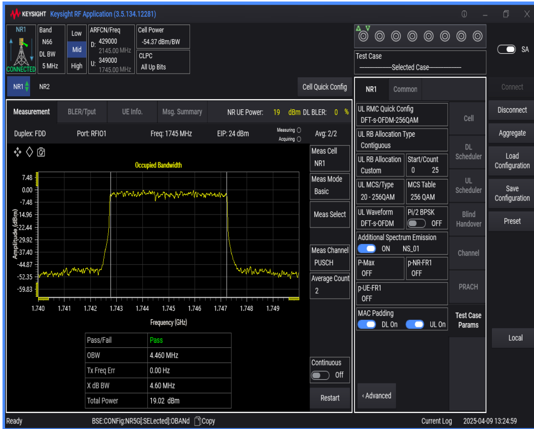
n66 SCS=15kHz DFT_QAM64 BW=15MHz Channel=349000 RB=75@0
