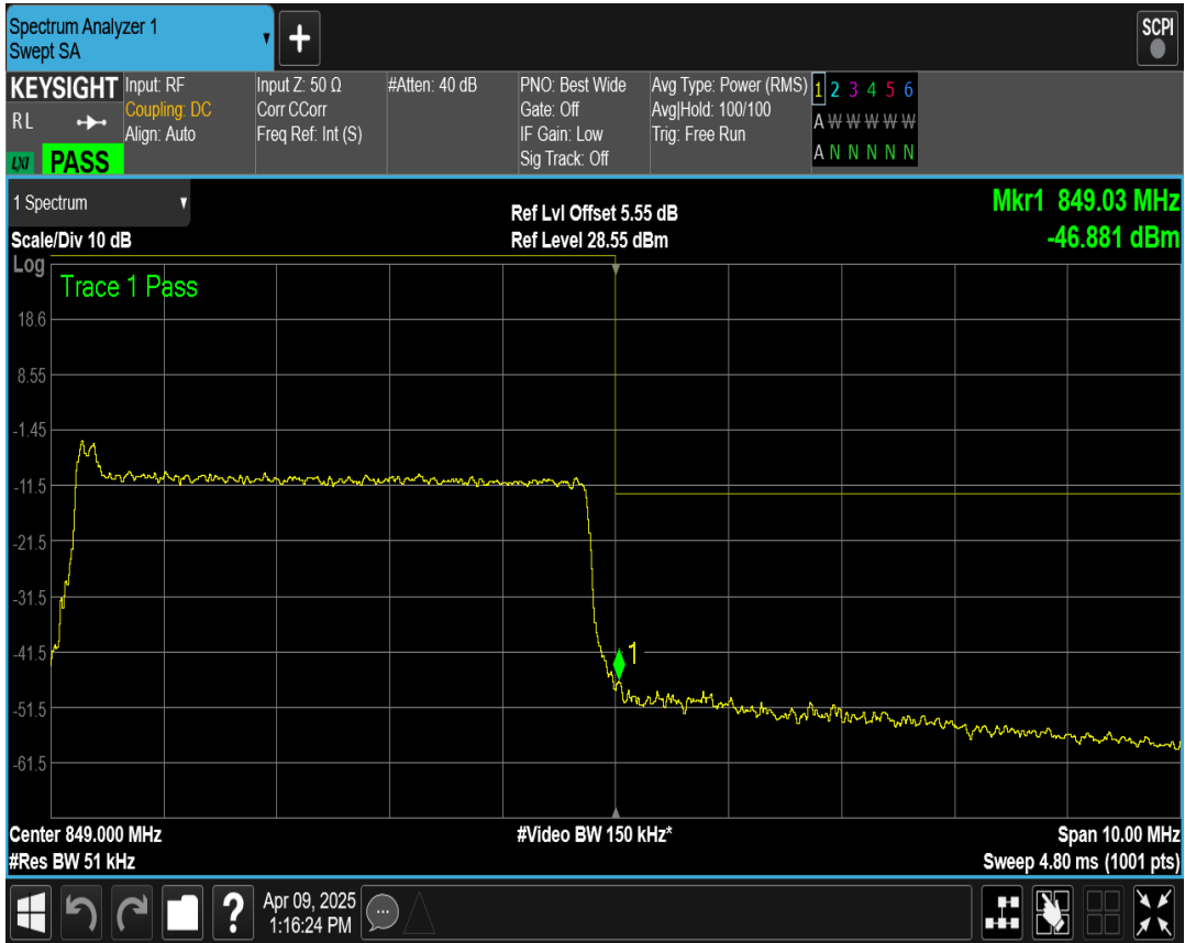
n5 SCS=15kHz CP_QPSK BW=5MHz Channel=169300 RB=1@24
