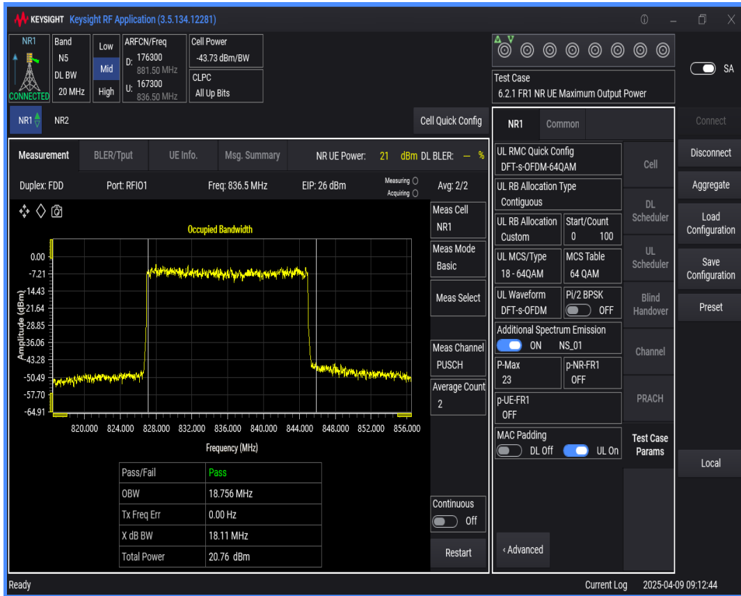
n5 SCS=15kHz DFT_QAM64 BW=15MHz Channel=167300 RB=75 @0
