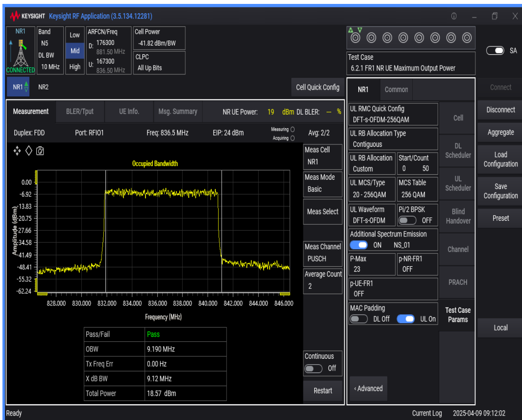
n5 SCS=15kHz DFT_QAM16 BW=5MHz Channel=167300 RB=25@0
