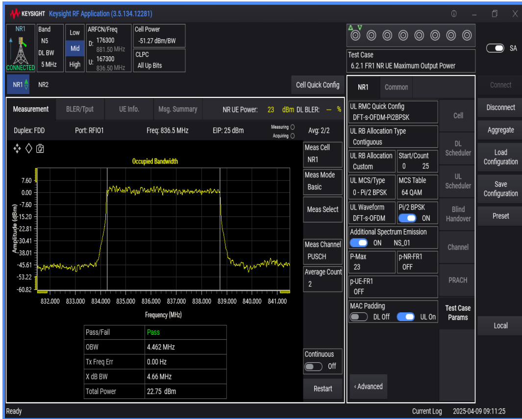
n5 SCS=15kHz DFT_QAM16 BW=15MHz Channel=167300 RB=75@0
