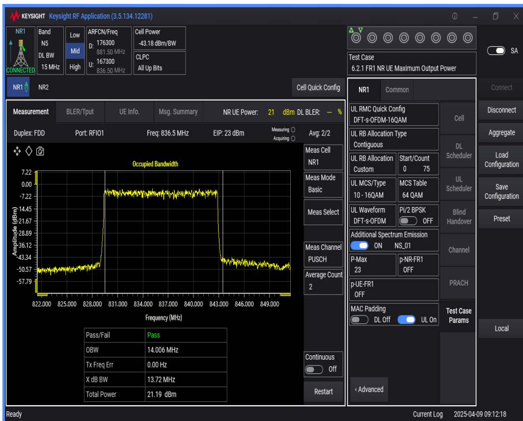
n5 SCS=15kHz DFT_QAM16 BW=20MHz Channel=167300 RB=100@0
