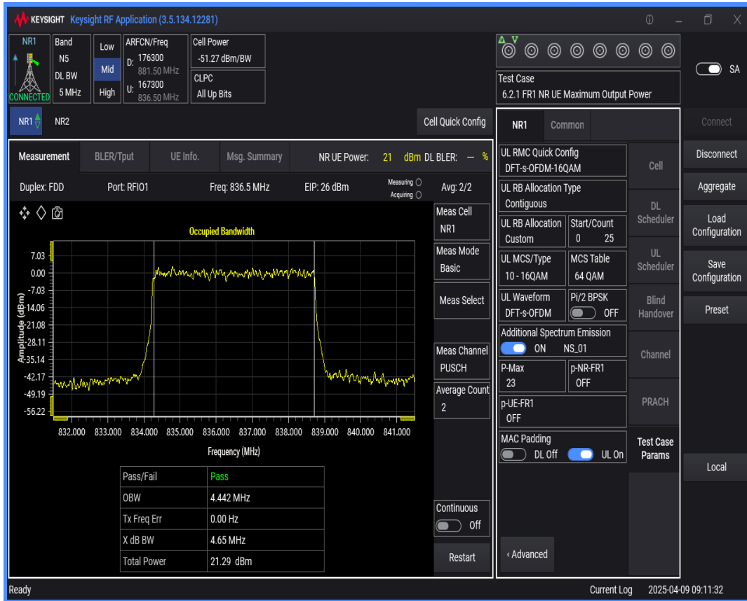
n5 SCS=15kHz DFT_QAM256 BW=15MHz Channel=167300 RB=75@0
