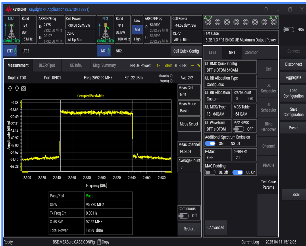
n41 SCS=30kHz DFT_QAM64 BW=50MHz Channel=518598 RB=128@0
