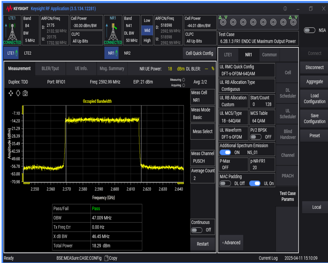
n41 SCS=30kHz DFT_QAM64 BW=40MHz Channel=518598 RB=100@0
