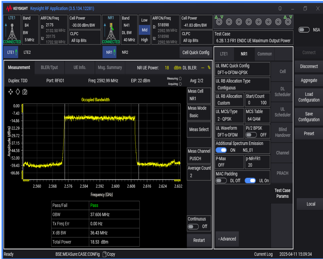
n41 SCS=30kHz DFT_QPSK BW=60MHz Channel=518598 RB=162@0
