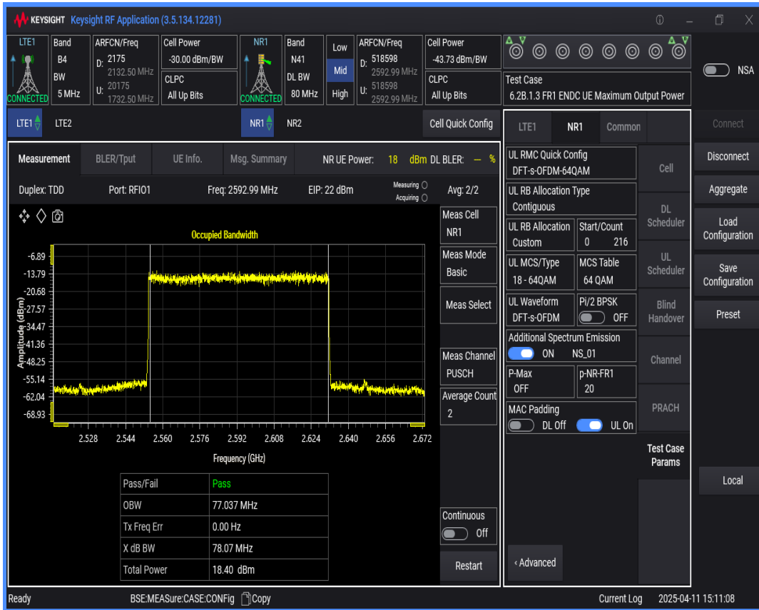
n41 SCS=30kHz DFT_QAM64 BW=60MHz Channel=518598 RB=162 @0
