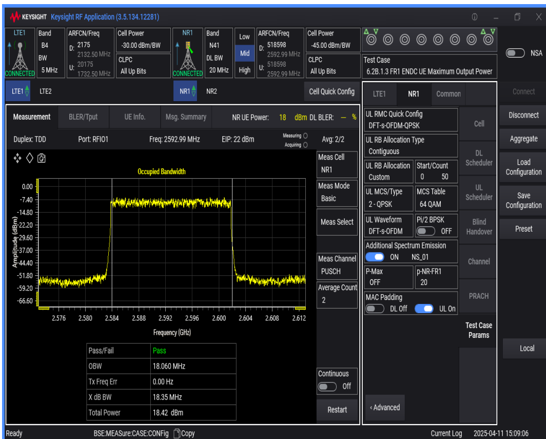
n41 SCS=30kHz DFT_QPSK BW=100MHz Channel=518598 RB=270@0
