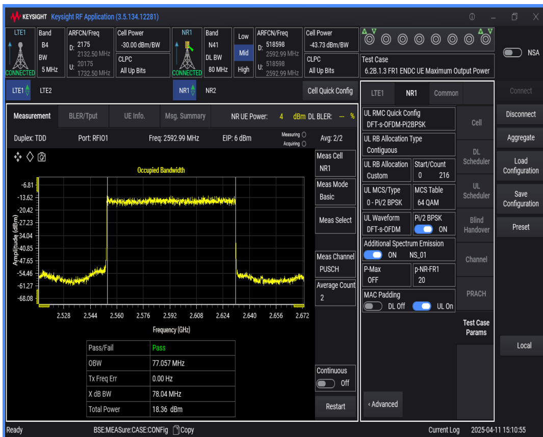
n41 SCS=30kHz DFT_BPSK BW=90MHz Channel=518598 RB=240@0
