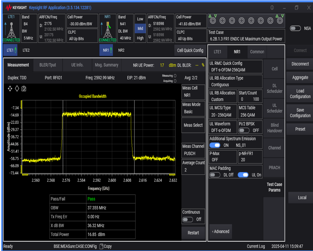
n41 SCS=30kHz DFT_QAM256 BW=80MHz Channel=518598 RB=216 @0
