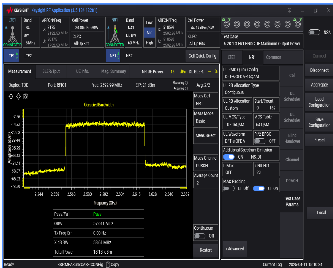
n41 SCS=30kHz DFT_QAM16 BW=20MHz Channel=518598 RB=50 @0
