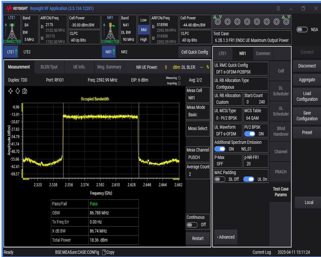
n41 SCS=30kHz DFT_BPSK BW=50MHz Channel=518598 RB=128@0
