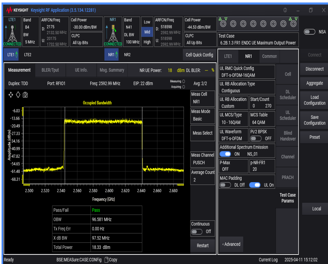
n41 SCS=30kHz DFT_QAM16 BW=50MHz Channel=518598 RB=128@0
