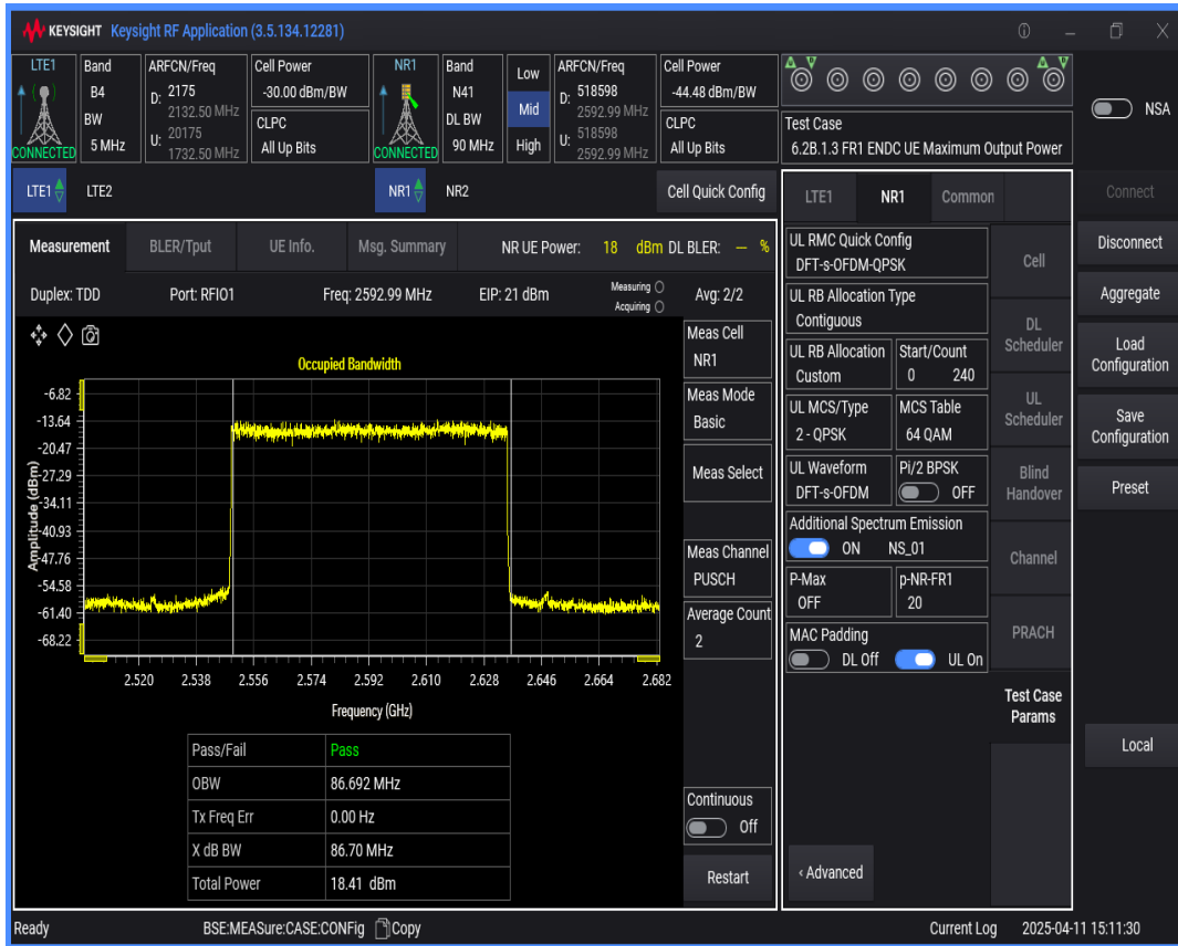
n41 SCS=30kHz DFT_QPSK BW=80MHz Channel=518598 RB=216@0
