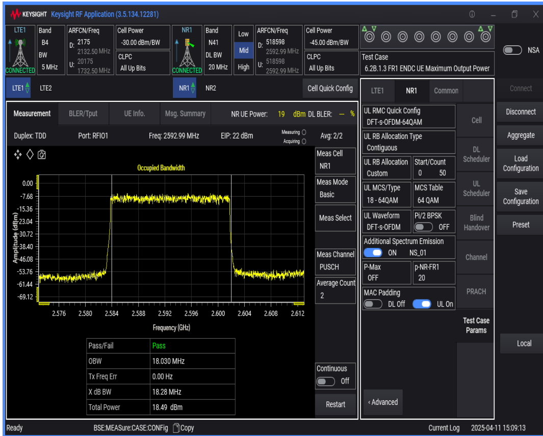
n41 SCS=30kHz DFT_QAM64 BW=100MHz Channel=518598 RB=270@0
