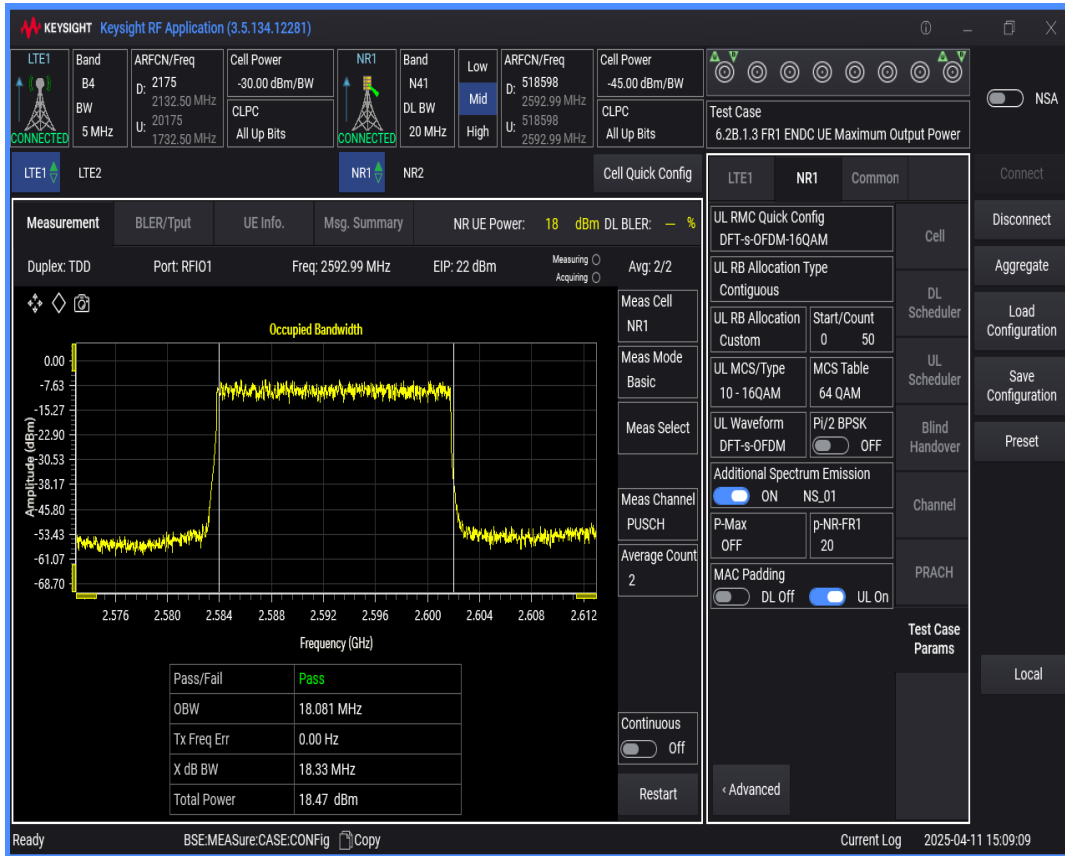
n41 SCS=30kHz DFT_QAM16 BW=100MHz Channel=518598 RB=270@0
