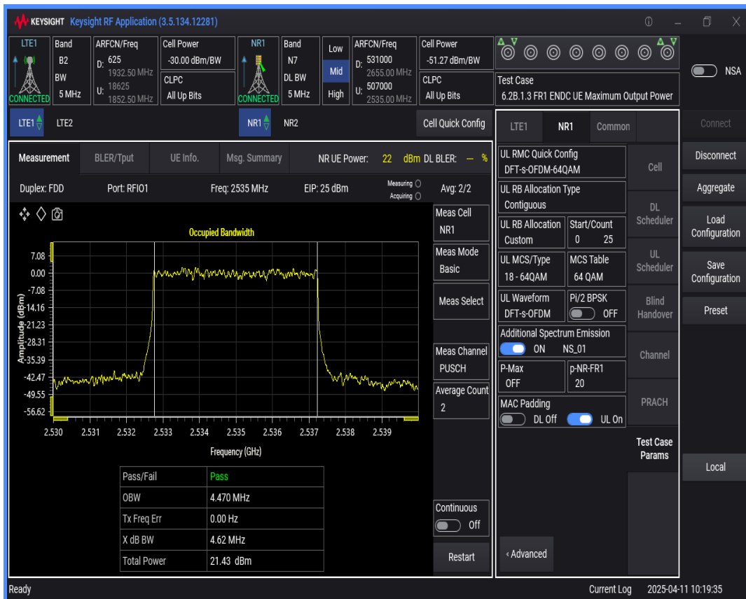
n7 SCS=30kHz DFT_QAM16 BW=20MHz Channel=507000 RB=50 @0
