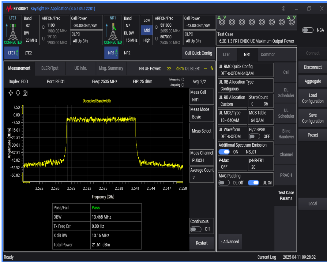
n7 SCS=30kHz DFT_QAM64 BW=10MHz Channel=507000 RB=24@0
