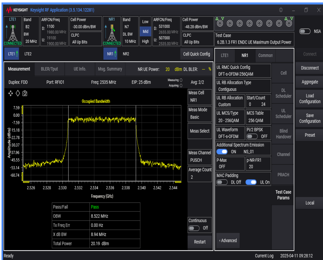
n7 SCS=30kHz DFT_QAM256 BW=15MHz Channel=507000 RB=36@0
