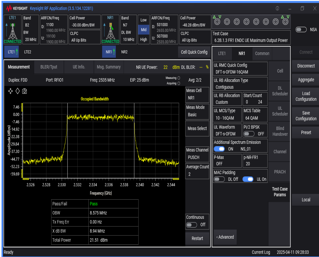
n7 SCS=30kHz DFT_QAM16 BW=15MHz Channel=507000 RB=36@0
