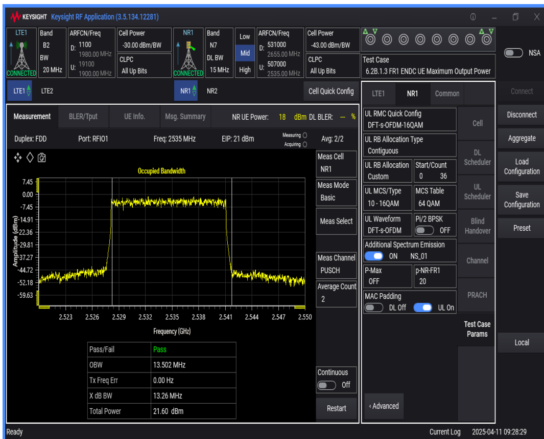
n7 SCS=30kHz DFT_QAM64 BW=15MHz Channel=507000 RB=36@0
