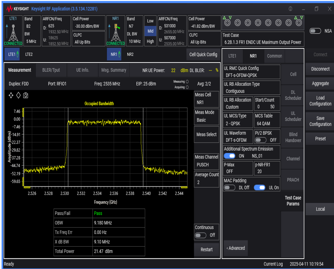
n7 SCS=15kHz DFT_QAM64 BW=5MHz Channel=507000 RB=25 @0
