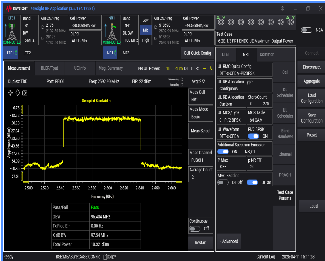
n41 SCS=30kHz DFT_BPSK BW=50MHz Channel=518598 RB=128@0
