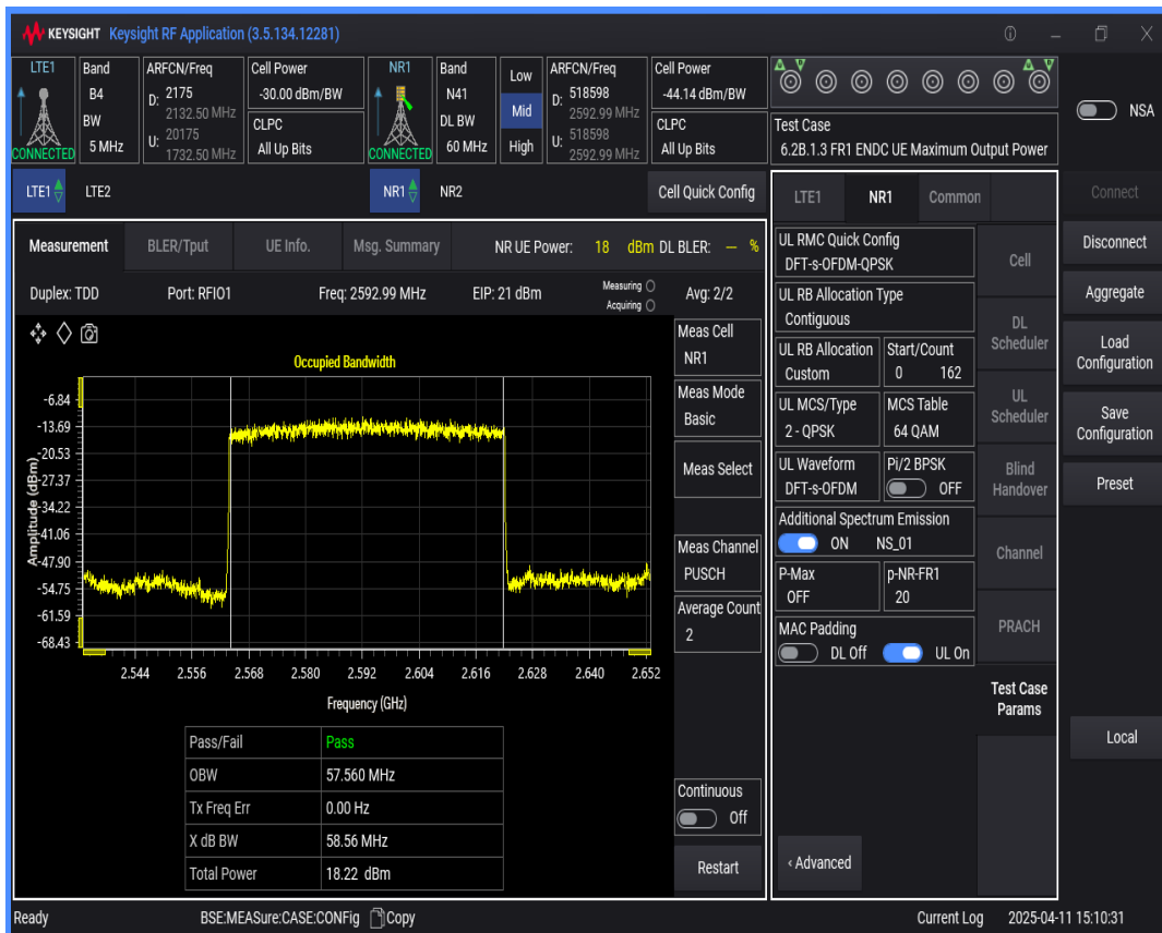
n41 SCS=30kHz DFT_QPSK BW=80MHz Channel=518598 RB=216 @0
