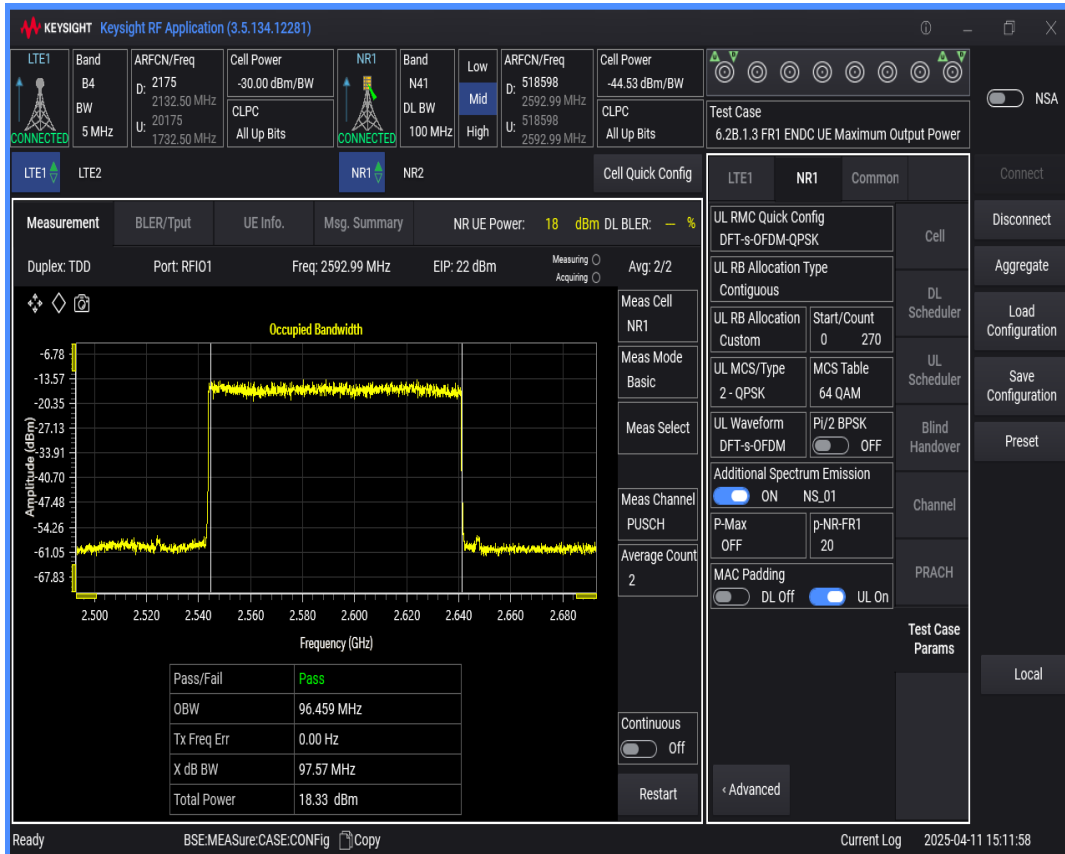
n41 SCS=30kHz DFT_QAM64 BW=90MHz Channel=518598 RB=240@0
