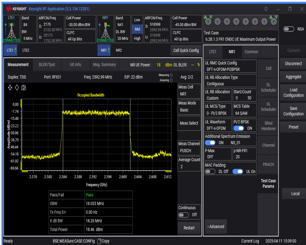
n41 SCS=30kHz DFT_BPSK BW=100MHz Channel=518598 RB=270@0
