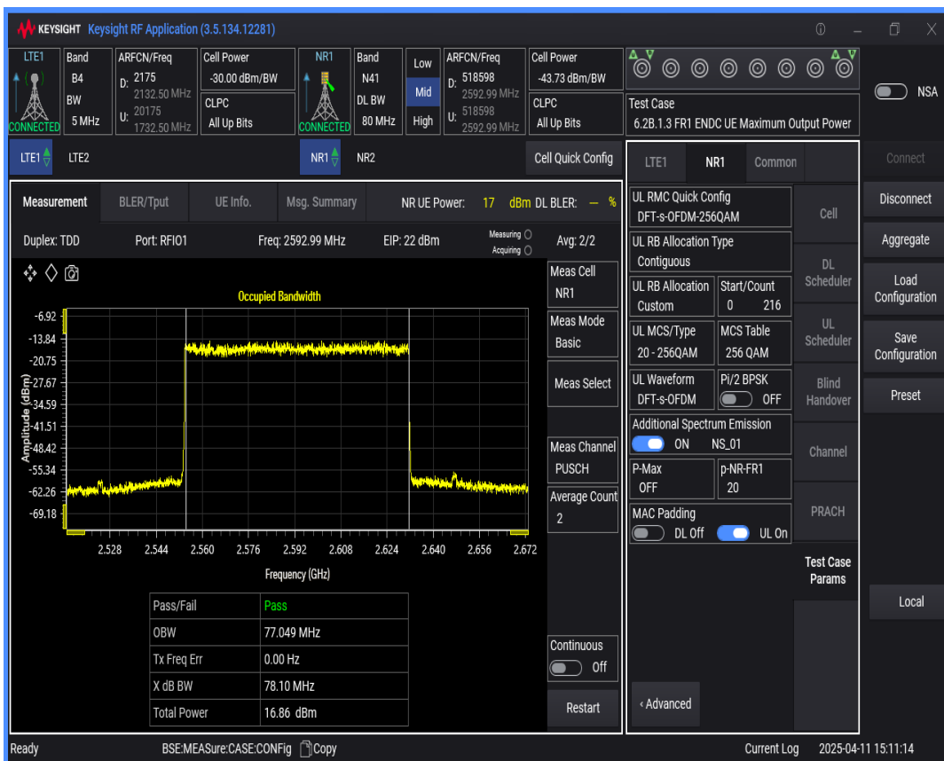
n41 SCS=30kHz DFT_QAM64 BW=100MHz Channel=518598 RB=270@0
