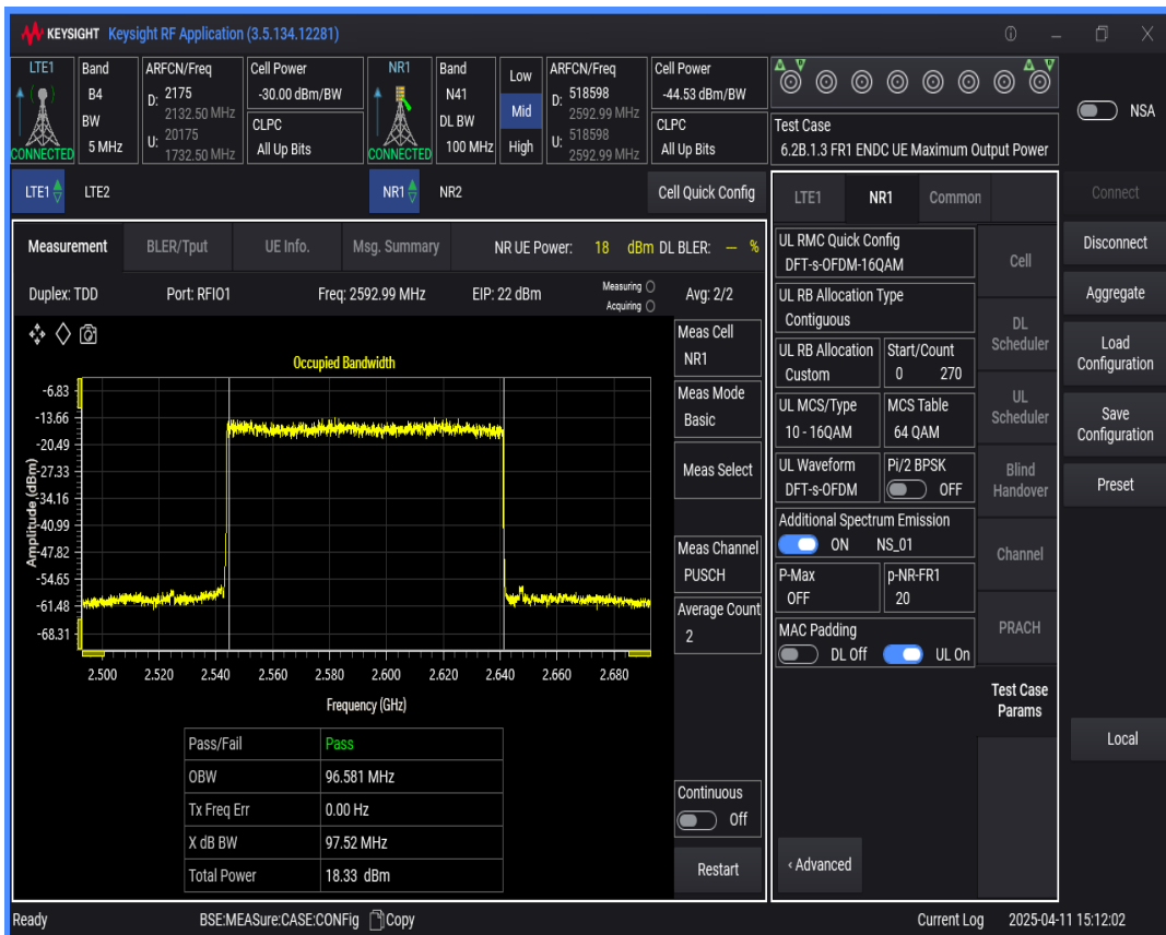
n41 SCS=30kHz DFT_BPSK BW=60MHz Channel=518598 RB=162@0
