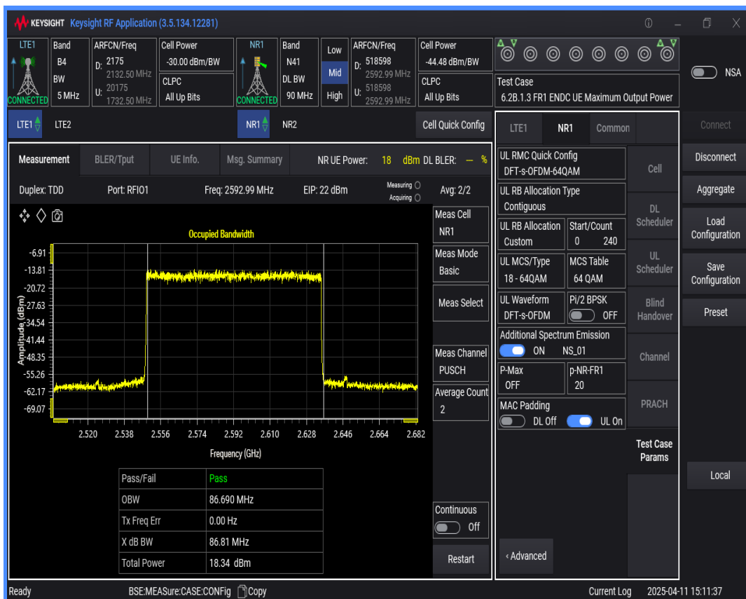
n41 SCS=30kHz DFT_QAM256 BW=90MHz Channel=518598 RB=240@0
