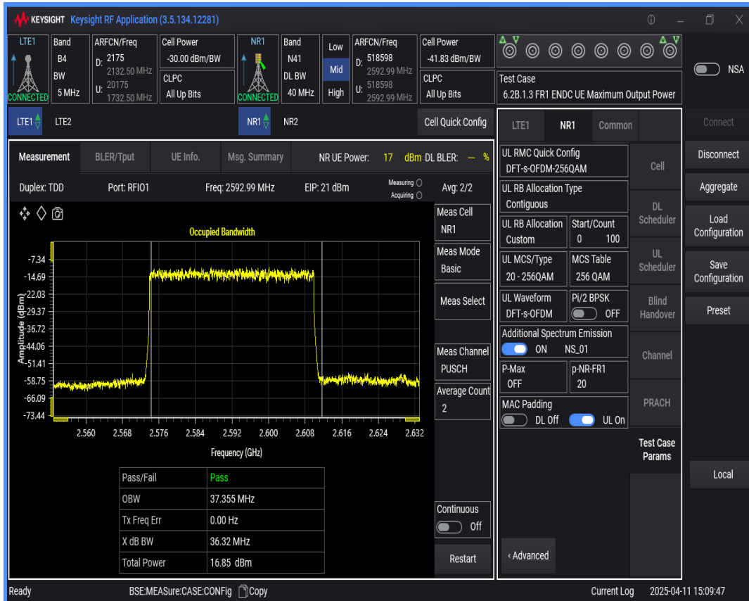
n41 SCS=30kHz DFT_QAM256 BW=50MHz Channel=518598 RB=128 @0
