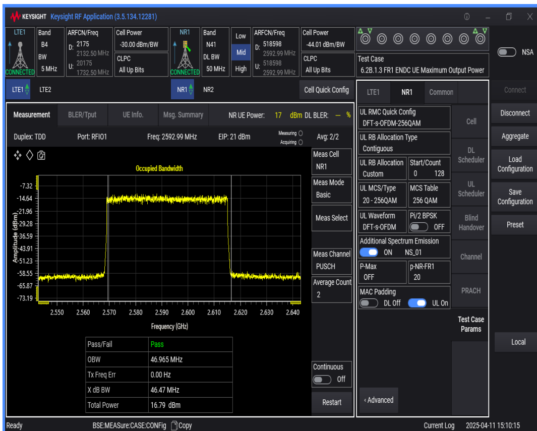
n41 SCS=30kHz DFT_QAM256 BW=60MHz Channel=518598 RB=162 @0
