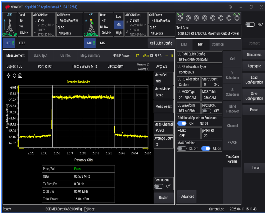
n41 SCS=30kHz DFT_QAM256 BW=80MHz Channel=518598 RB=216@0
