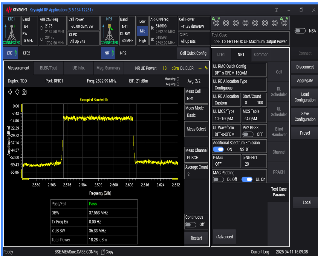
n41 SCS=30kHz DFT_QAM256 BW=40MHz Channel=518598 RB=100@0
