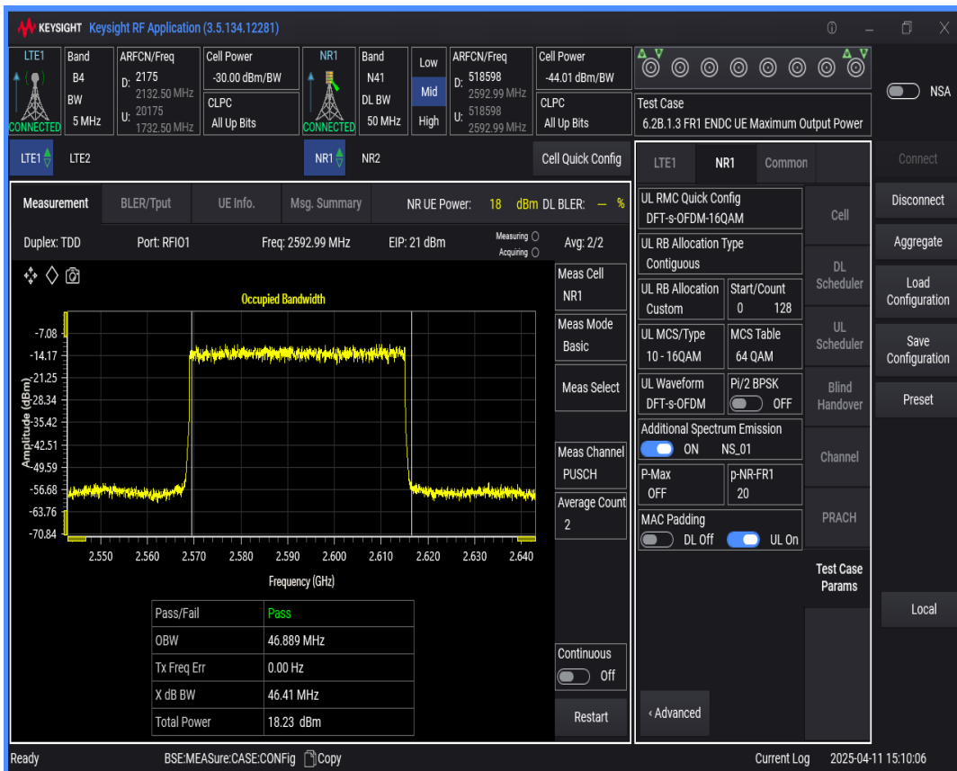
n41 SCS=30kHz DFT_QAM16 BW=40MHz Channel=518598 RB=100@0
