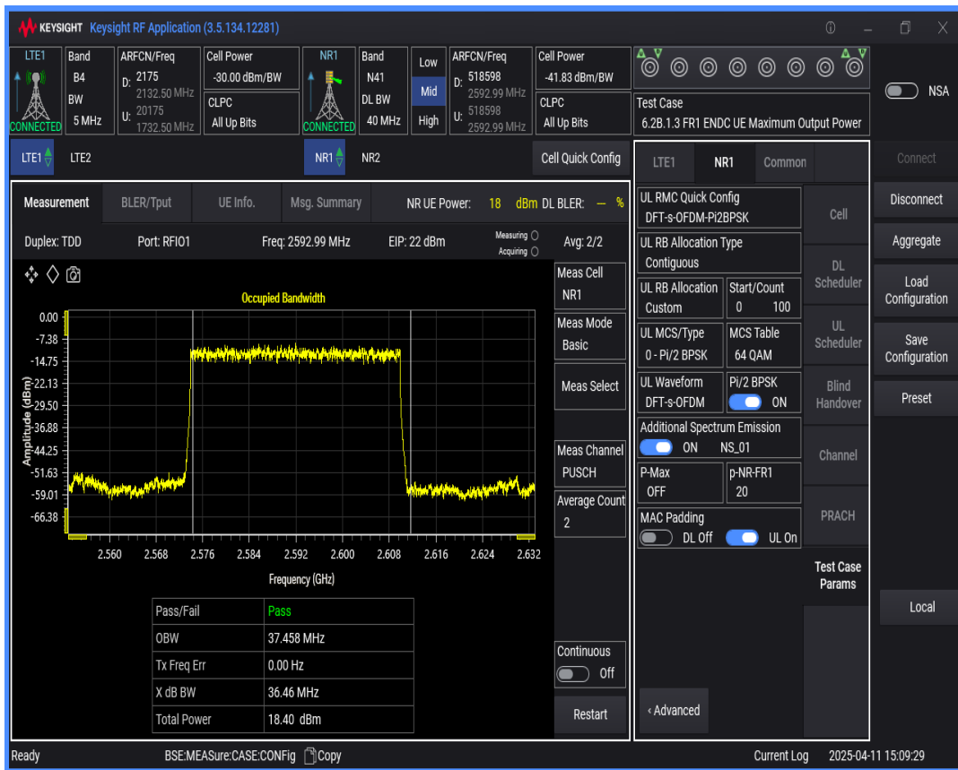
n41 SCS=30kHz DFT_QAM16 BW=60MHz Channel=518598 RB=162 @0
