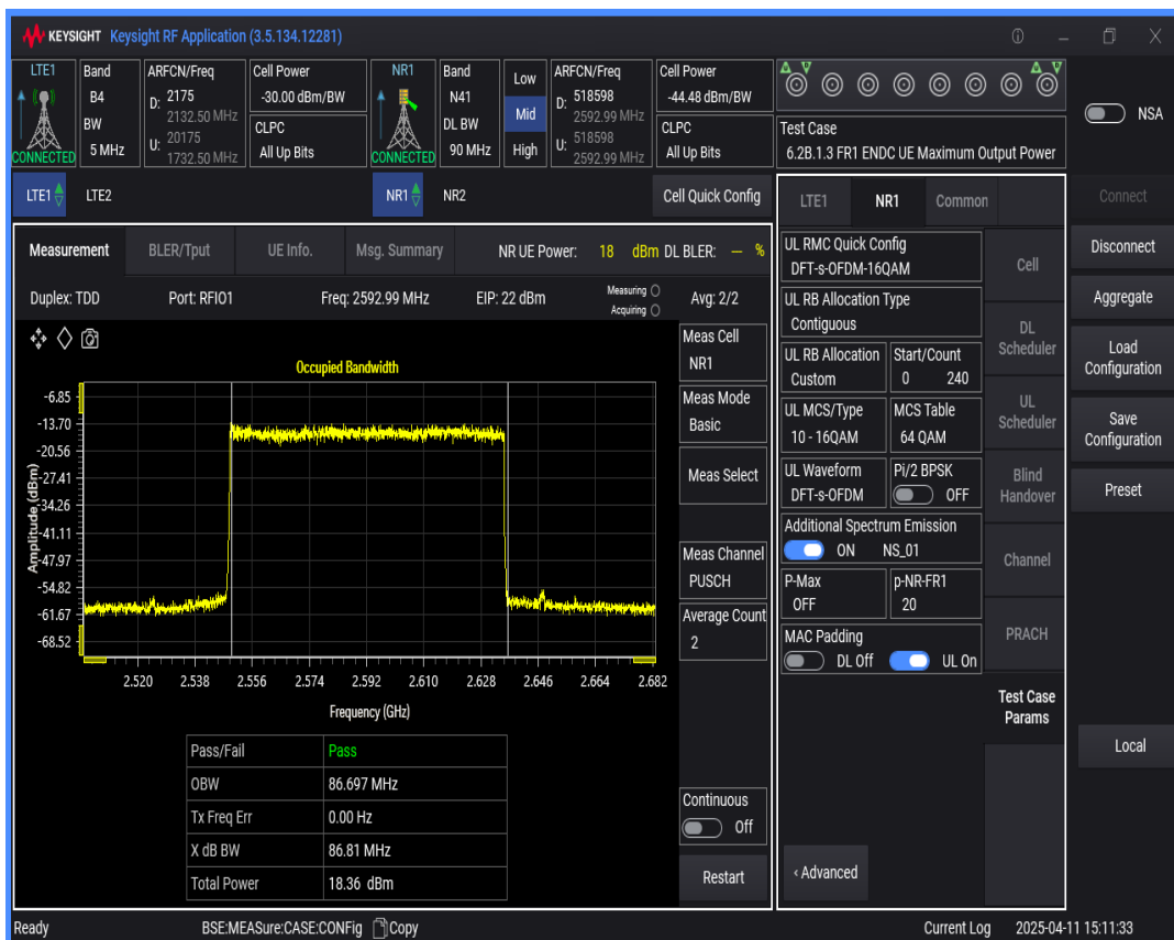
n41 SCS=30kHz DFT_QAM256 BW=100MHz Channel=518598 RB=270 @0
