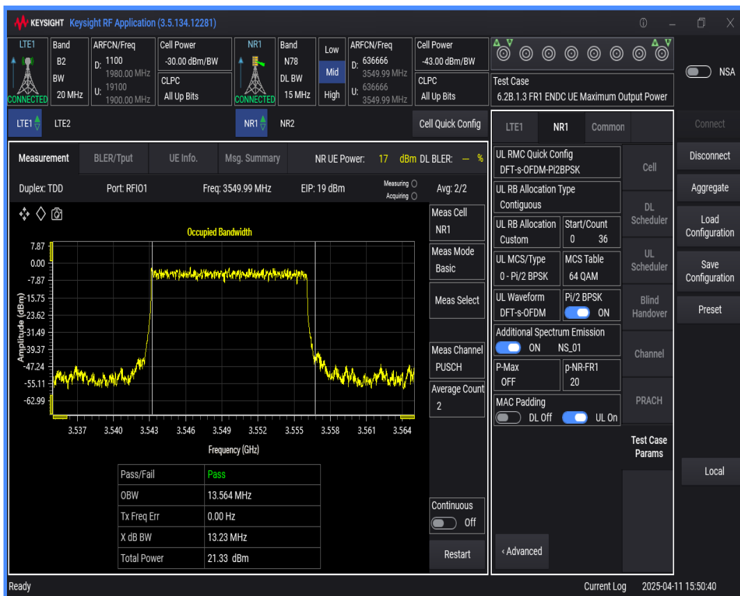
n78 SCS=30kHz DFT_QAM16 BW=15MHz Channel=636666 RB=36@0
