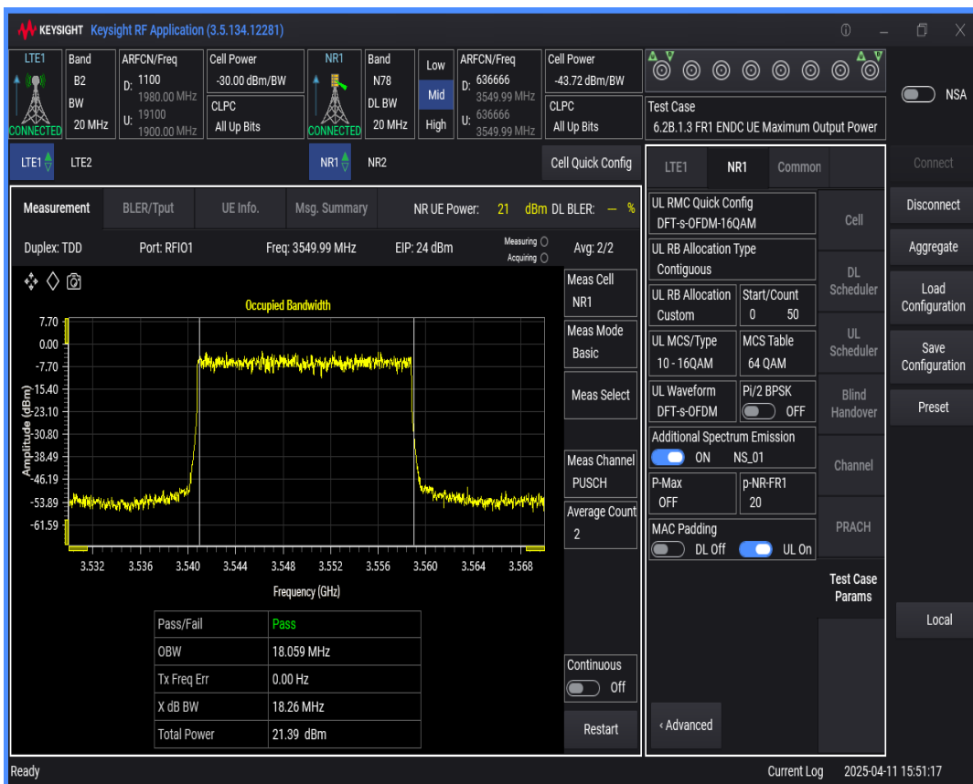
n78 SCS=30kHz DFT_QAM16 BW=100MHz Channel=636666 RB=270@0
