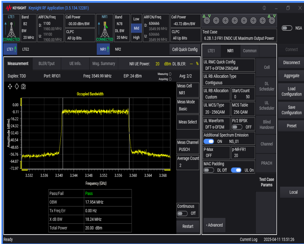
n78 SCS=30kHz DFT_QAM64 BW=100MHz Channel=636666 RB=270@0
