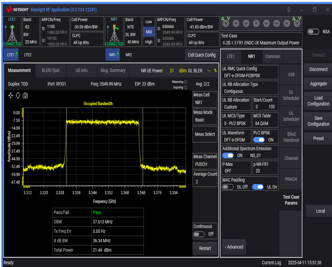
n78 SCS=30kHz DFT_BPSK BW=10MHz Channel=636666 RB=24@0
