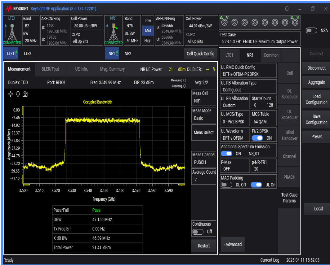
n78 SCS=30kHz DFT_BPSK BW=90MHz Channel=636666 RB=240@0
