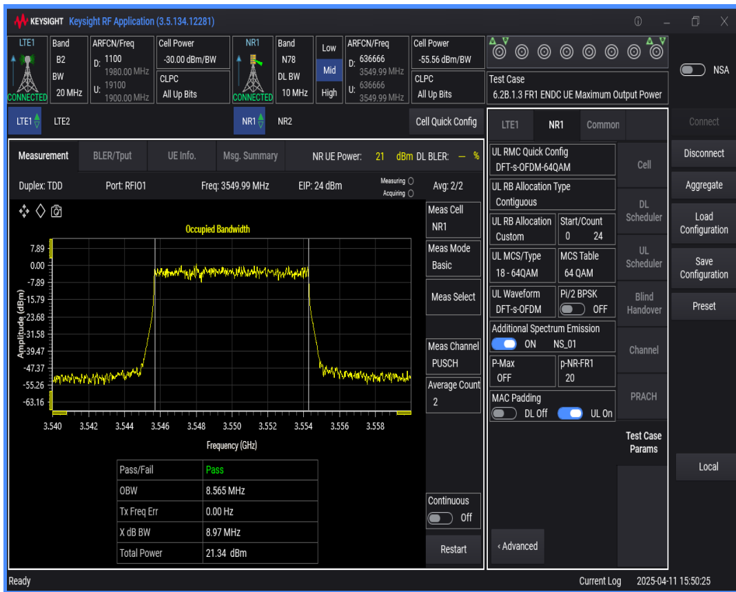
n78 SCS=30kHz DFT_QAM256 BW=90MHz Channel=636666 RB=240@0
