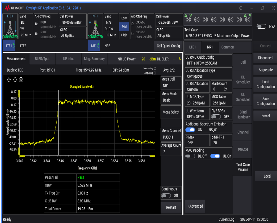
n78 SCS=30kHz DFT_QAM16 BW=50MHz Channel=636666 RB=128@0
