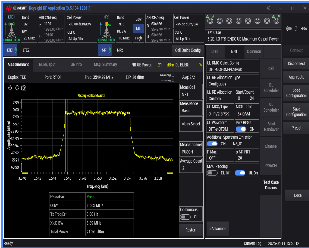
n78 SCS=30kHz DFT_BPSK BW=15MHz Channel=636666 RB=36@0
