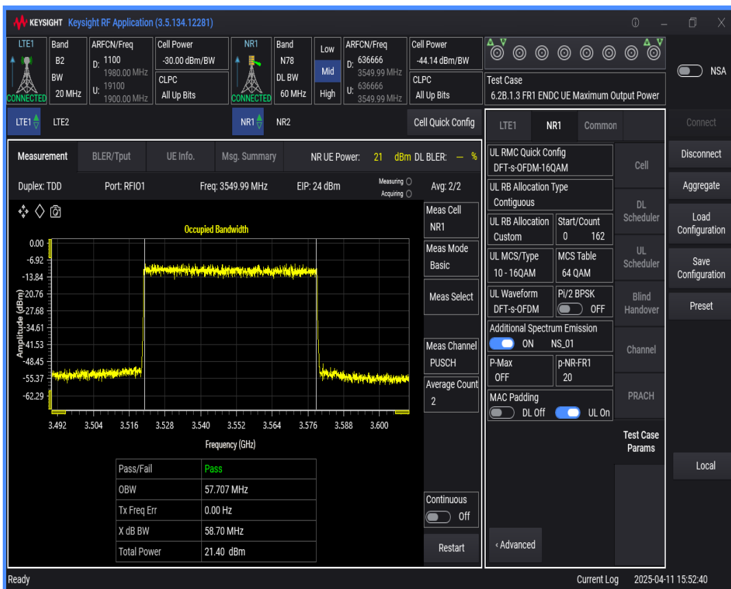
n78 SCS=30kHz DFT_QAM16 BW=80MHz Channel=636666 RB=216 @0
