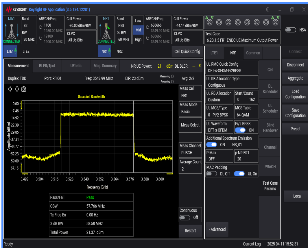
n78 SCS=30kHz DFT_BPSK BW=50MHz Channel=636666 RB=128 @0
