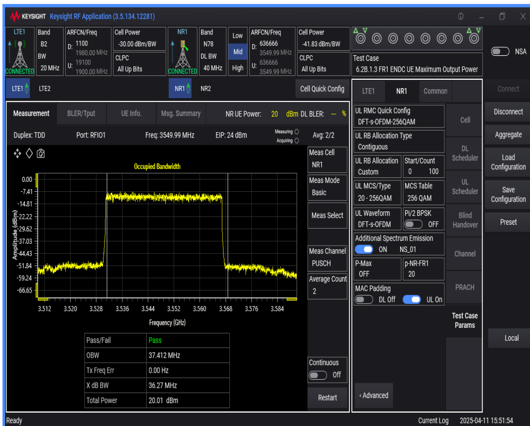
n78 SCS=30kHz DFT_QAM256 BW=50MHz Channel=636666 RB=128@0
