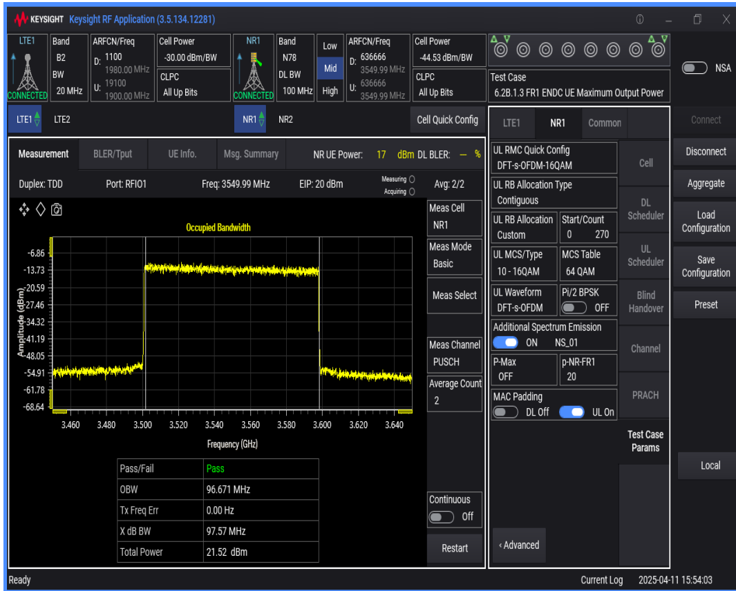
n78 SCS=30kHz DFT_BPSK BW=60MHz Channel=636666 RB=162 @0
