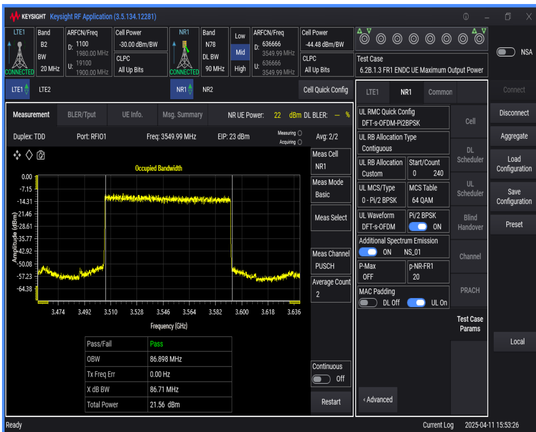
n78 SCS=30kHz DFT_BPSK BW=80MHz Channel=636666 RB=216@0
