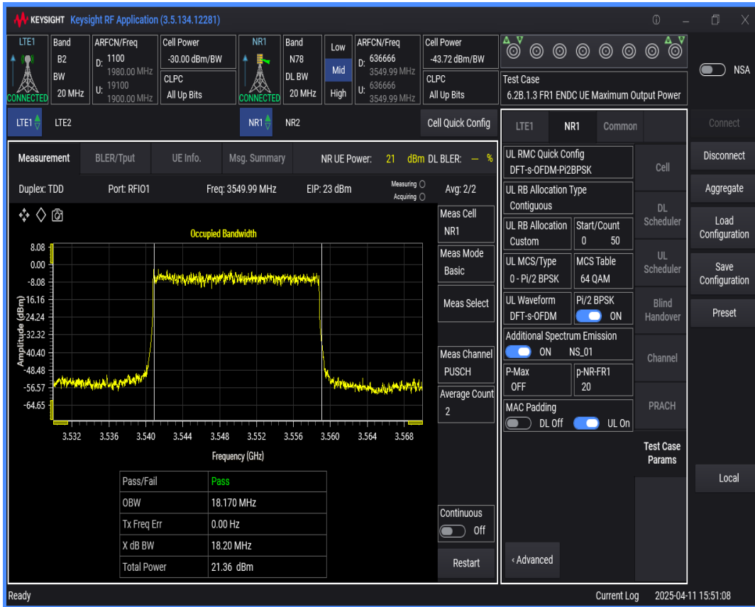
n78 SCS=30kHz DFT_BPSK BW=40MHz Channel=636666 RB=100@0
