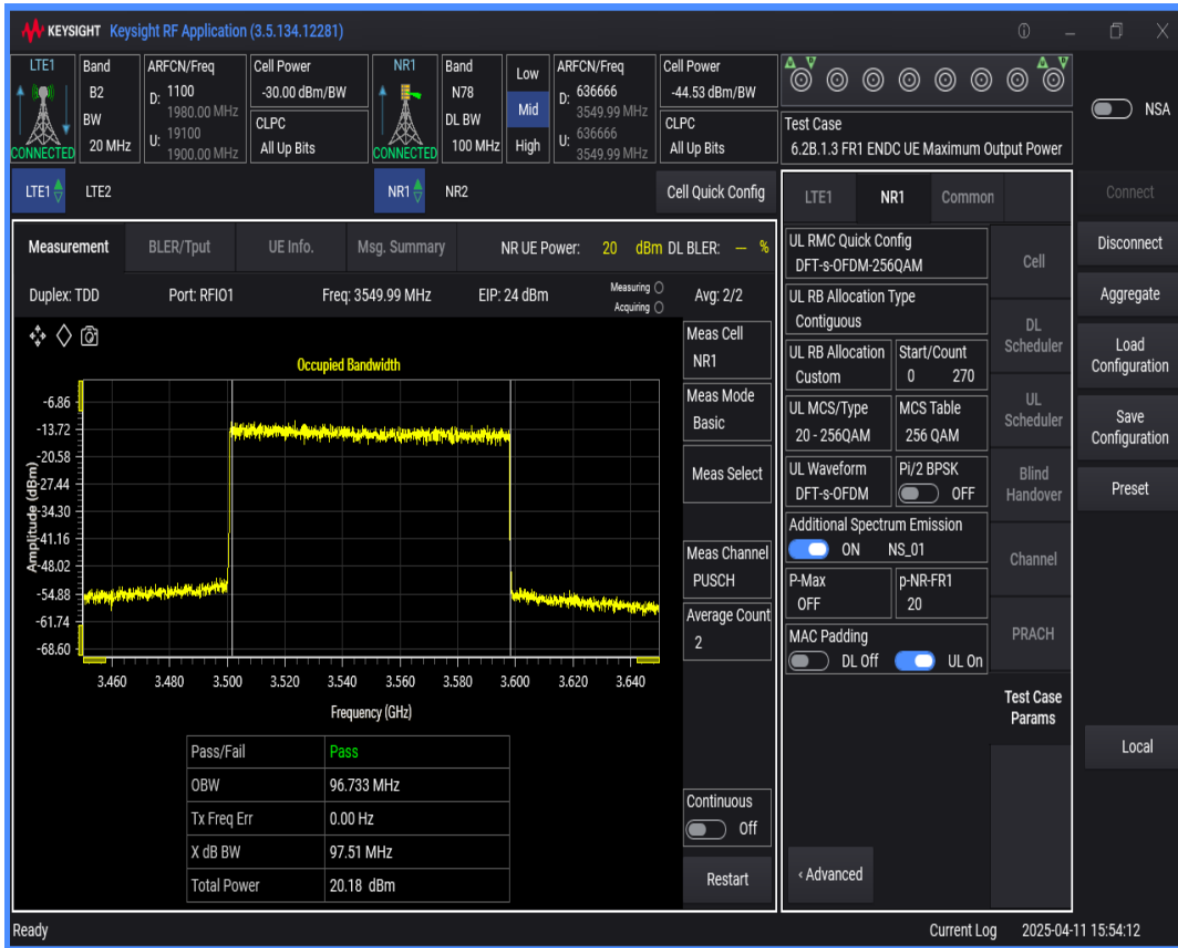
n78 SCS=30kHz DFT_QAM256 BW=10MHz Channel=636666 RB=24@0
