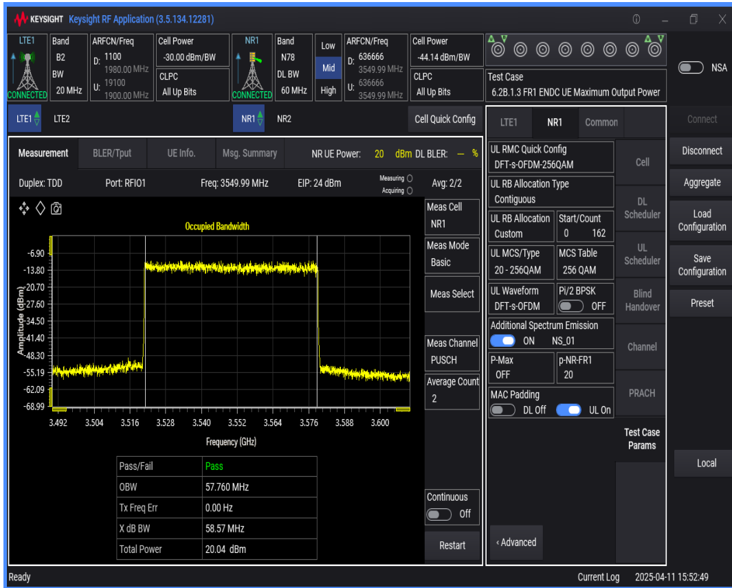
n78 SCS=30kHz DFT_QAM256 BW=80MHz Channel=636666 RB=216@0
