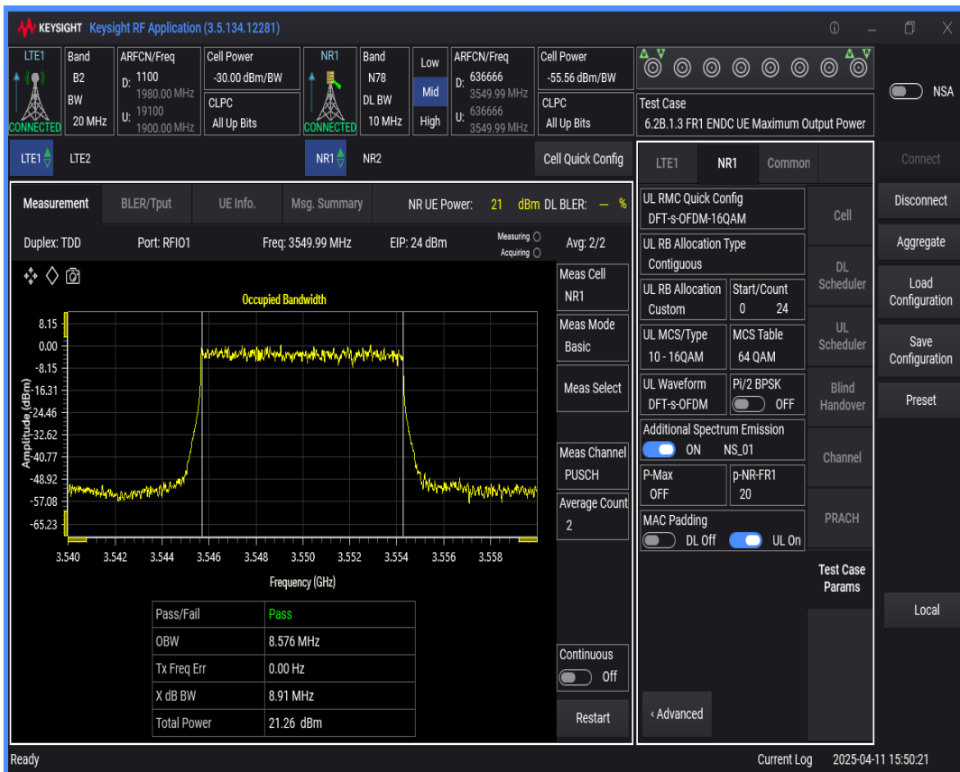
n78 SCS=30kHz DFT_QAM16 BW=40MHz Channel=636666 RB=100@0
