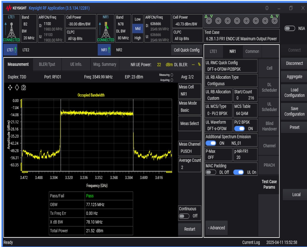
n78 SCS=30kHz DFT_QAM16 BW=90MHz Channel=636666 RB=240 @0
