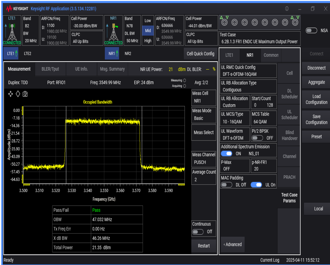
n78 SCS=30kHz DFT_QAM16 BW=60MHz Channel=636666 RB=162 @0
