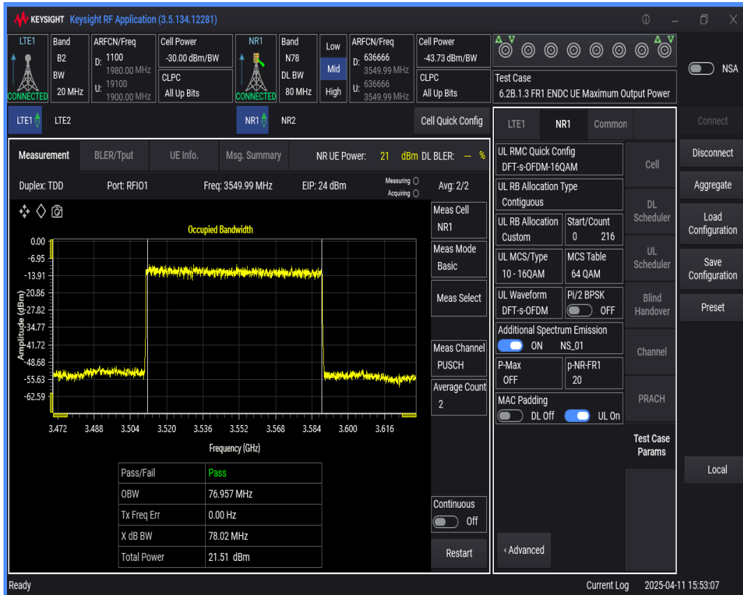
n78 SCS=30kHz DFT_QAM256 BW=40MHz Channel=636666 RB=100@0
