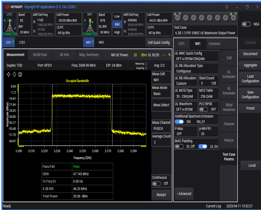
n78 SCS=30kHz DFT_QAM256 BW=15MHz Channel=636666 RB=36@0
