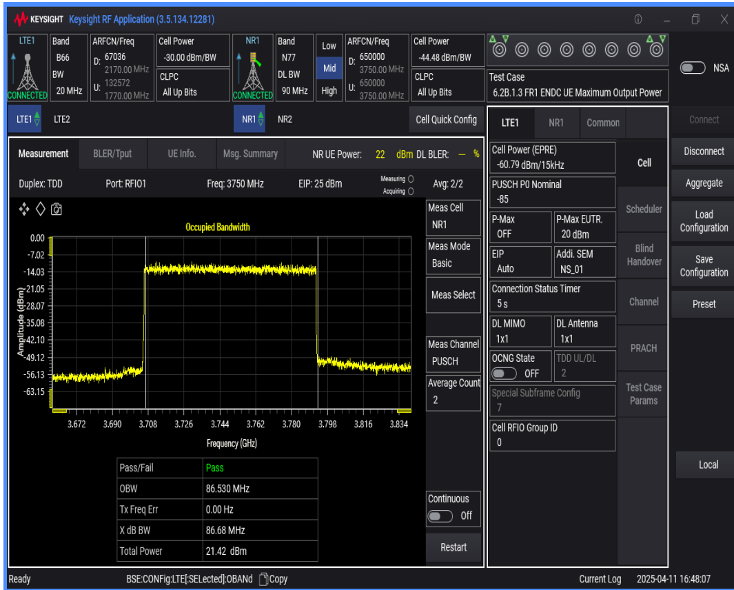
n77 SCS=30kHz DFT_QPSK BW=60MHz Channel=650000 RB=162 @0
