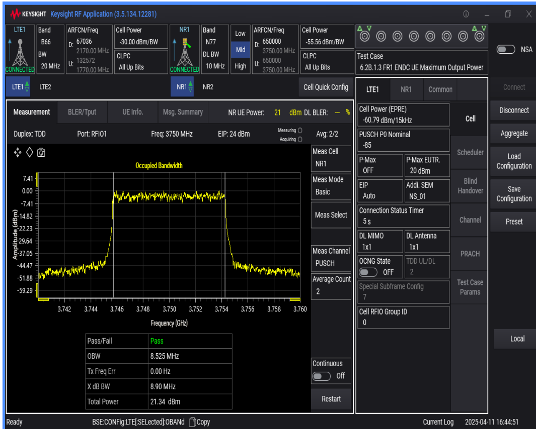
n77 SCS=30kHz DFT_QAM64 BW=90MHz Channel=650000 RB=240 @0
