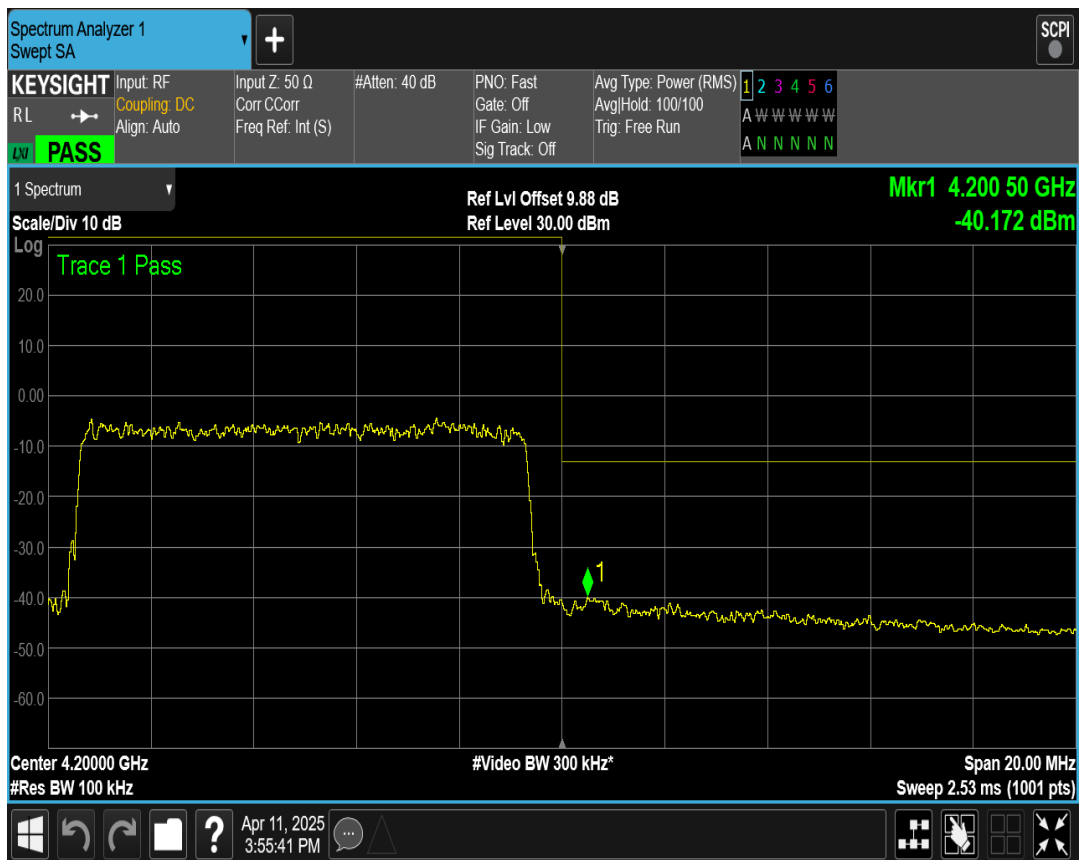
n77 SCS=30kHz CP_QPSK BW=10MHz Channel=679666 RB=1 @23
