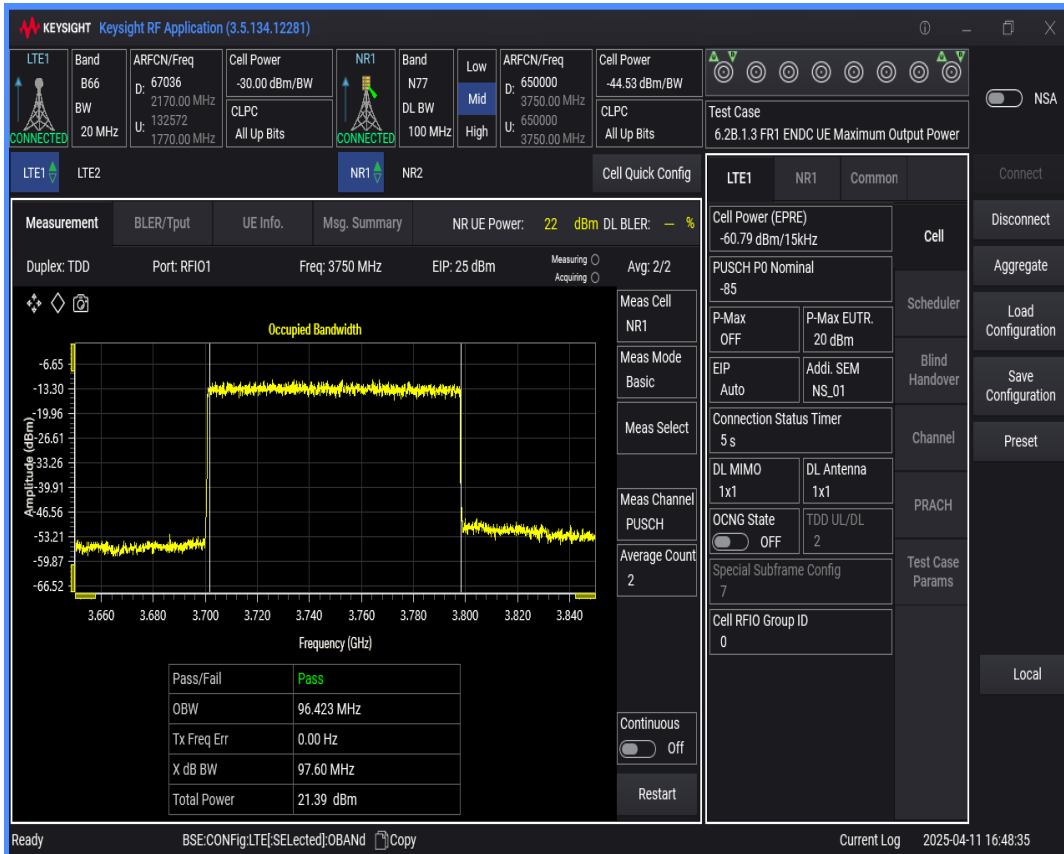
n77 SCS=30kHz DFT_QPSK BW=80MHz Channel=650000 RB=216@0
