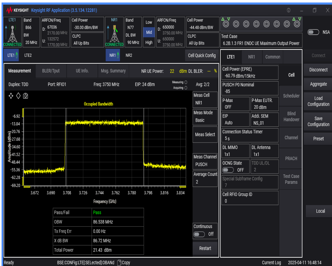
n77 SCS=30kHz DFT_QPSK BW=100MHz Channel=650000 RB=270 @0
