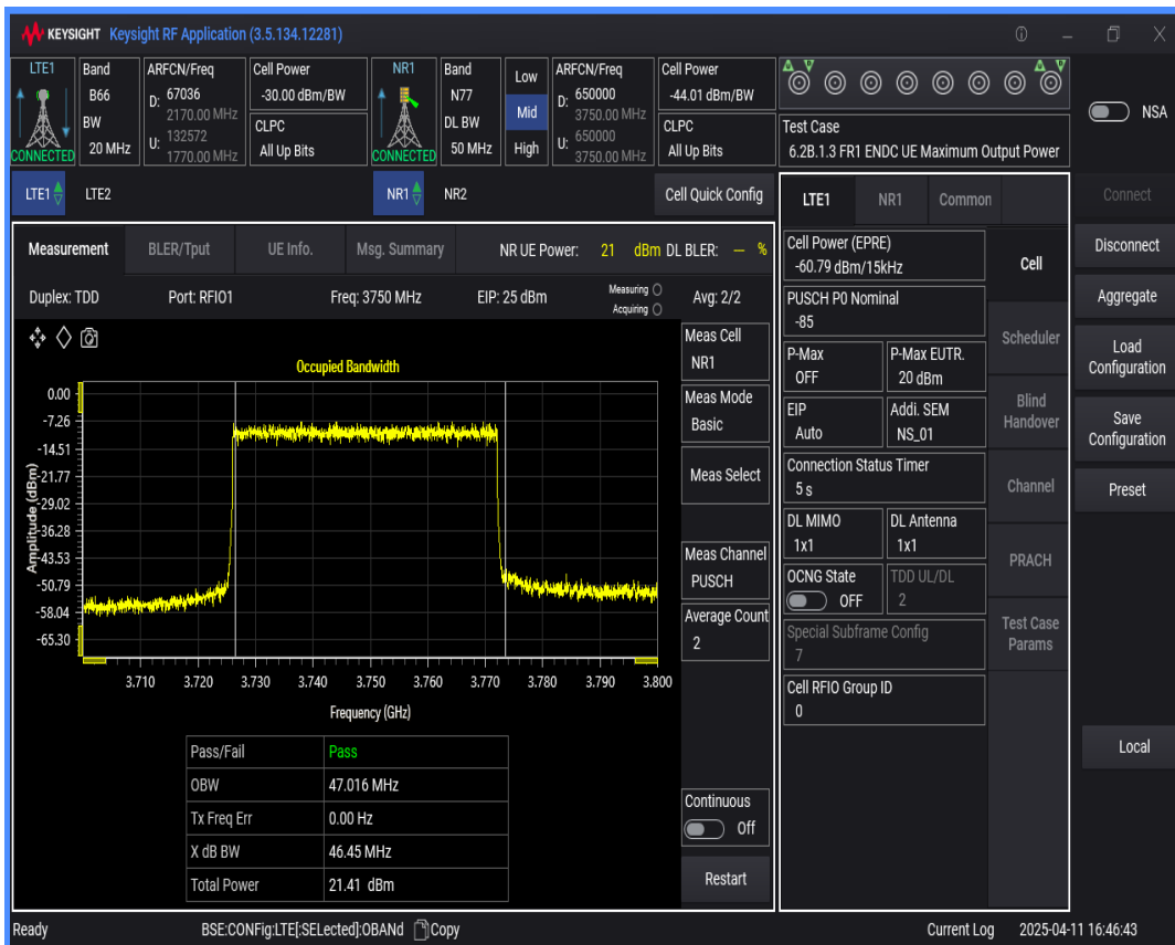
n77 SCS=30kHz DFT_QPSK BW=50MHz Channel=650000 RB=128@0
