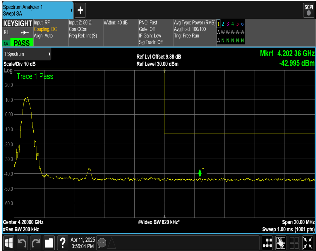
n77 SCS=30kHz CP_QPSK BW=10MHz Channel=620334 RB=24 @0
