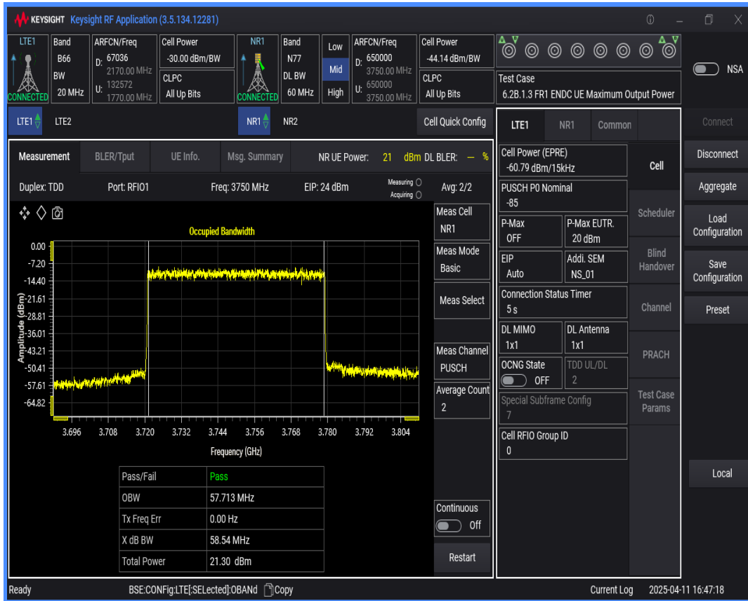
n77 SCS=30kHz DFT_QAM64 BW=80MHz Channel=650000 RB=216 @0
