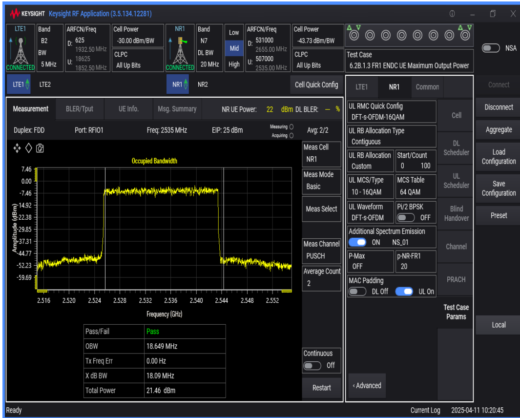
n7 SCS=15kHz DFT_BPSK BW=5MHz Channel=507000 RB=25 @0
