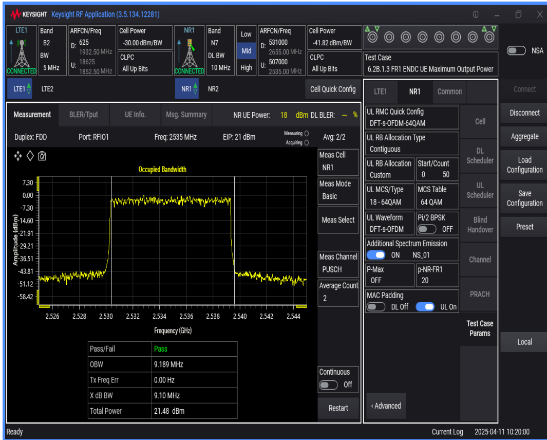
n7 SCS=15kHz DFT_QAM64 BW=5MHz Channel=507000 RB=25 @0
