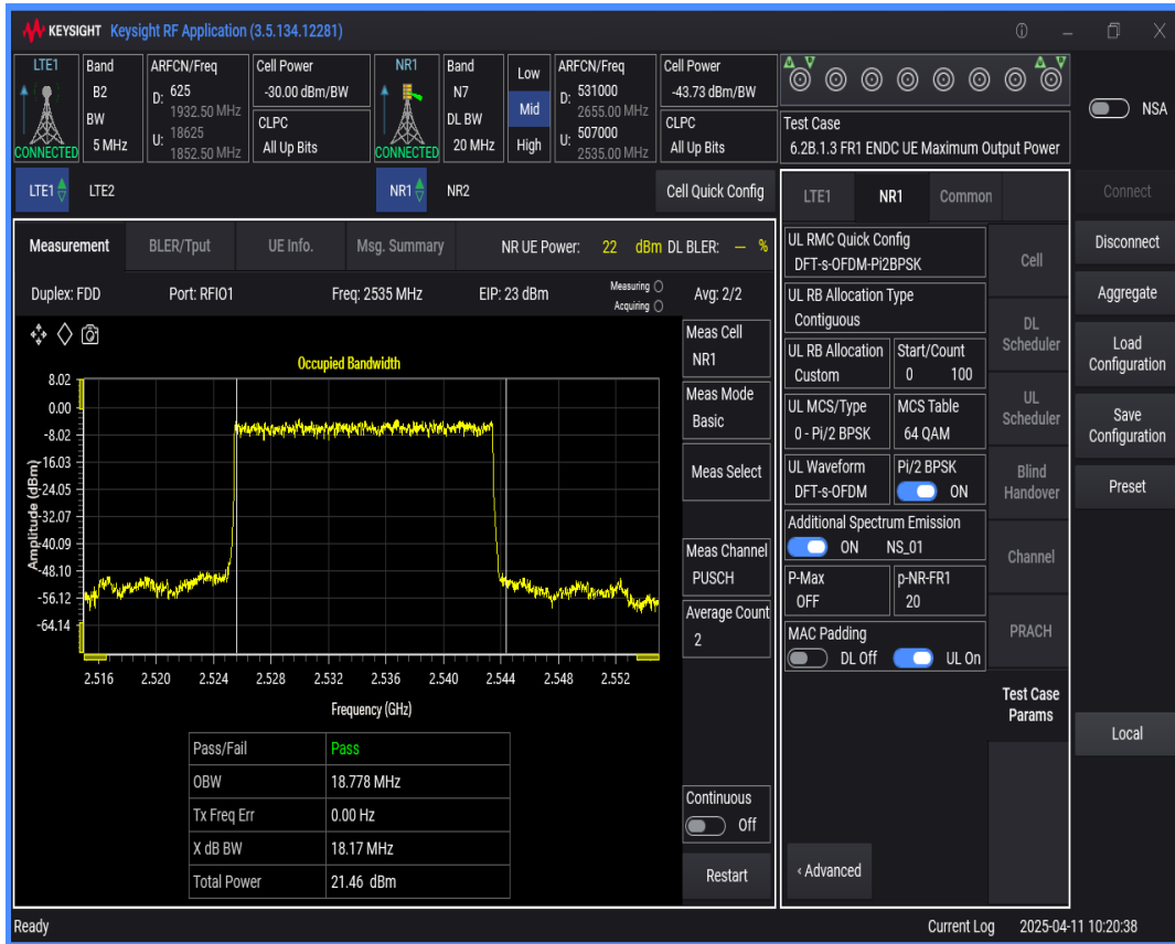
n7 SCS=15kHz DFT_QAM64 BW=15MHz Channel=507000 RB=75@0
