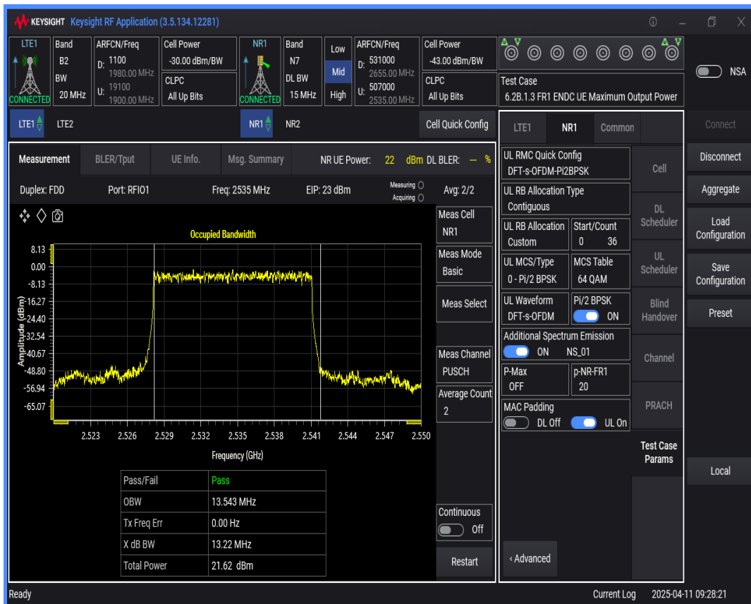
n7 SCS=30kHz DFT_QAM16 BW=10MHz Channel=507000 RB=24 @0
