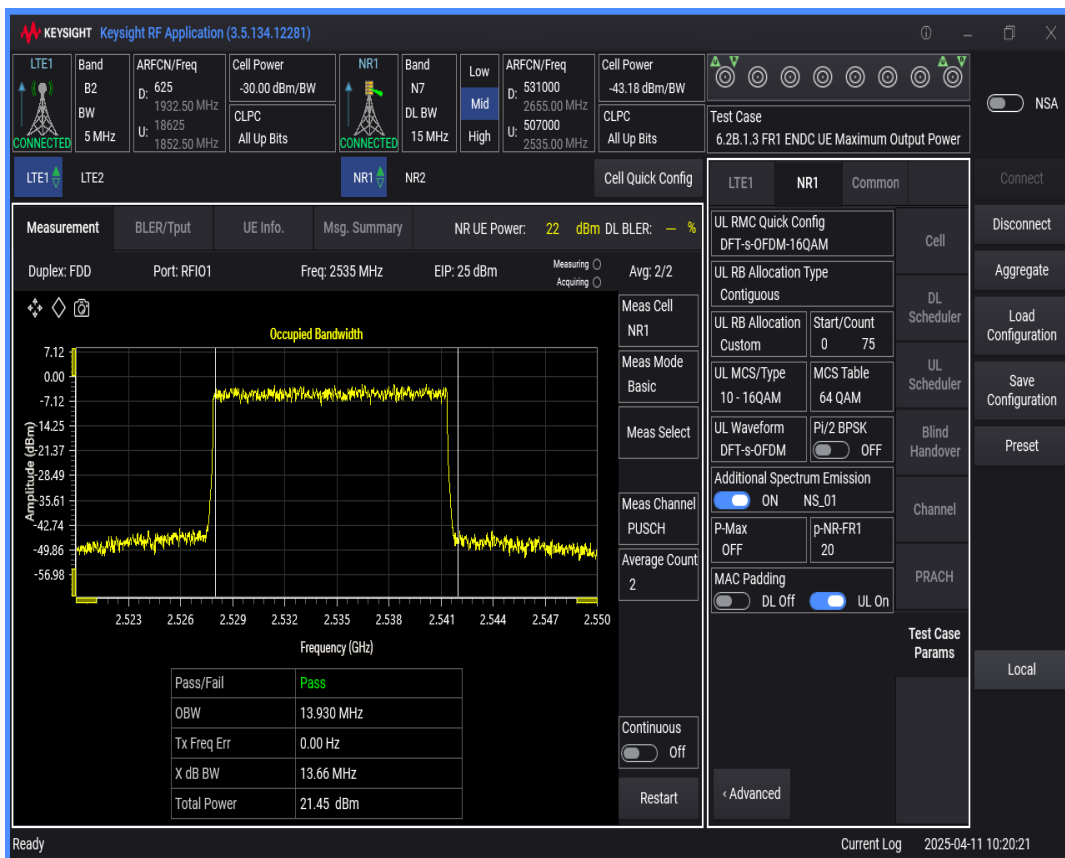
n7 SCS=15kHz DFT_QAM16 BW=20MHz Channel=507000 RB=100@0
