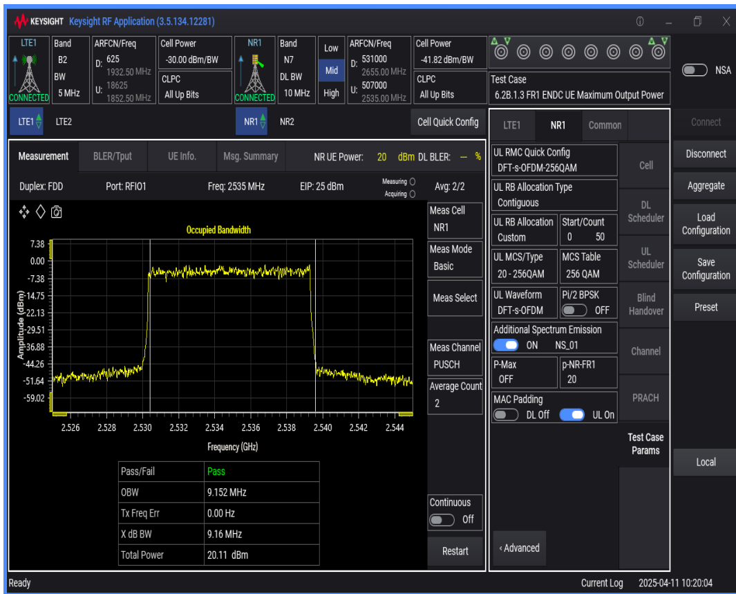
n7 SCS=15kHz DFT_QAM16 BW=5MHz Channel=507000 RB=25 @0
