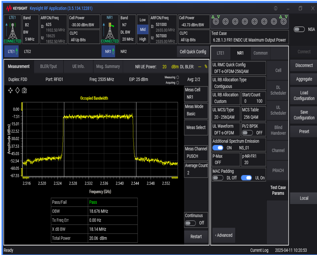
n7 SCS=15kHz DFT_QAM256 BW=15MHz Channel=507000 RB=75@0
