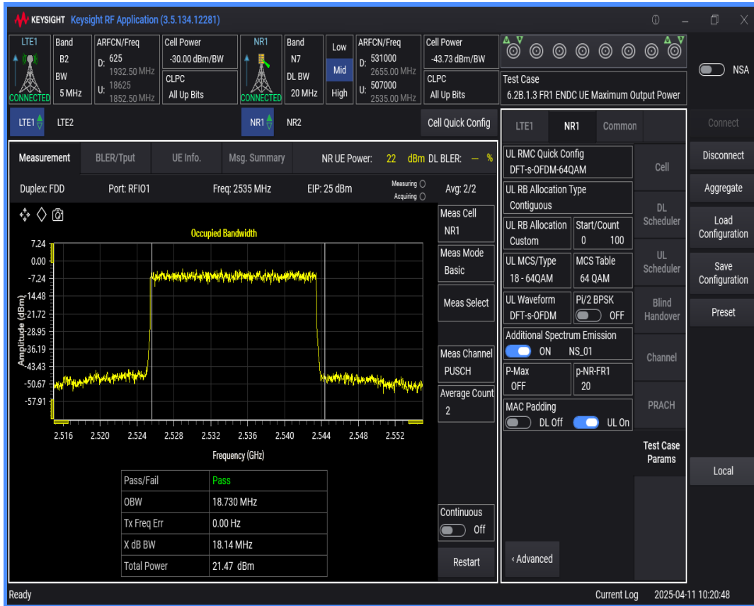
n7 SCS=15kHz DFT_QAM256 BW=5MHz Channel=507000 RB=25@0
