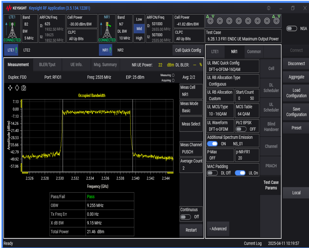
n7 SCS=15kHz DFT_QAM16 BW=15MHz Channel=507000 RB=75@0
