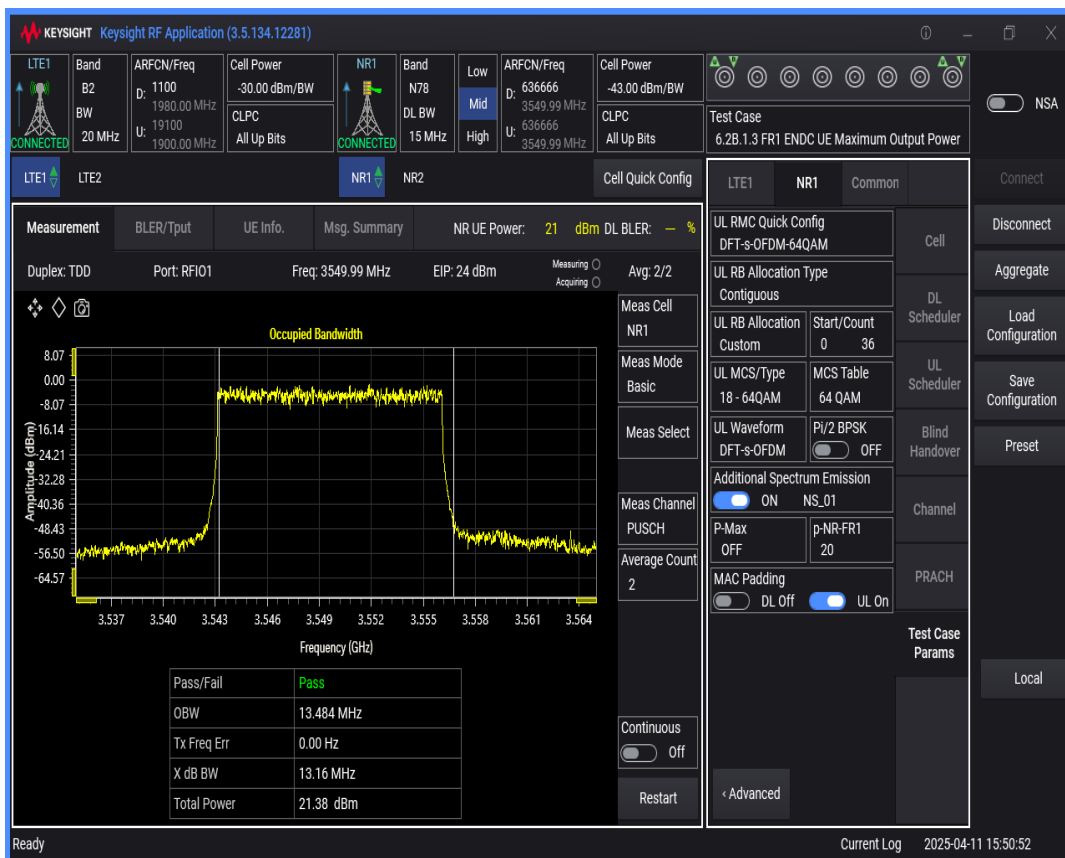
n78 SCS=30kHz DFT_QAM64 BW=40MHz Channel=636666 RB=100@0
