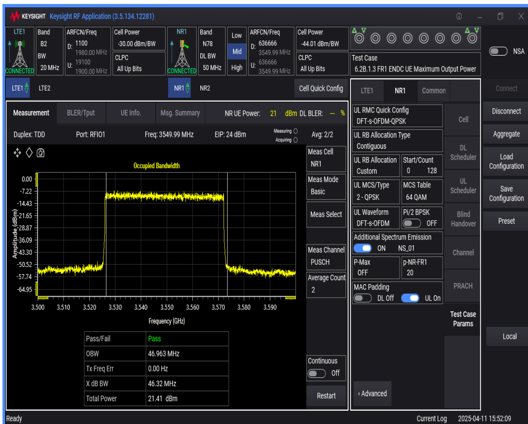
n78 SCS=30kHz DFT_QPSK BW=50MHz Channel=636666 RB=128@0
