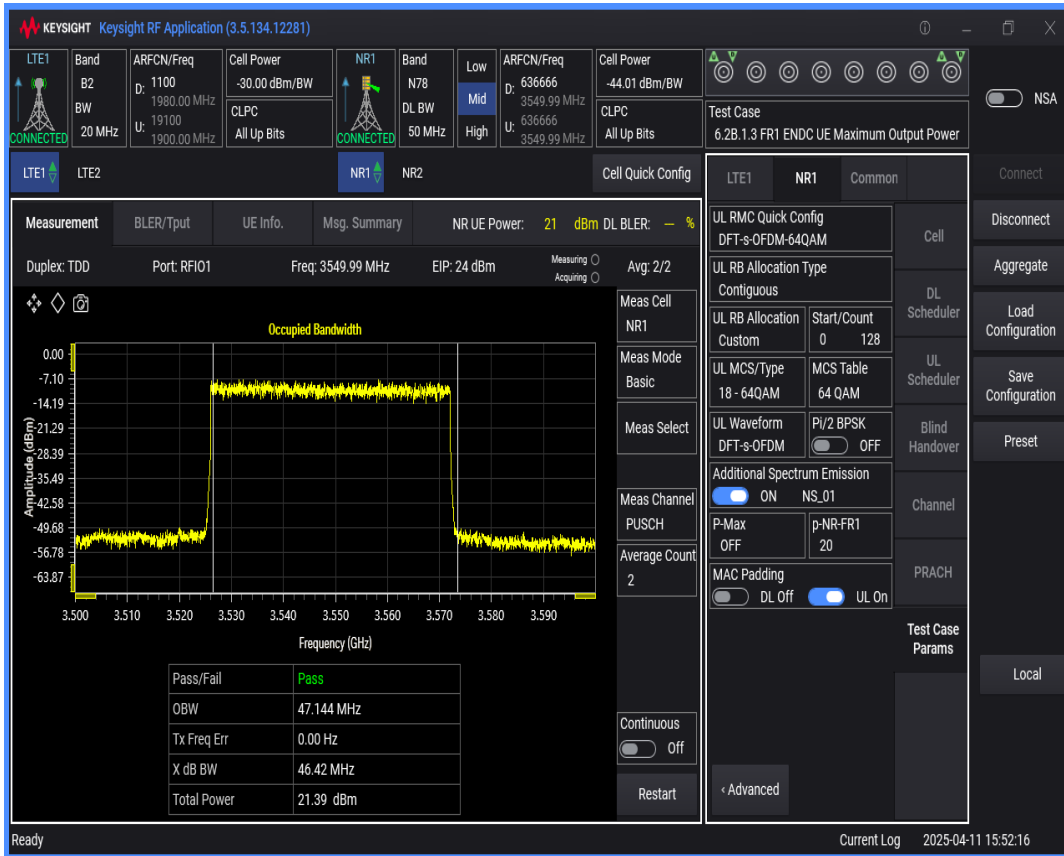
n78 SCS=30kHz DFT_QPSK BW=80MHz Channel=636666 RB=216@0
