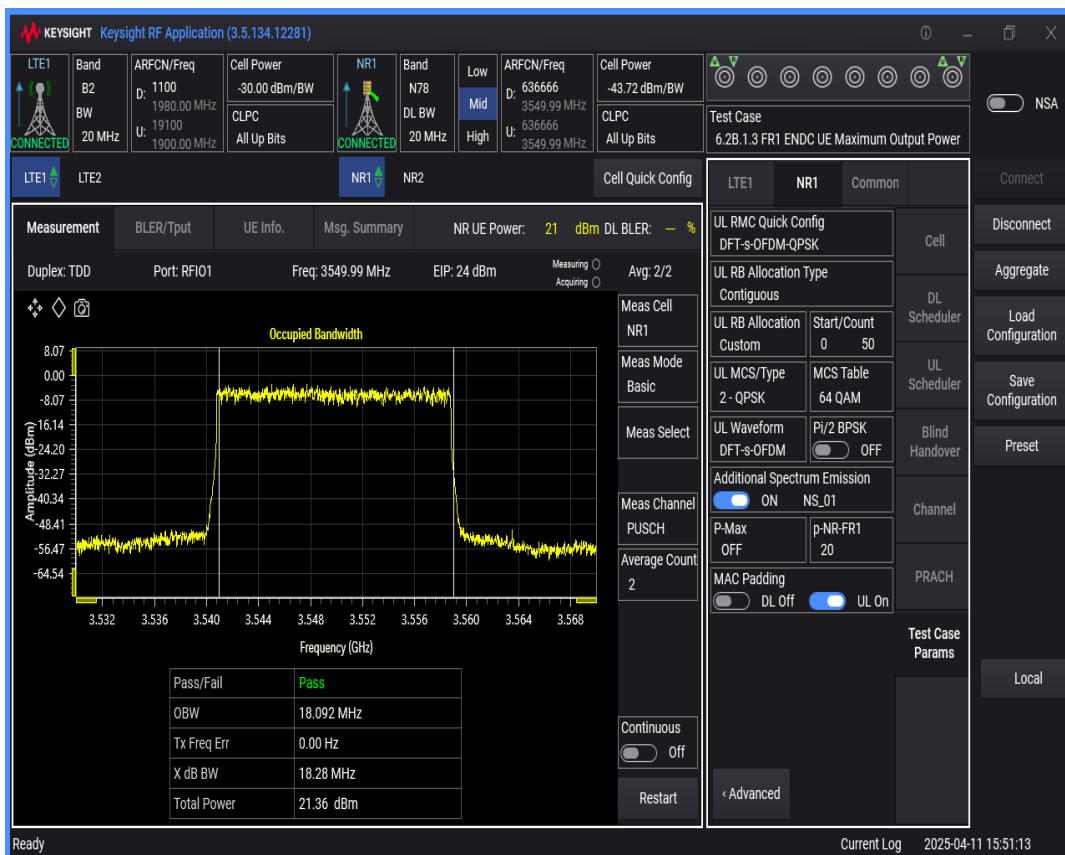
n78 SCS=30kHz DFT_QPSK BW=15MHz Channel=636666 RB=36@0
