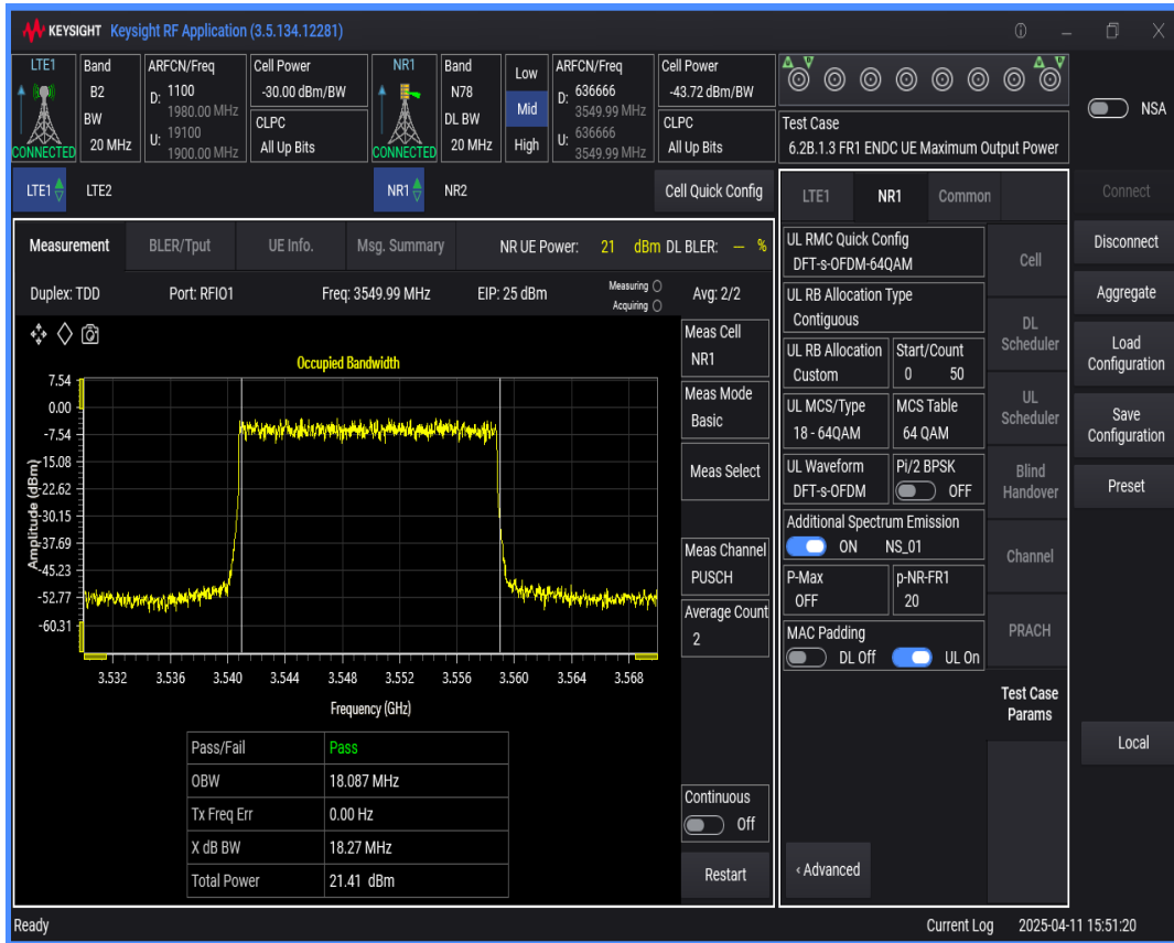
n78 SCS=30kHz DFT_QAM64 BW=15MHz Channel=636666 RB=36@0
