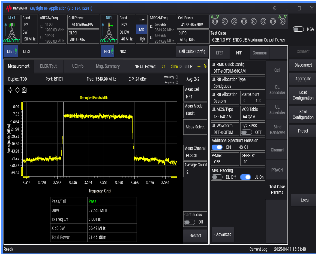
n78 SCS=30kHz DFT_QAM64 BW=60MHz Channel=636666 RB=162 @0
