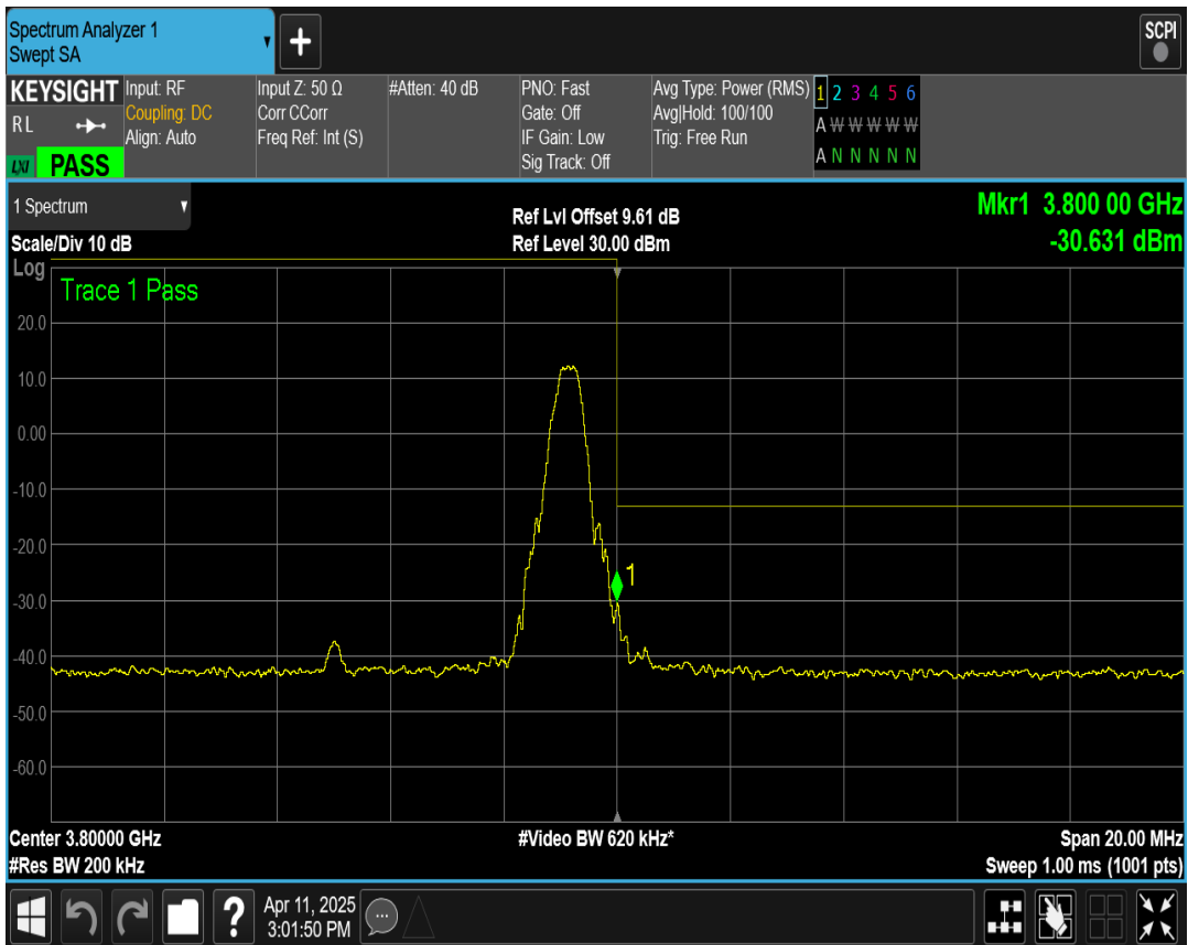
n78 SCS=30kHz CP_QPSK BW=50MHz Channel=621668 RB=133 @0
