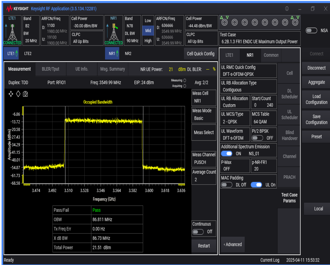
n78 SCS=30kHz DFT_QPSK BW=60MHz Channel=636666 RB=162 @0
