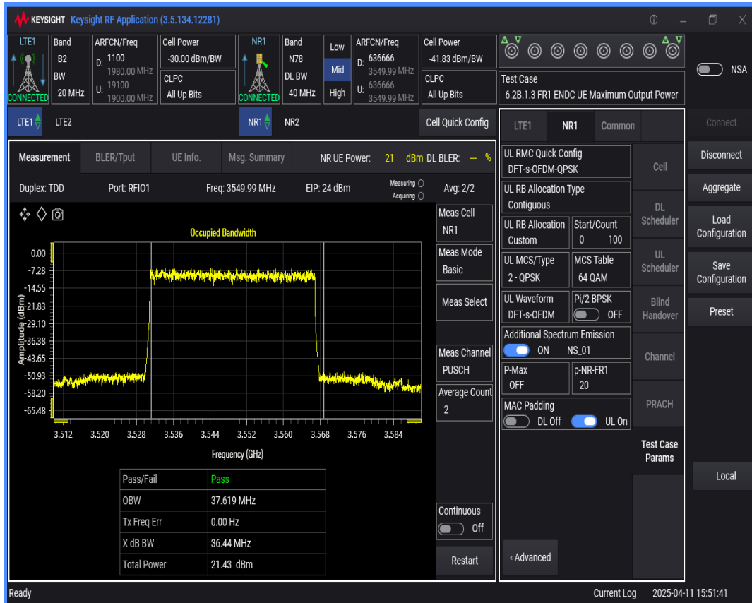
n78 SCS=30kHz DFT_QPSK BW=50MHz Channel=636666 RB=128@0
