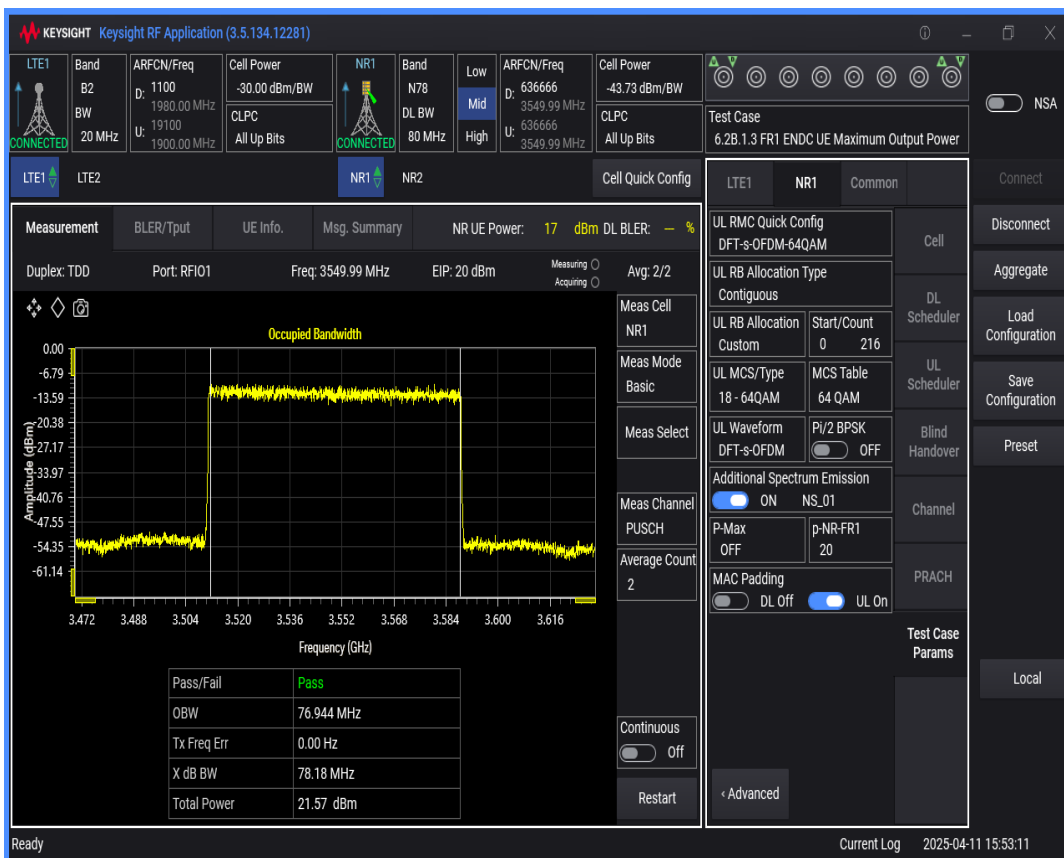
n78 SCS=30kHz DFT_QAM64 BW=20MHz Channel=636666 RB=50 @0
