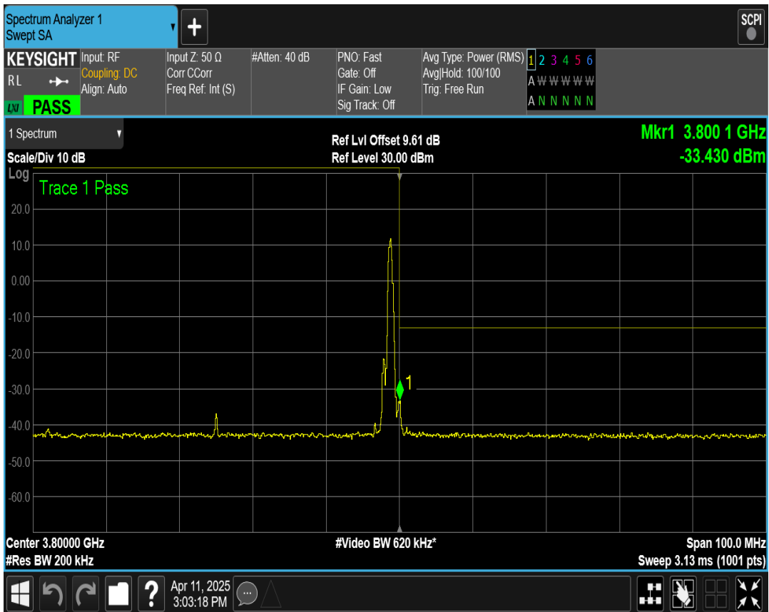
n78 SCS=30kHz CP_QPSK BW=50MHz Channel=651666 RB=133@0
