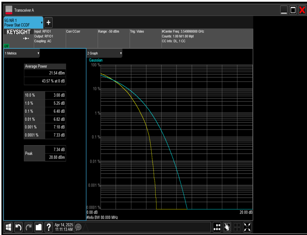
n78 SCS=30kHz DFT_QAM64 BW=80MHz Channel=622668 RB=216@0
