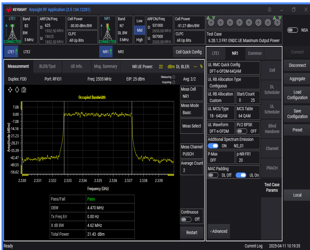
n7 SCS=15kHz DFT_QAM64 BW=20MHz Channel=507000 RB=100 @0
