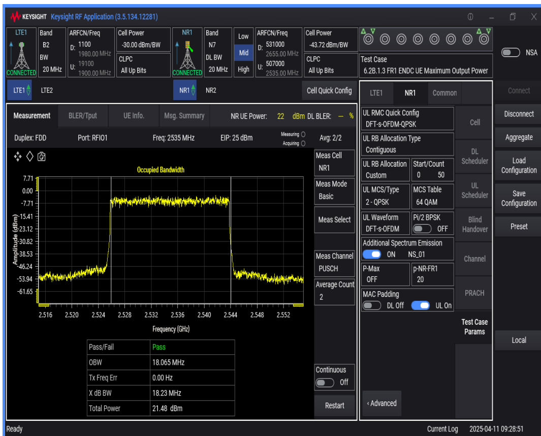
n7 SCS=30kHz DFT_QPSK BW=15MHz Channel=507000 RB=36 @0
