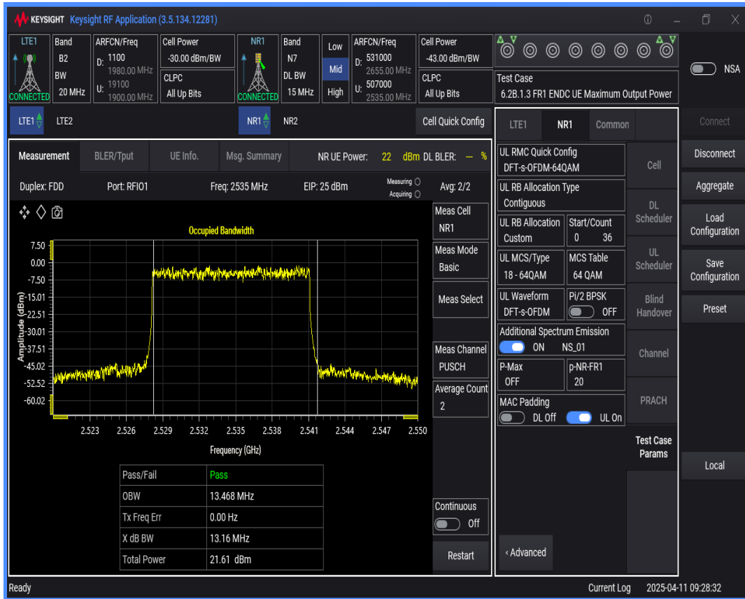
n7 SCS=30kHz DFT_QAM64 BW=10MHz Channel=507000 RB=24@0
