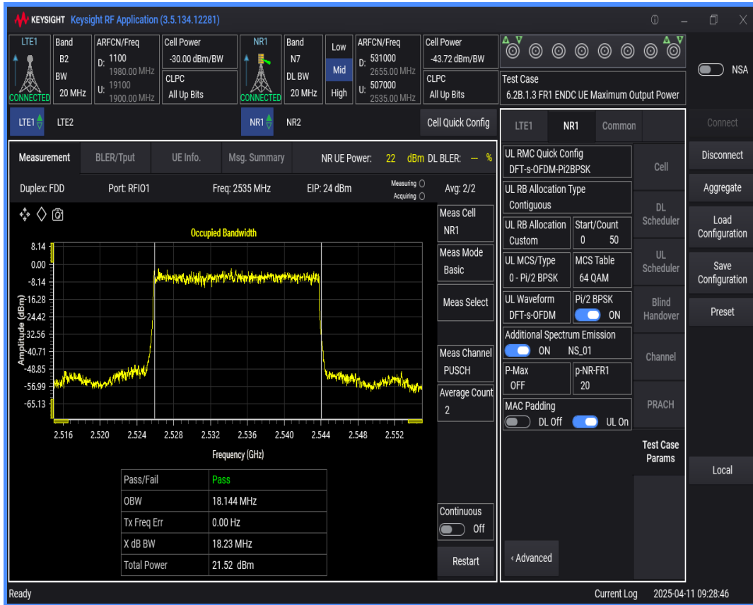
n7 SCS=15kHz DFT_QAM64 BW=5MHz Channel=507000 RB=25 @0
