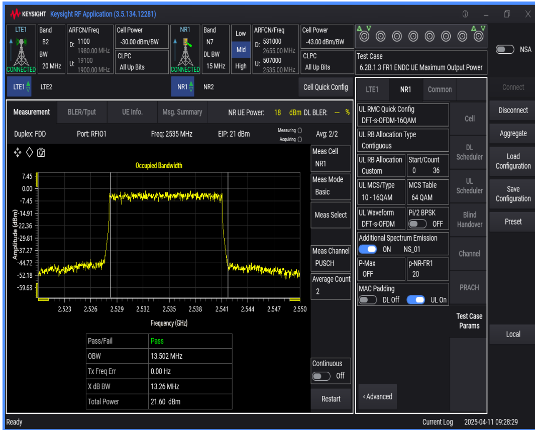
n7 SCS=30kHz DFT_QAM256 BW=15MHz Channel=507000 RB=36@0
