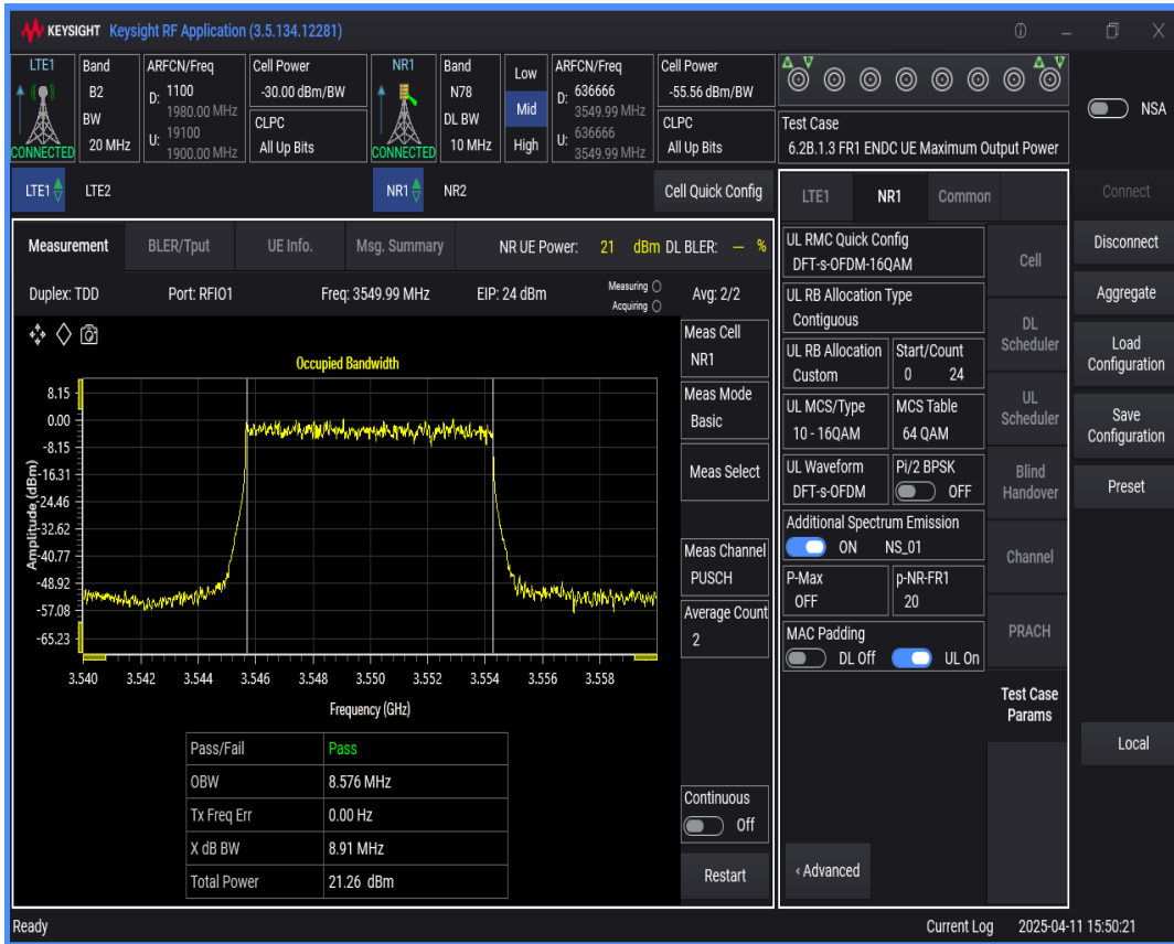
n78 SCS=30kHz DFT_QAM16 BW=15MHz Channel=636666 RB=36@0
