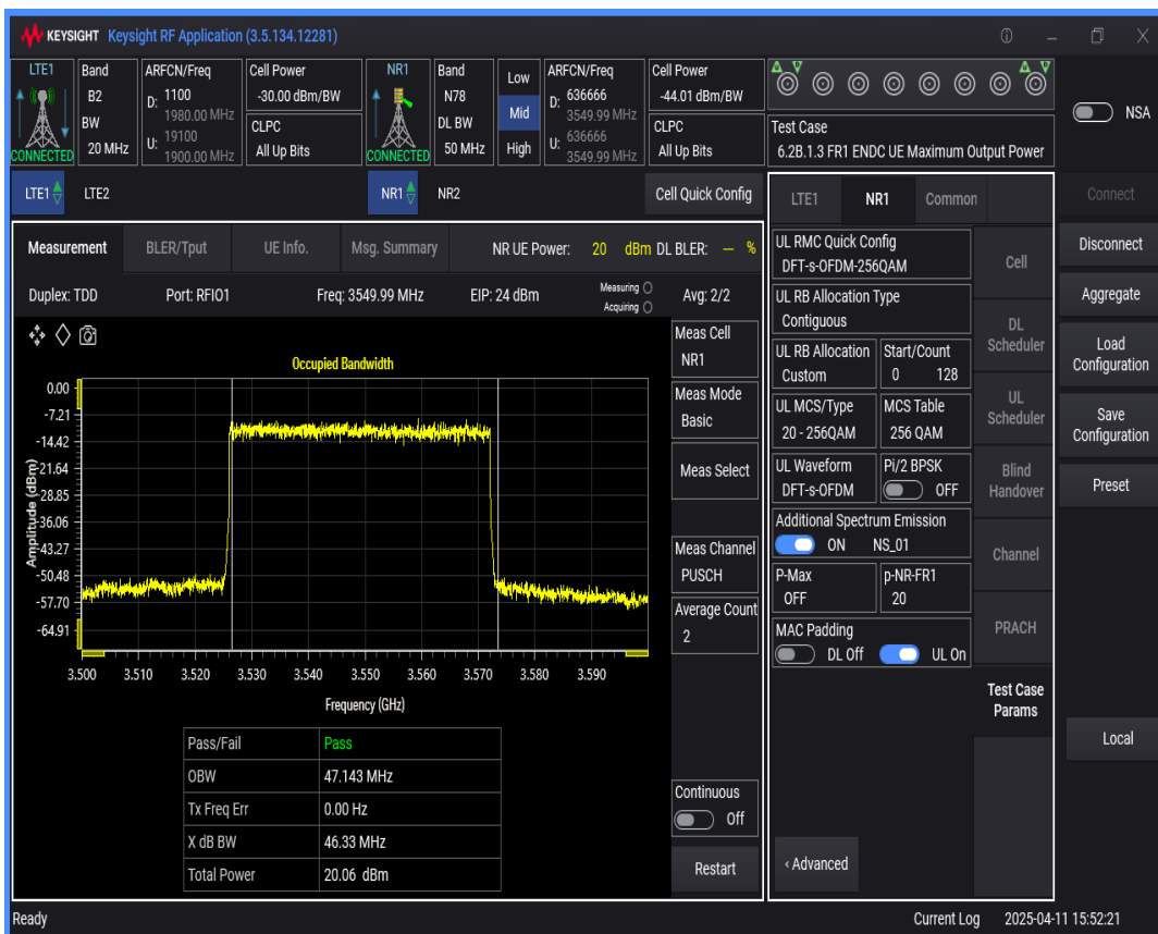
n78 SCS=30kHz DFT_QAM256 BW=60MHz Channel=636666 RB=162 @0
