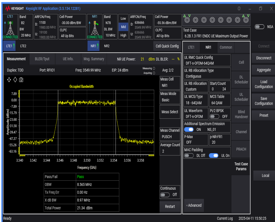
n78 SCS=30kHz DFT_QAM64 BW=15MHz Channel=636666 RB=36@0
