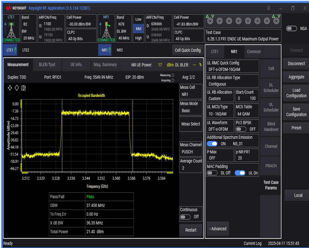
n78 SCS=30kHz DFT_QAM16 BW=80MHz Channel=636666 RB=216 @0
