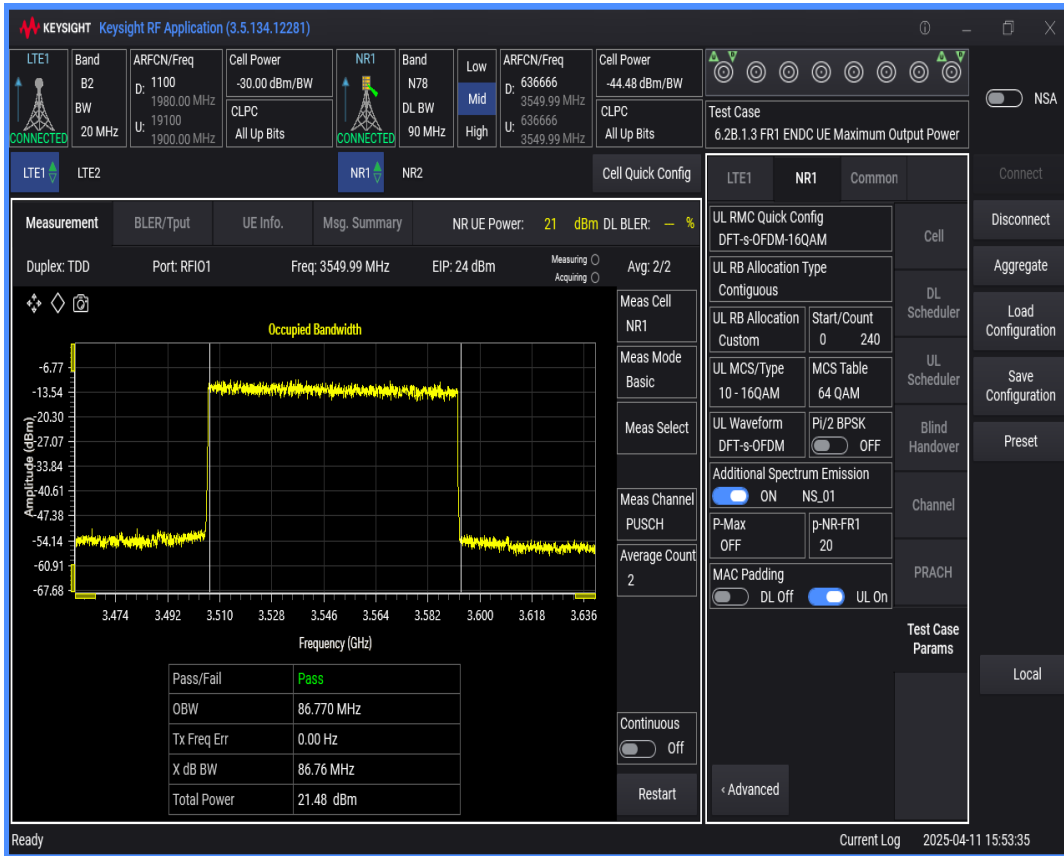
n78 SCS=30kHz DFT_QAM16 BW=50MHz Channel=636666 RB=128 @0
