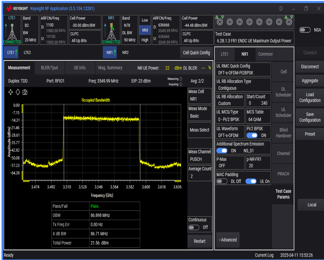
n78 SCS=30kHz DFT_QAM16 BW=100MHz Channel=636666 RB=270@0
