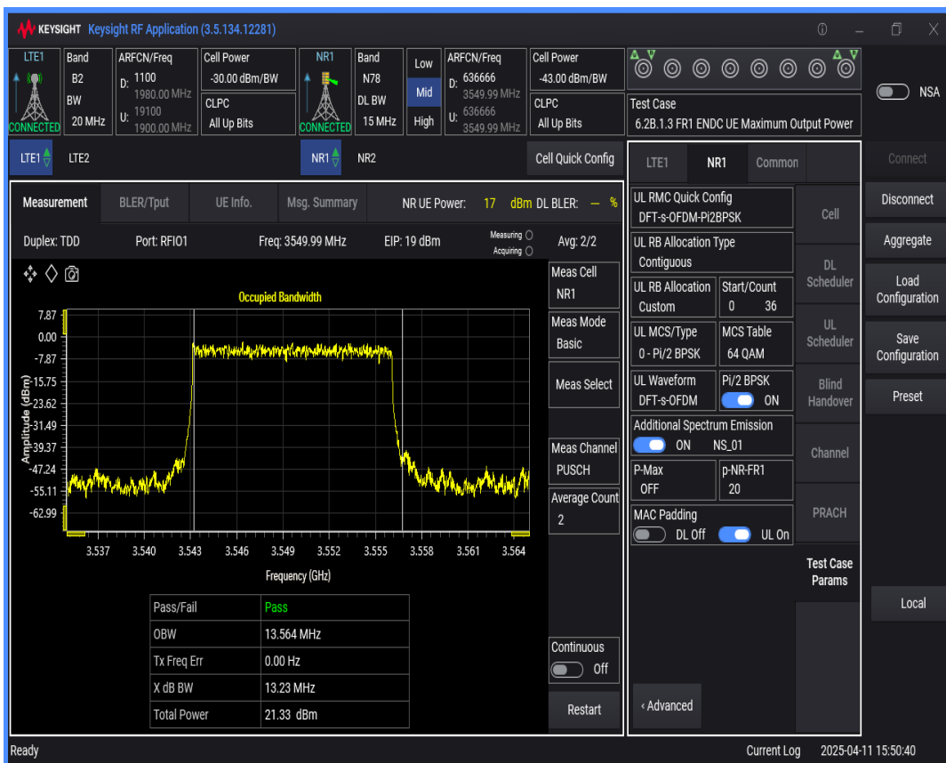
n78 SCS=30kHz DFT_QAM16 BW=10MHz Channel=636666 RB=24@0
