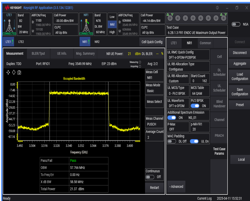
n78 SCS=30kHz DFT_BPSK BW=20MHz Channel=636666 RB=50 @0
