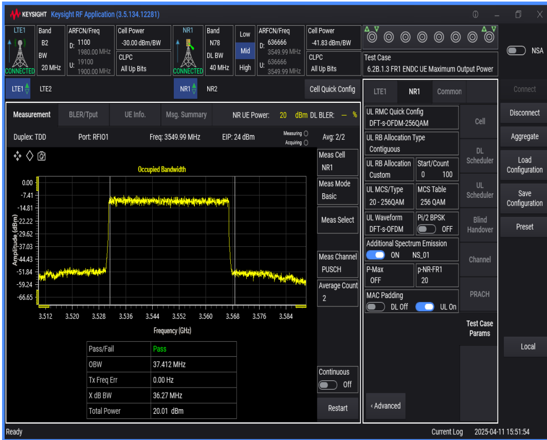
n78 SCS=30kHz DFT_QAM256 BW=50MHz Channel=636666 RB=128 @0
