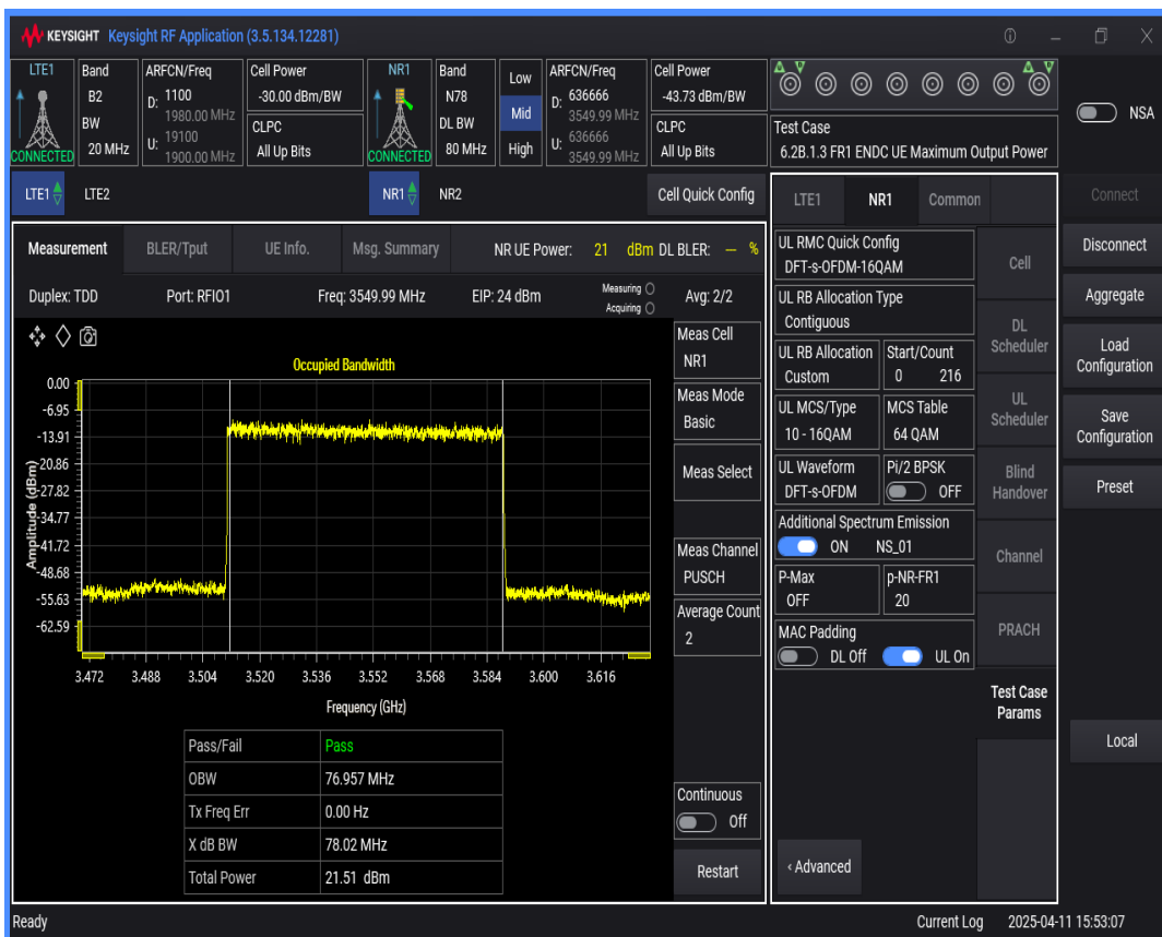
n78 SCS=30kHz DFT_QAM16 BW=60MHz Channel=636666 RB=162 @0
