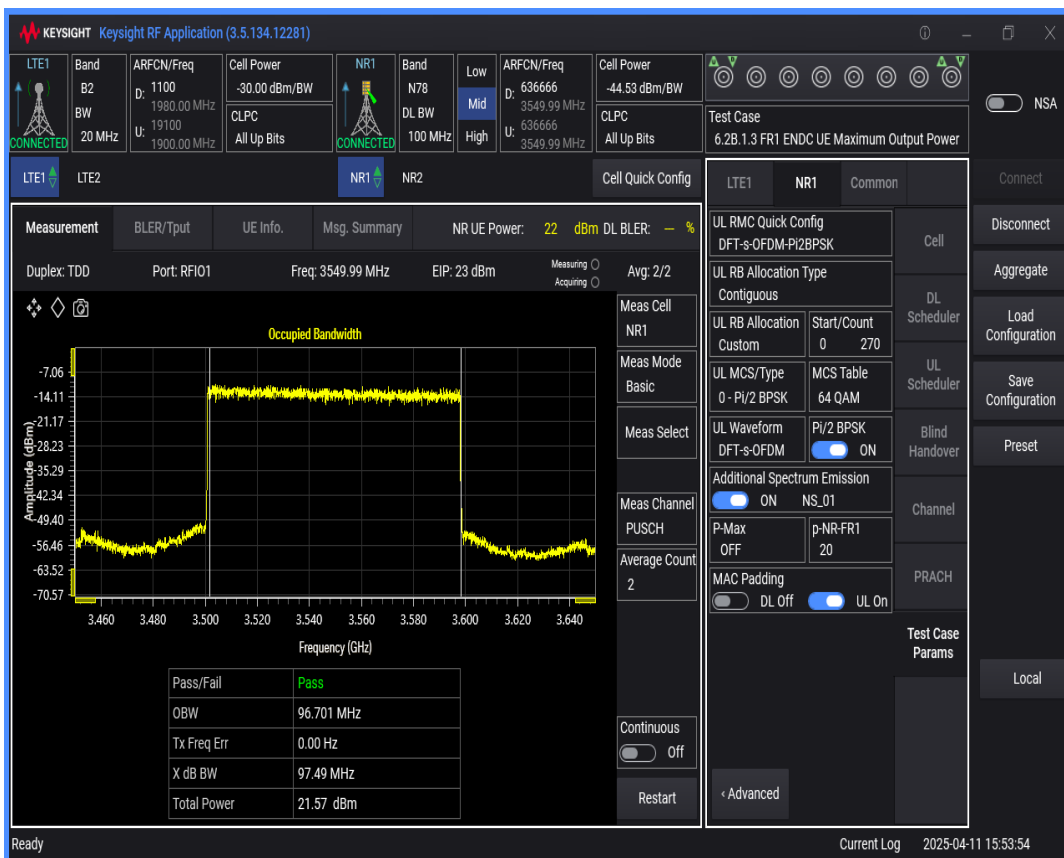
n78 SCS=30kHz DFT_BPSK BW=10MHz Channel=636666 RB=24 @0
