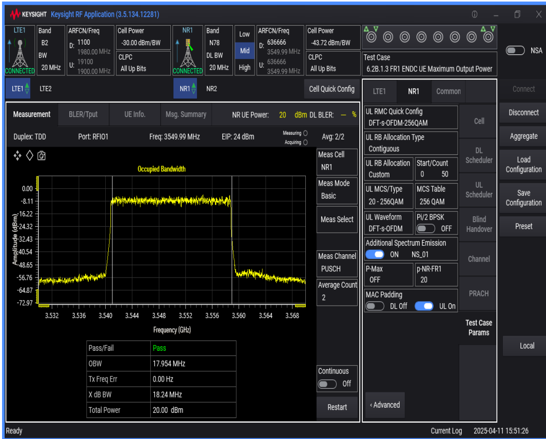
n78 SCS=30kHz DFT_QAM256 BW=15MHz Channel=636666 RB=36@0
