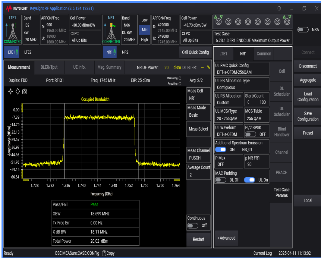
n66 SCS=15kHz DFT_QAM256 BW=5MHz Channel=349000 RB=25@0
