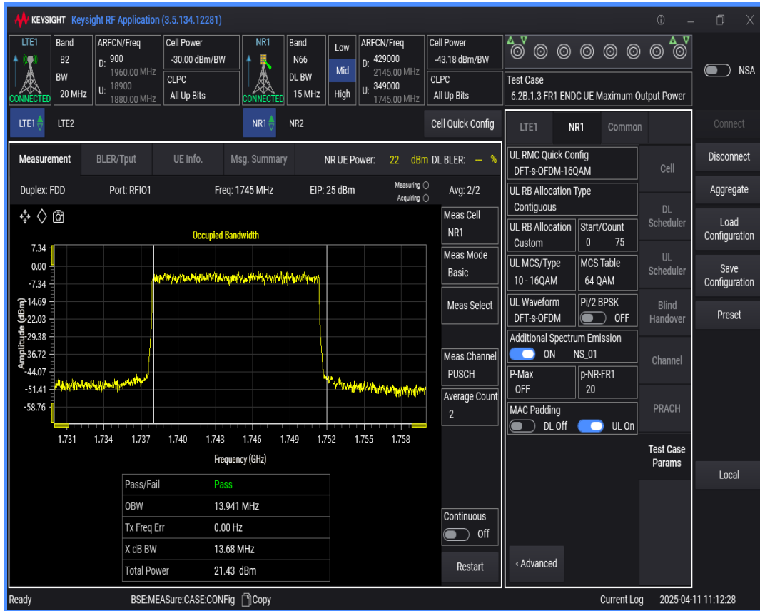
n66 SCS=15kHz DFT_BPSK BW=40MHz Channel=349000 RB=216@0
