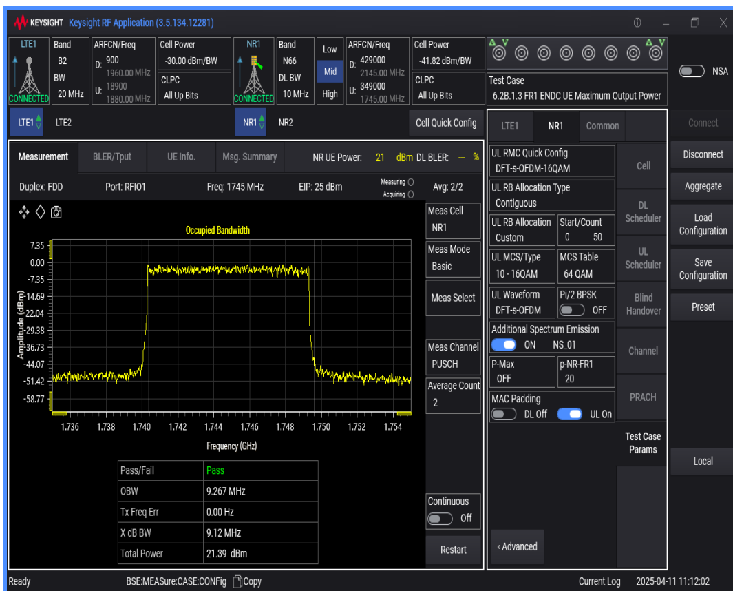
n66 SCS=15kHz DFT_QAM16 BW=15MHz Channel=349000 RB=75@0
