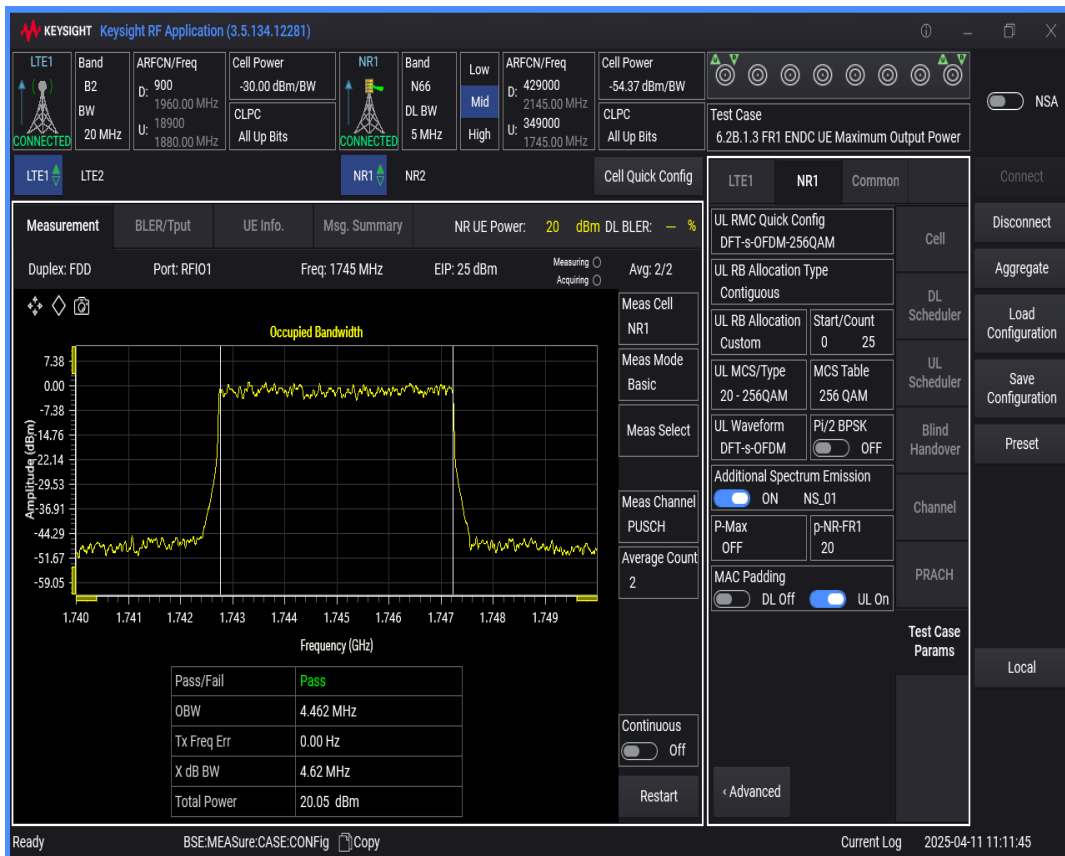
n66 SCS=15kHz DFT_QAM64 BW=15MHz Channel=349000 RB=75@0
