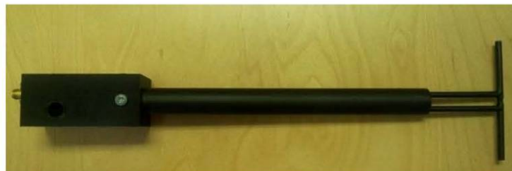
Figure 1 – MVG COMOSAR Validation Dipole
