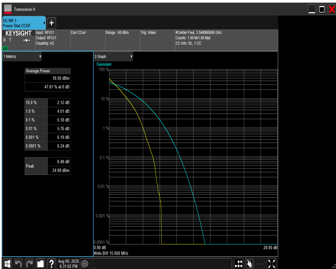
n78 SCS=30kHz DFT_BPSK BW=15MHz Channel=620500 RB=36@0
