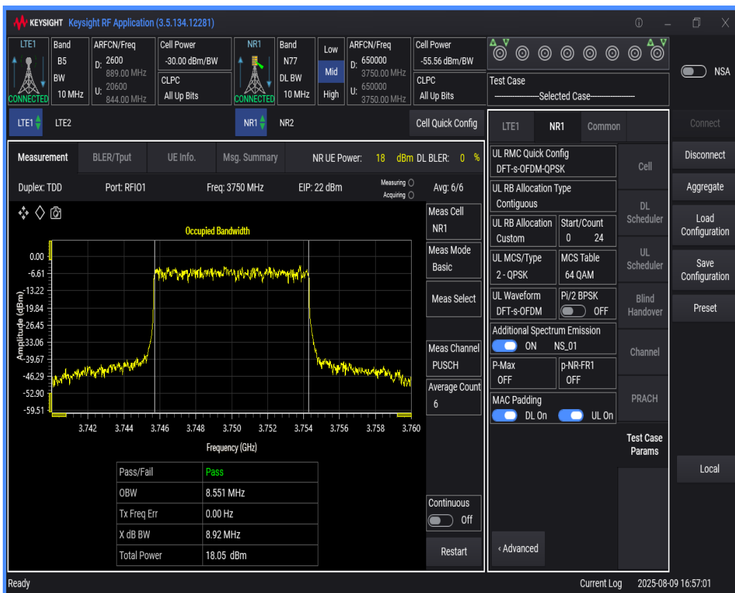
n77 SCS=30kHz DFT_QPSK BW=100MHz Channel=650000 RB=270@0
