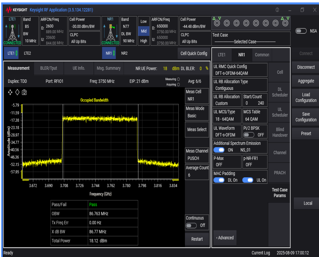
n77 SCS=30kHz DFT_QAM64 BW=80MHz Channel=650000 RB=216@0
