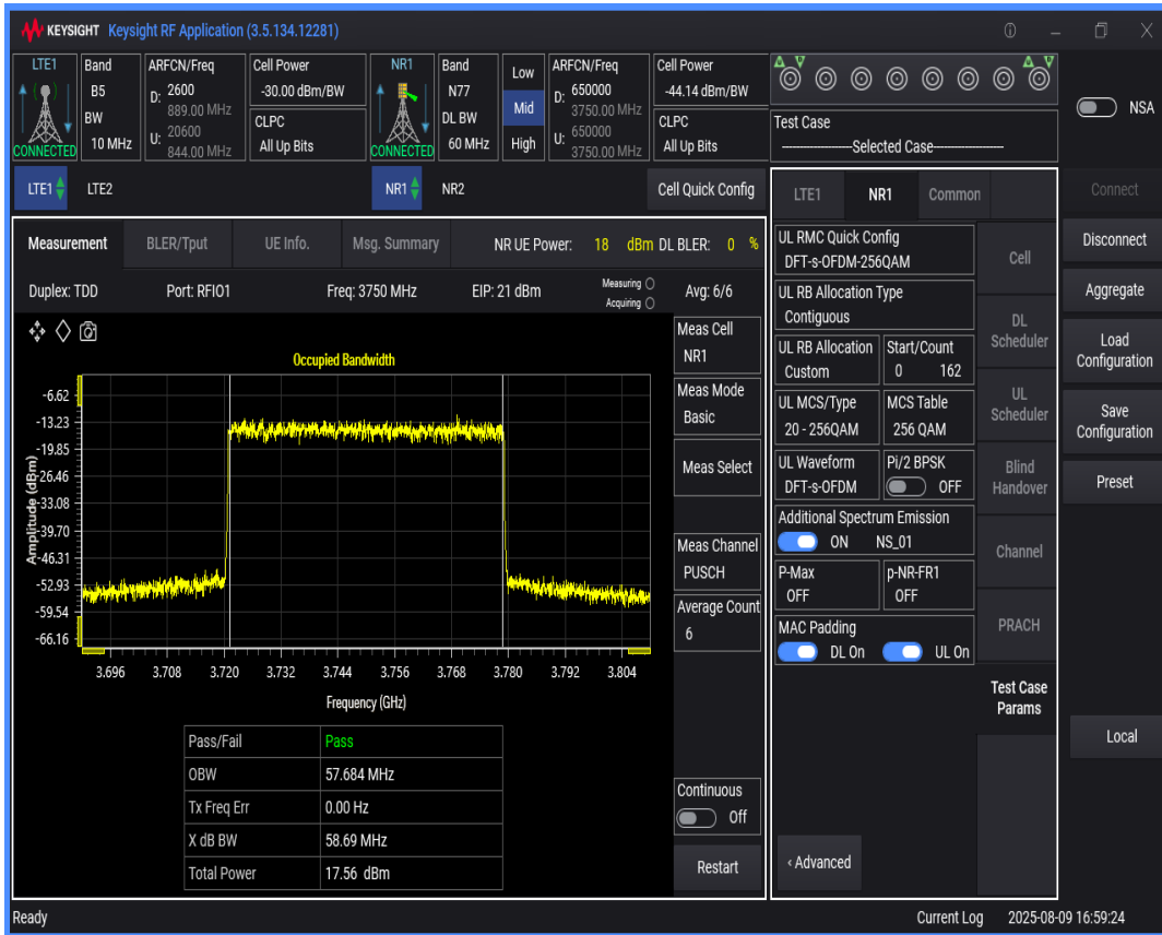
n77 SCS=30kHz DFT_QAM64 BW=90MHz Channel=650000 RB=240@0
