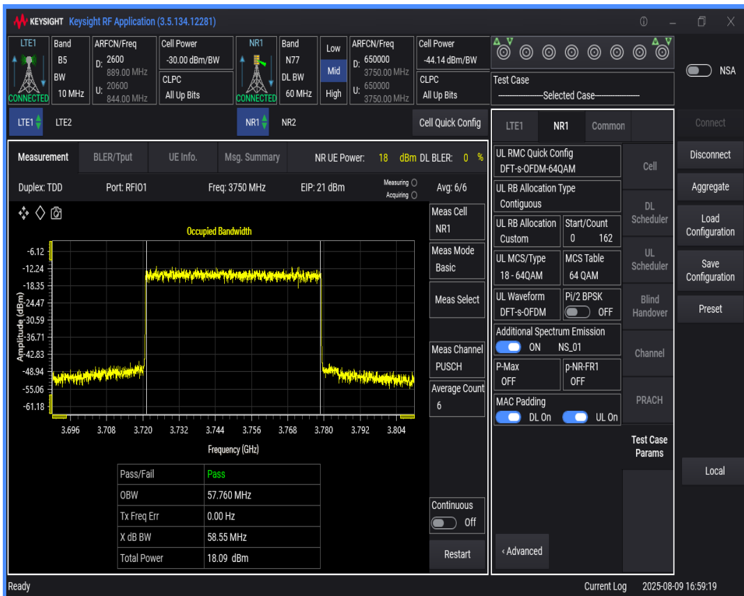
n77 SCS=30kHz DFT_QAM64 BW=50MHz Channel=650000 RB=128 @0
