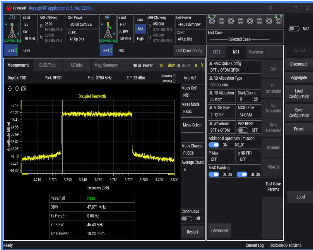
n77 SCS=30kHz DFT_QPSK BW=15MHz Channel=650000 RB=36@0
