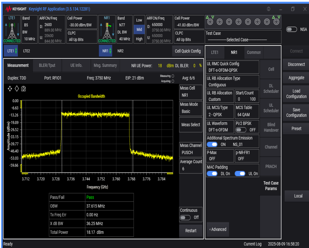
n77 SCS=30kHz DFT_QPSK BW=40MHz Channel=650000 RB=100@0
