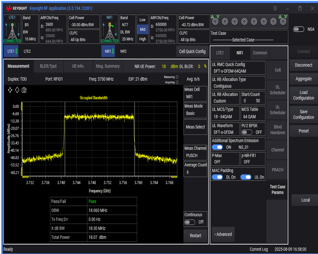
n77 SCS=30kHz DFT_QAM64 BW=60MHz Channel=650000 RB=162 @0
