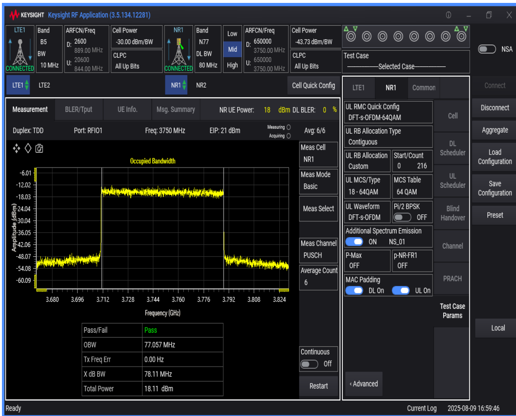
n77 SCS=30kHz DFT_QPSK BW=10MHz Channel=650000 RB=24@0
