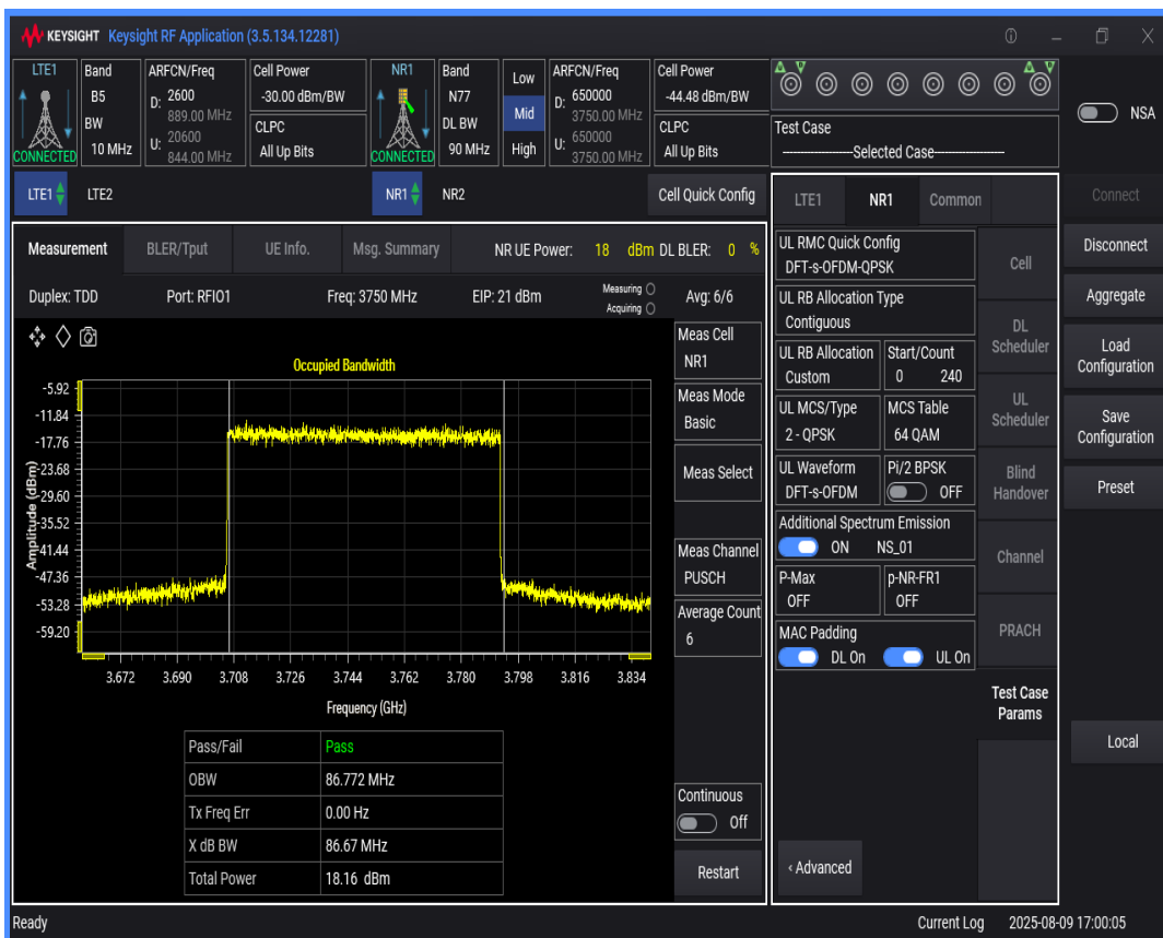
n77 SCS=30kHz DFT_QPSK BW=50MHz Channel=650000 RB=128@0
