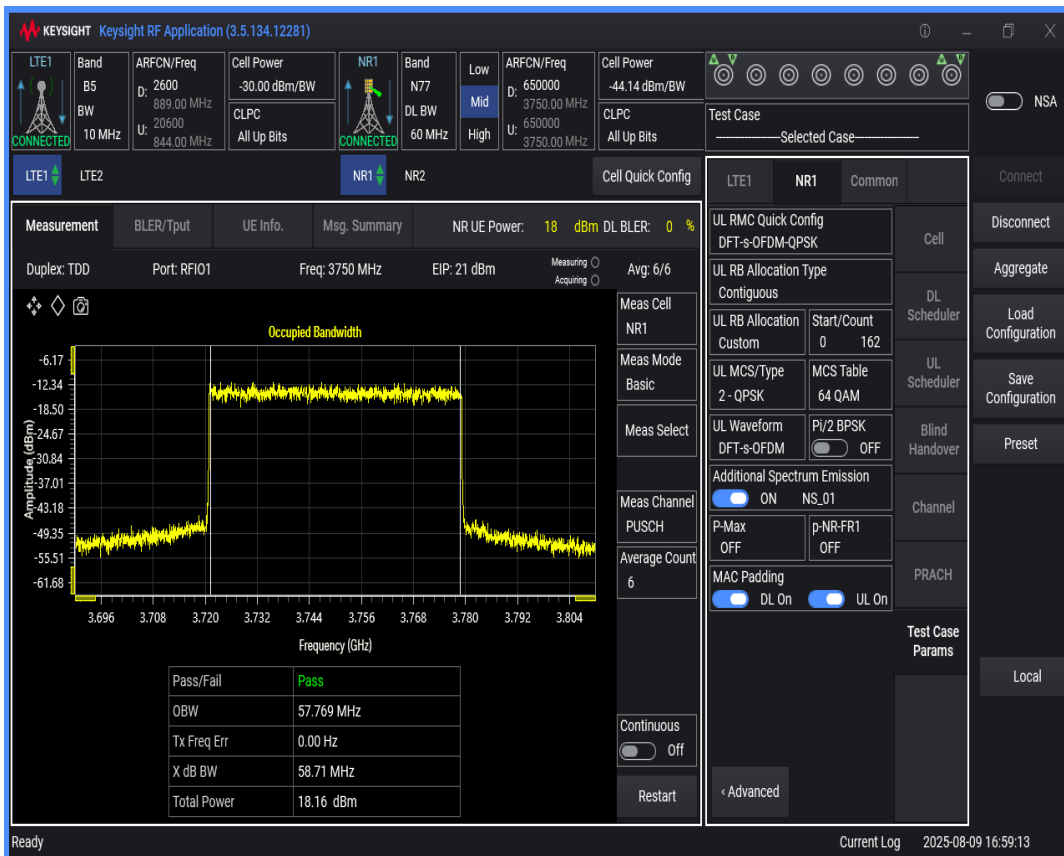
n77 SCS=30kHz DFT_QPSK BW=80MHz Channel=650000 RB=216@0
