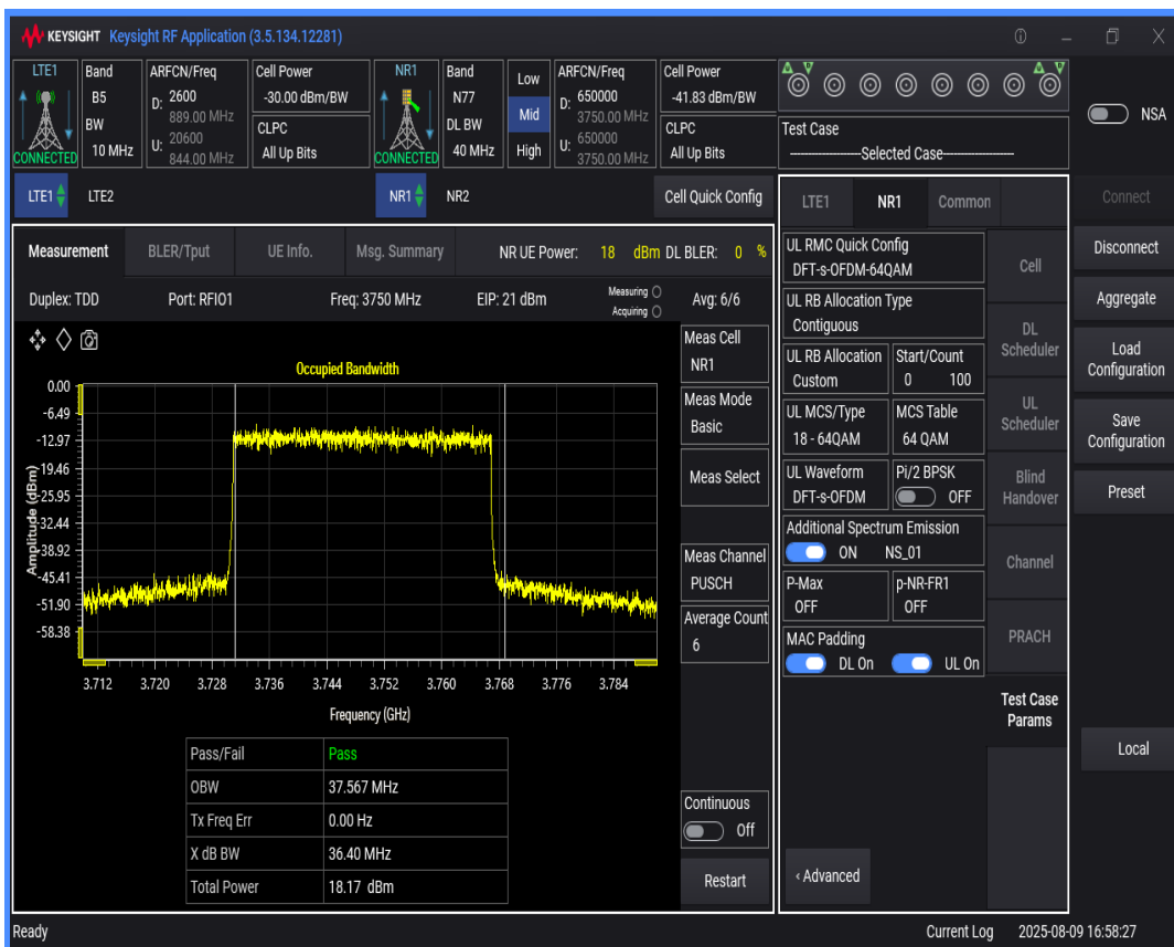
n77 SCS=30kHz DFT_QAM64 BW=20MHz Channel=650000 RB=50@0
