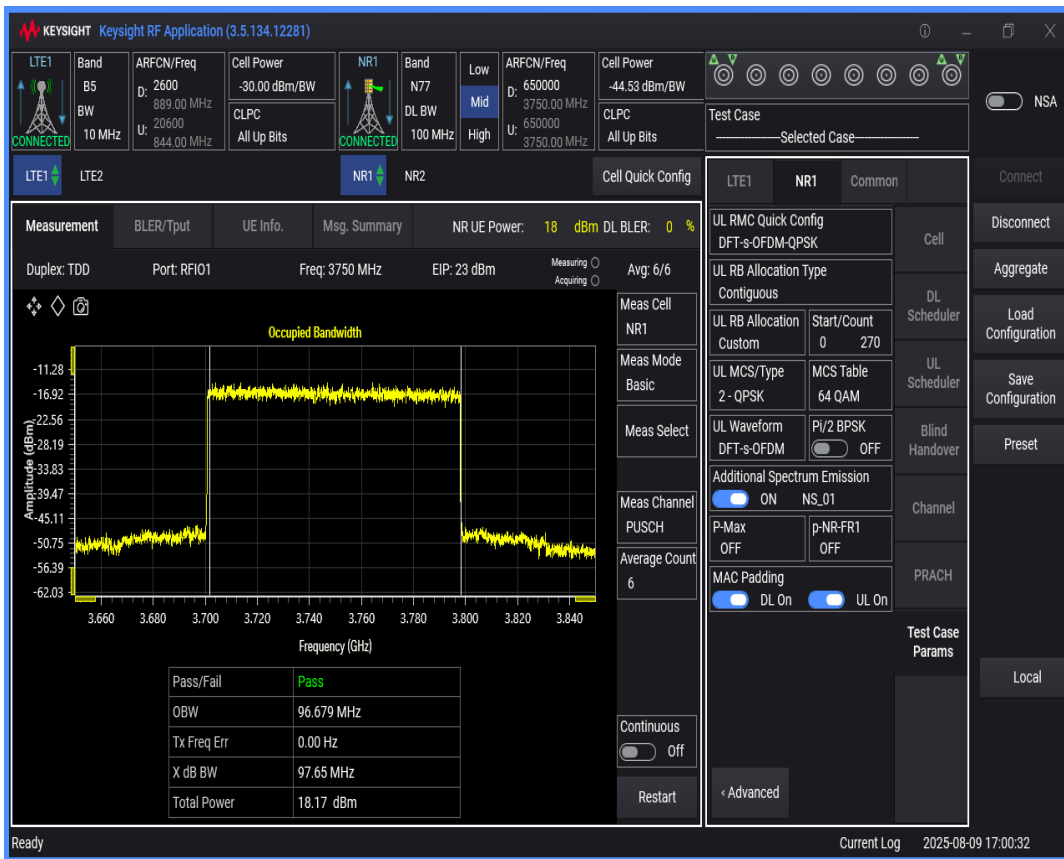
n77 SCS=30kHz DFT_QAM64 BW=40MHz Channel=650000 RB=100@0
