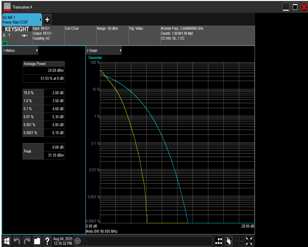
n77(3450-3550) SCS=30kHz DFT_BPSK BW=90MHz Channel=633334 RB=240@0
