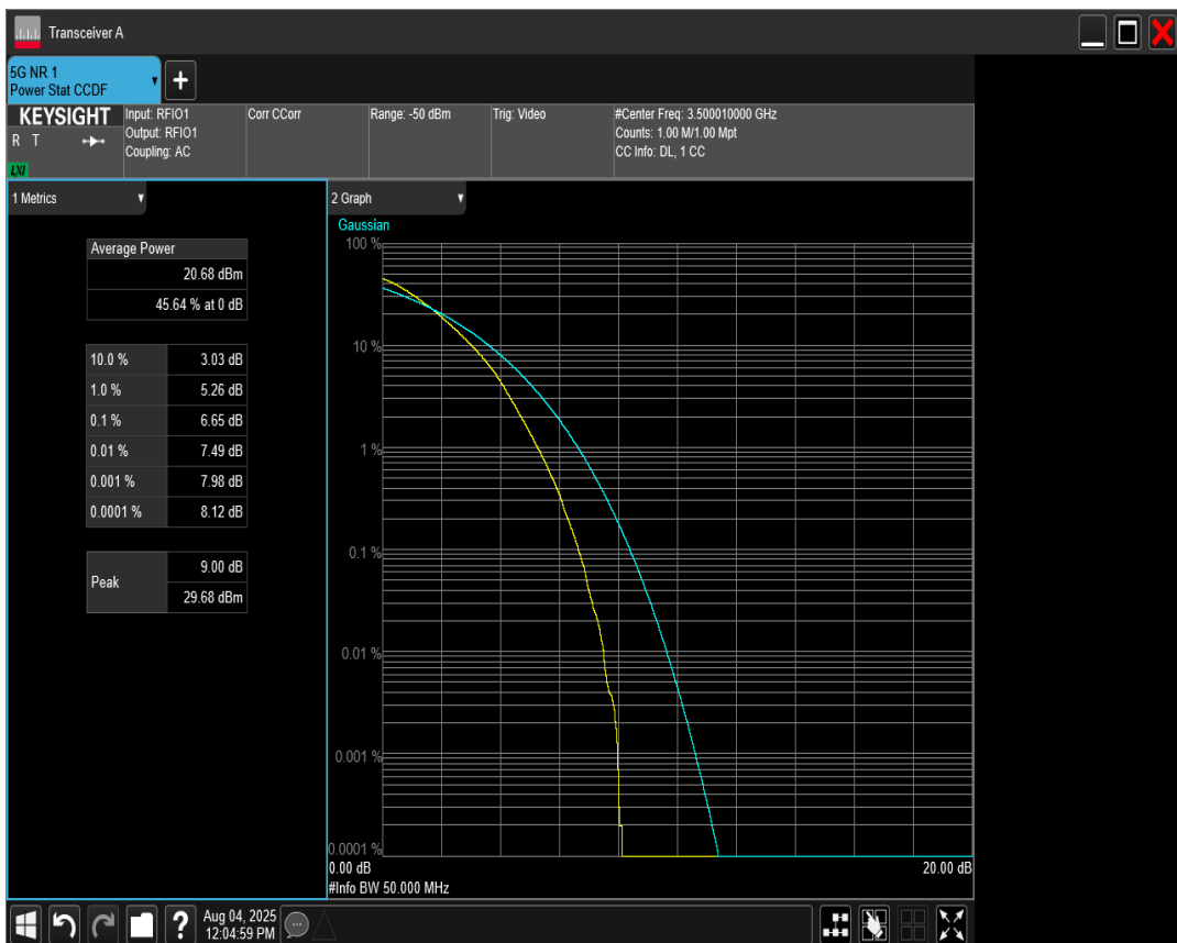
n77(3450-3550) SCS=30kHz DFT_QAM256 BW=50MHz Channel=635000 RB=128@0
