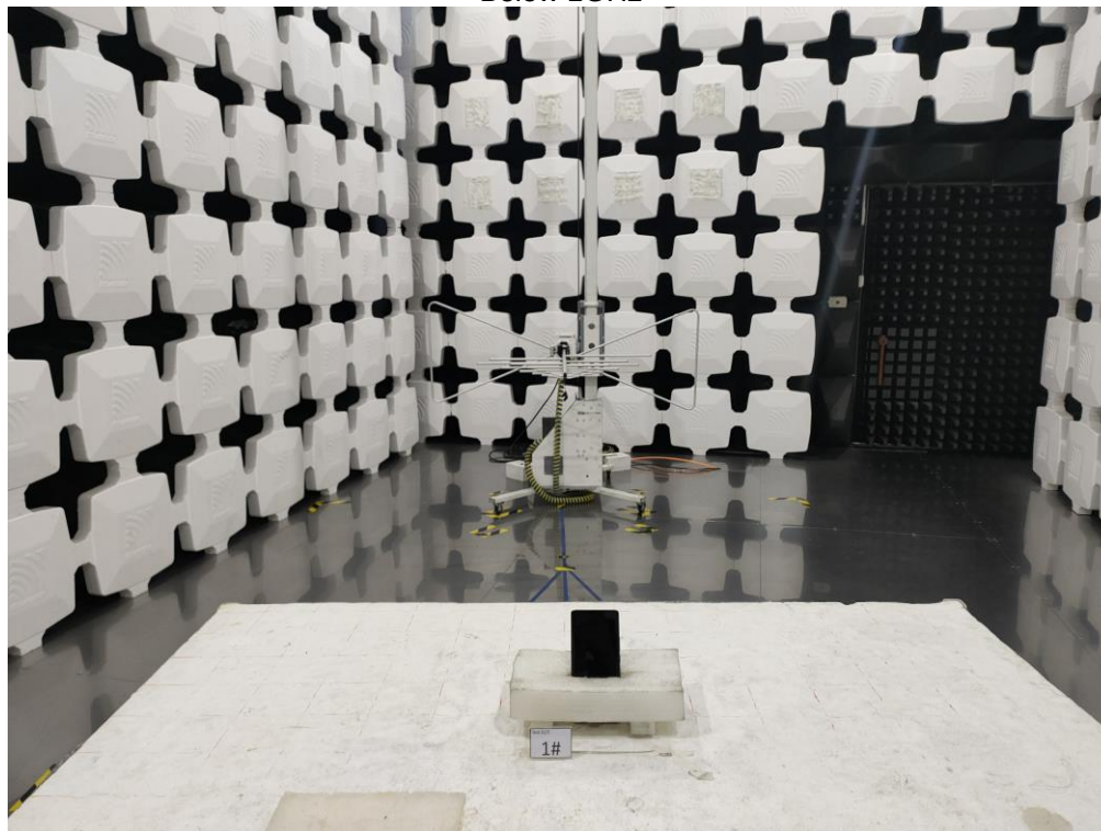
Radiated Spurious Emission Below 1GHz
