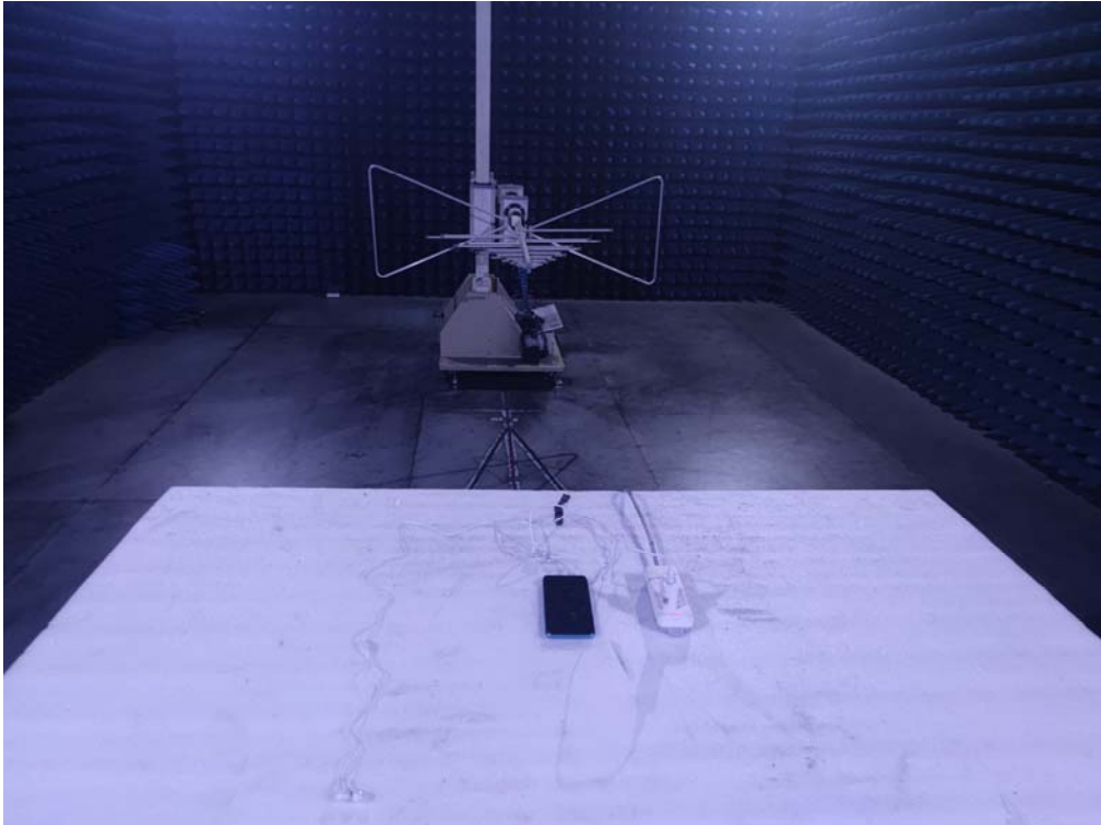
Photo of Radiated Emission Measurement (Below 1G)
