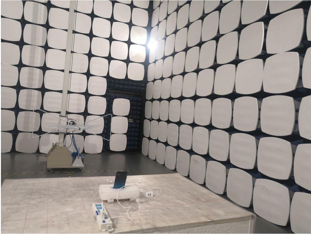
Radiated Spurious Emission Below 1GHz
