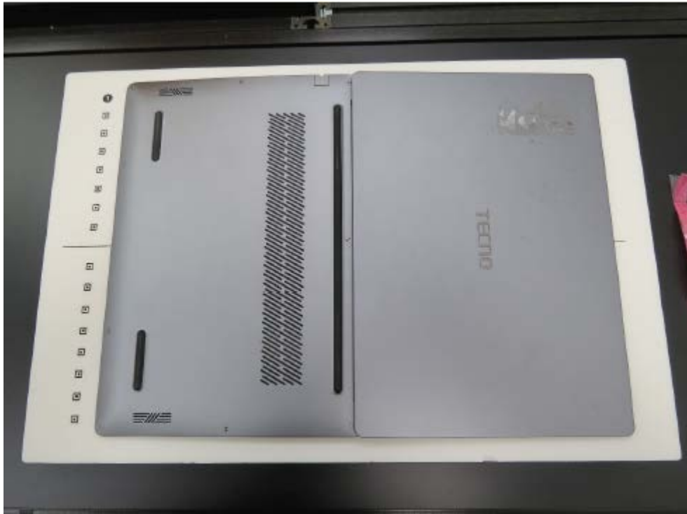
Back Side, the distance from EUT to the Phantom is 0mm
