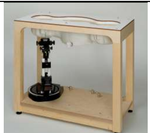
Fig. 8.7 Photo of SAM Twin Phantom
