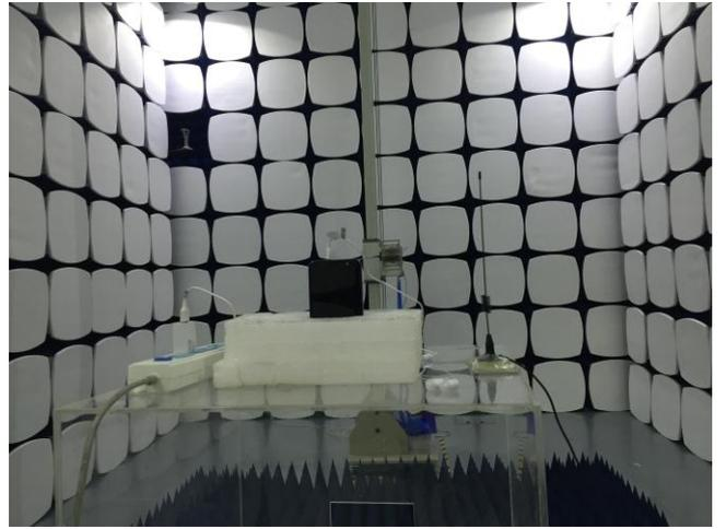
Radiated Spurious Emissions Test Setup Above
