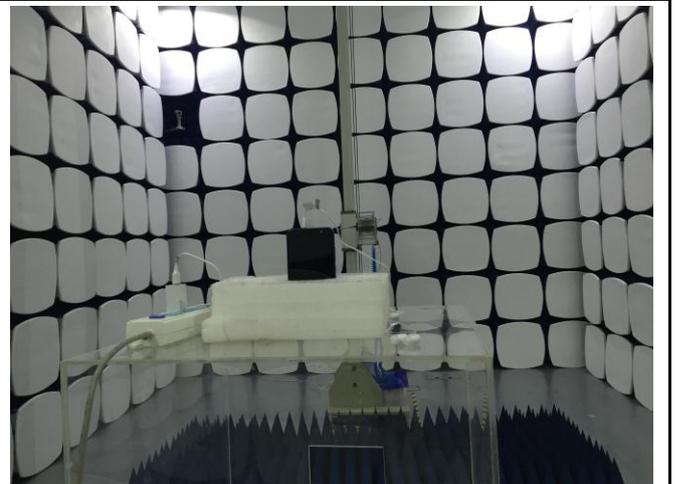
Radiated Spurious Emissions Test Setup Above
