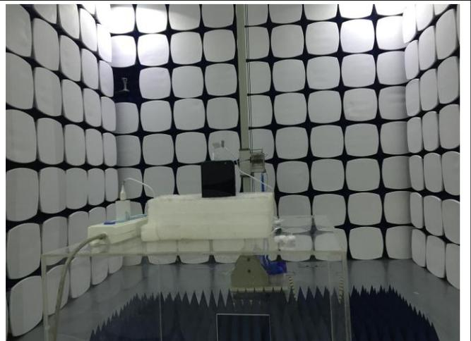
Radiated Spurious Emissions Test Setup Above
