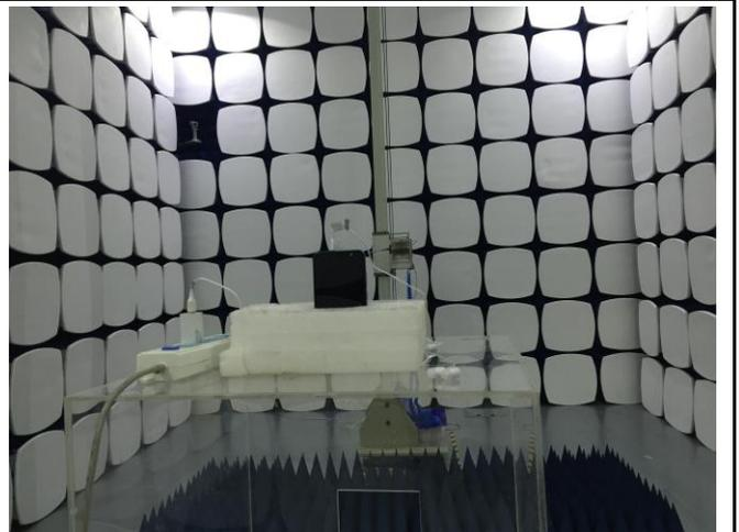
Radiated Spurious Emissions Test Setup Above
