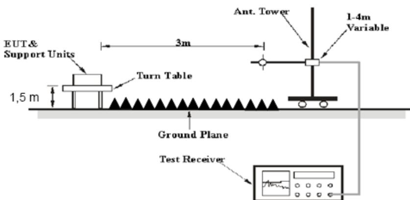
The radiated emission tests were performed in the 10 meters chamber test site for the range 30MHz to 1GHz and the 3 meters chamber test site for above 1GHz, using the setup accordance with the ANSI C63.10-2013. The specification used was the FCC 15.209, and FCC 15.247 limits.
