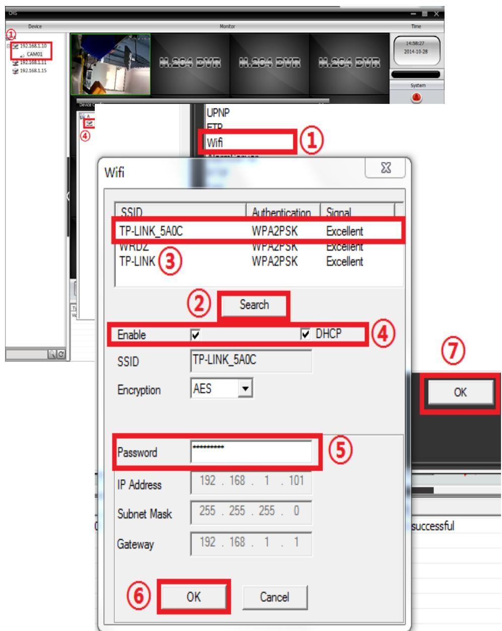
**Note:** After connecting the IP Camera to your Router, camera will request a restart. Please disconnect network cable and restart camera to allow the camera connect to your router in wireless.
