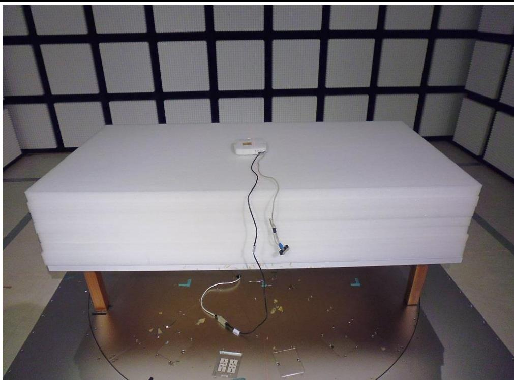
**Radiated Emission Above 1GHz Test (Adapter mode)**
