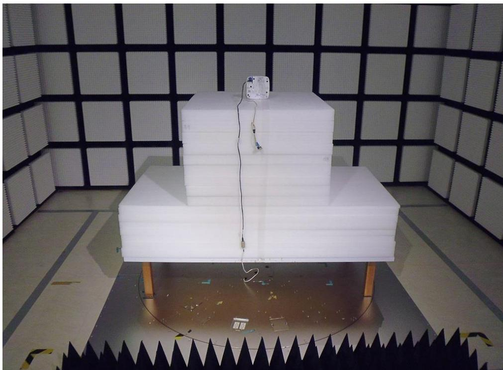
**Radiated Emission Above 1GHz Test (POE mode)**
