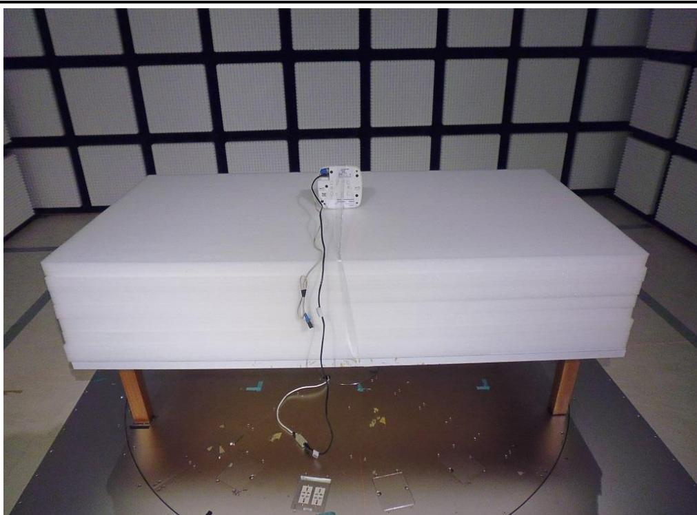
**Radiated Emission Above 1GHz Test (Adapter mode)**
