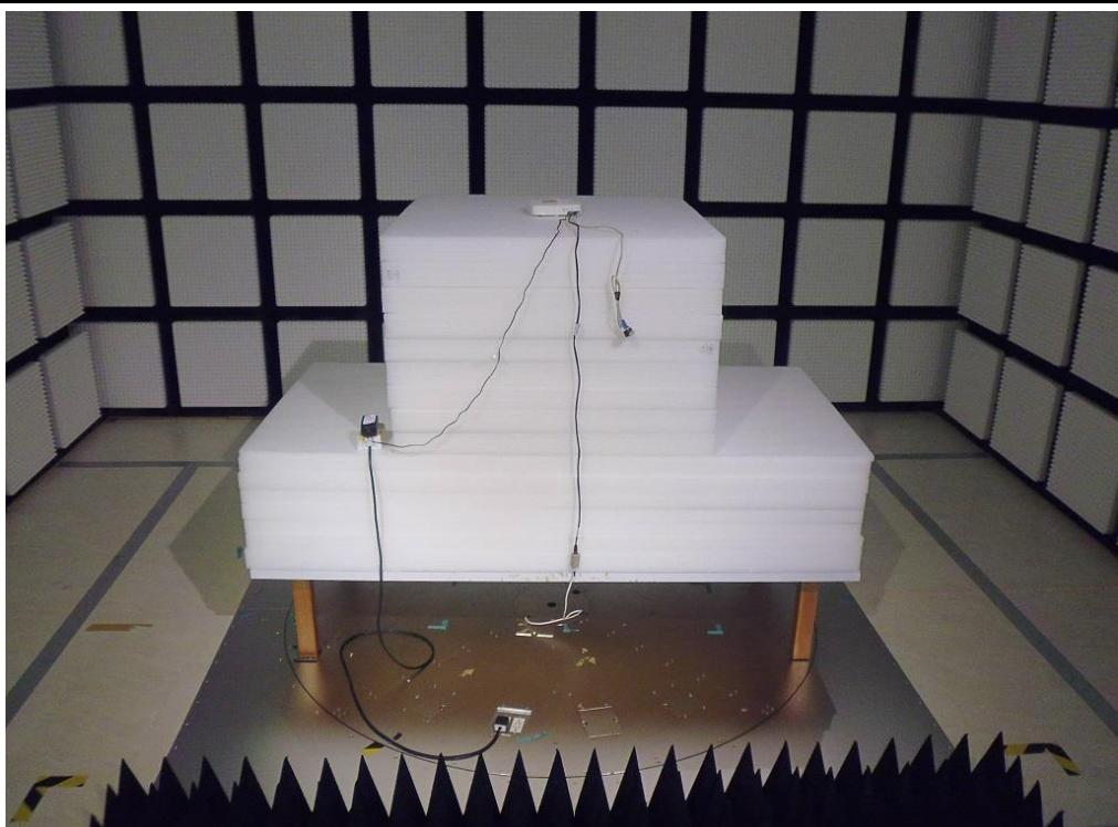
**Radiated Emission Above 1GHz Test (Adapter mode)**
