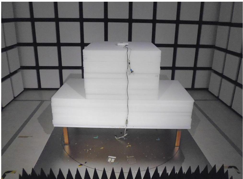
**Radiated Emission Above 1GHz Test (POE mode)**
