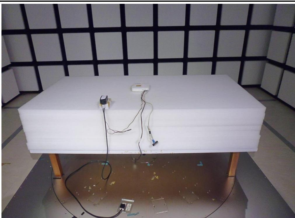
**Radiated Emission Below 1GHz Test (POE mode)**
