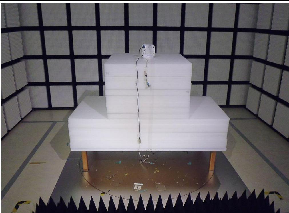
**Radiated Emission Above 1GHz Test (POE mode)**
