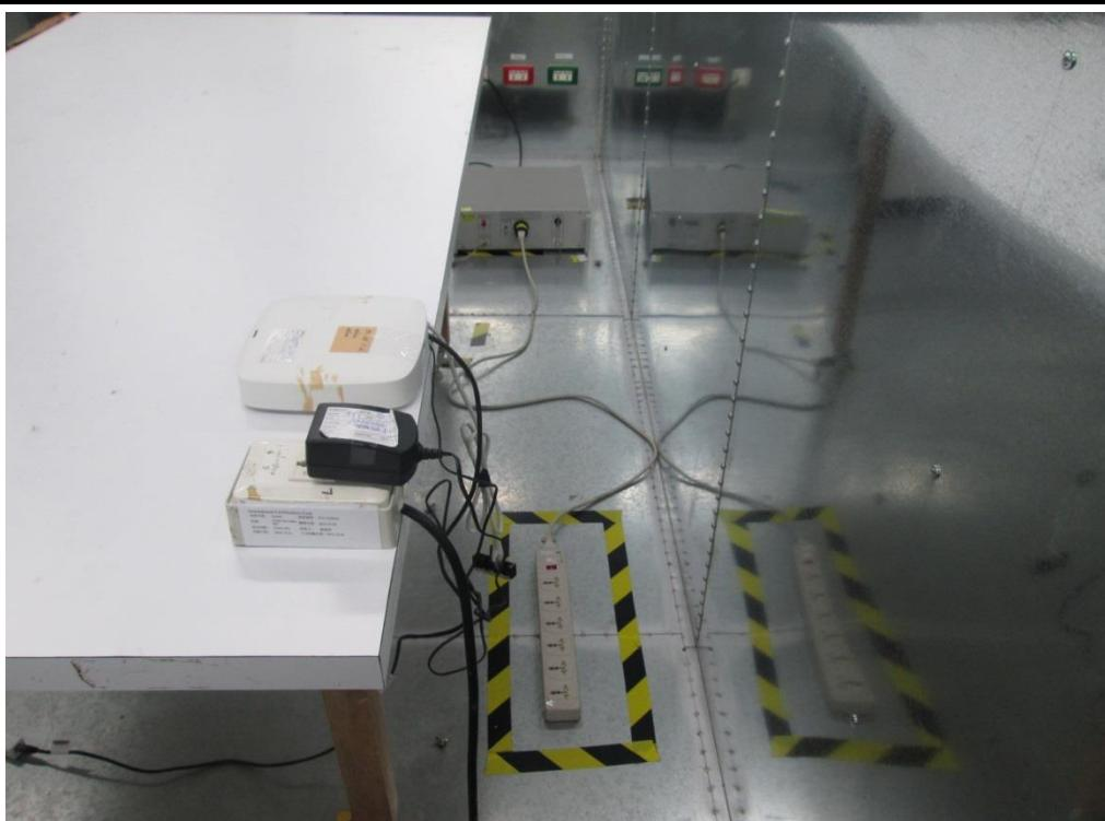
**Conducted Emission Test (POE mode)**
