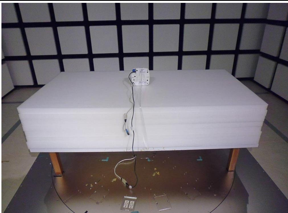
**Radiated Emission Above 1GHz Test (Adapter mode)**
