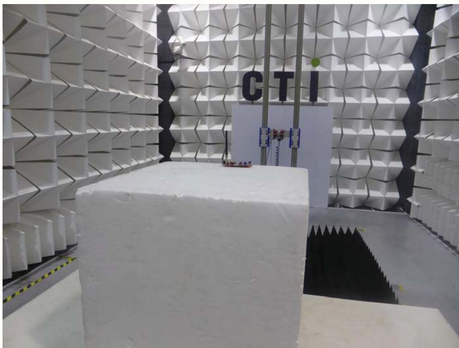
Radiated spurious emission Test Setup-2(Above 1GHz)
