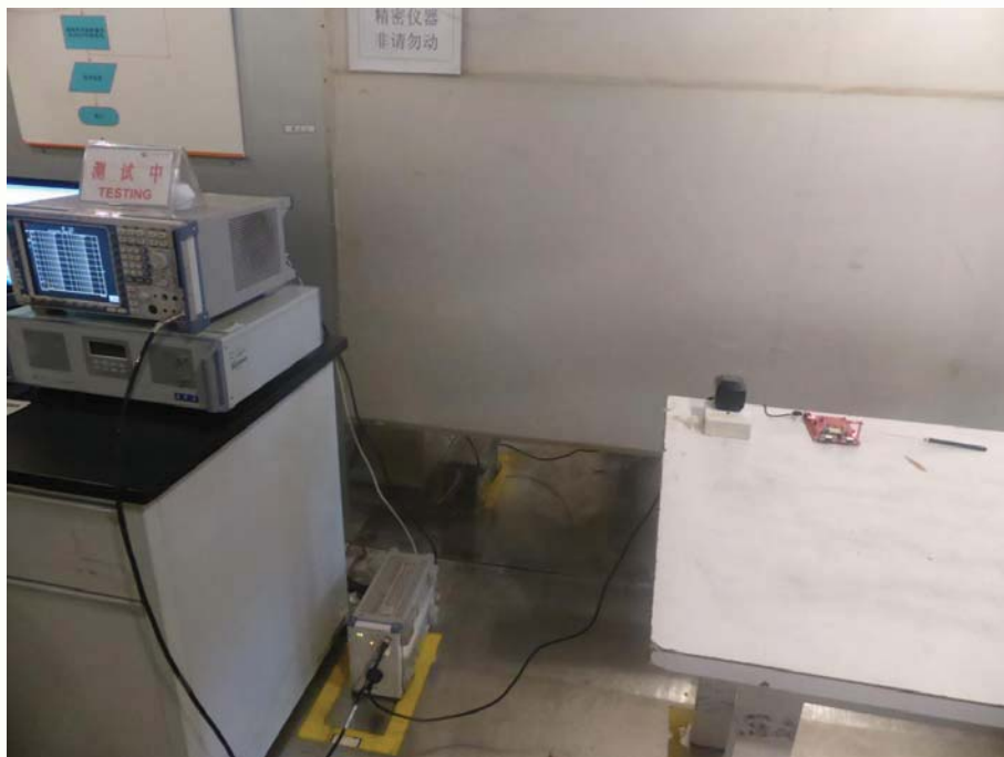
Conducted emission Test Setup
