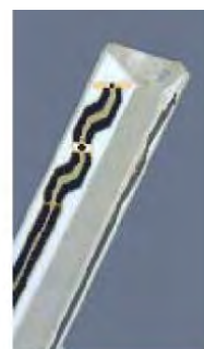
Figure E.2.2 Probe Thick-Film Technique
