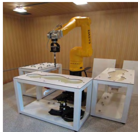
Figure E.7.1 DASY5 Test System
