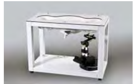
Figure E.5.1 SAM Twin Phantom
