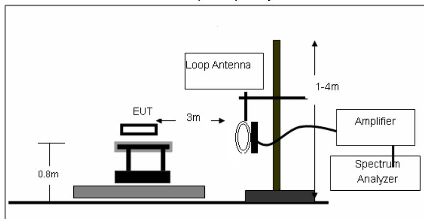
(2) Radiated Emission Test-Up Frequency 30MHz~1GHz
