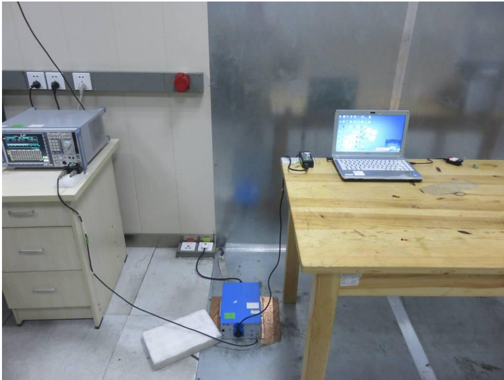
FCC RADIATED EMISSION TEST SETUP
