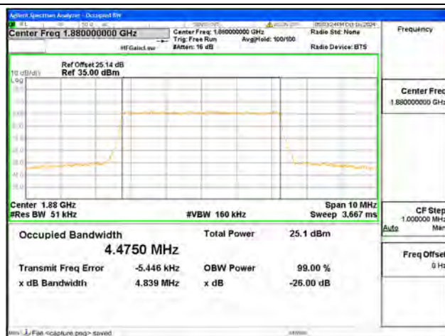
B2 / 5MHz / 16QAM/ Mid CH
