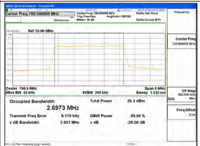
B12 / 3MHz / 64QAM/ Low CH
