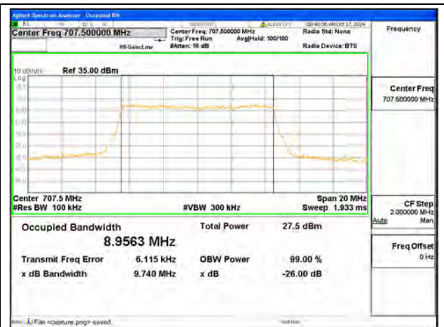
B12 / 10MHz / 16QAM/ Mid CH
