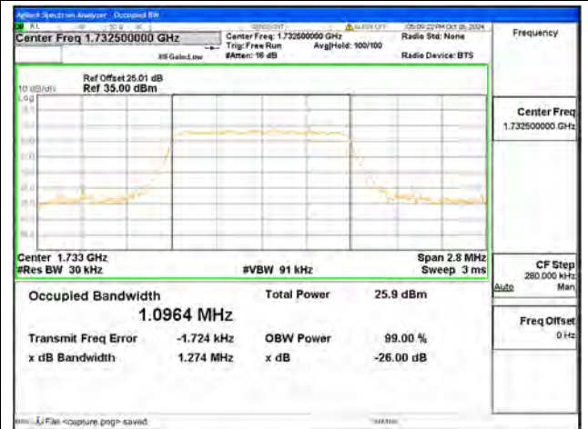
B4 / 1.4MHz / QPSK/ Mid CH
