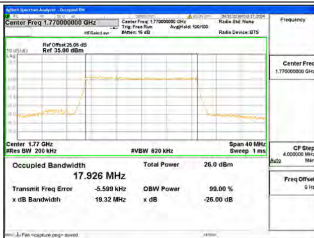
B66 / 20MHz / 16QAM/ High CH
