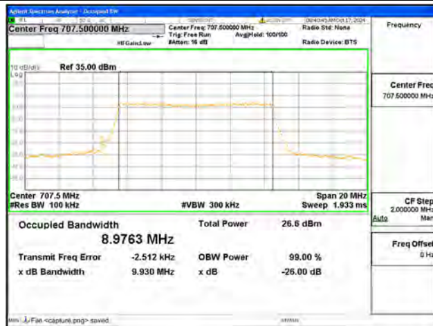
B12 / 10MHz / 64QAM/ Mid CH
