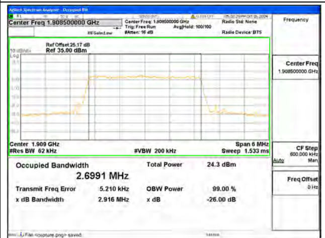
B2 / 3MHz / 64QAM/ High CH
