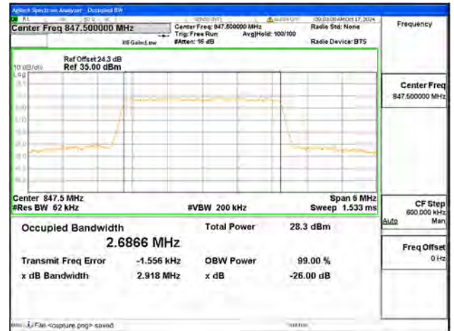
B5 / 3MHz / QPSK/ High CH
