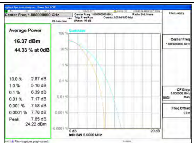
B2 / 3MHz / Mid CH / 16QAM
