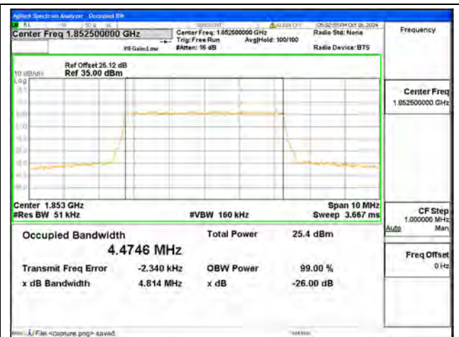
B2 / 5MHz / 16QAM/ Low CH
