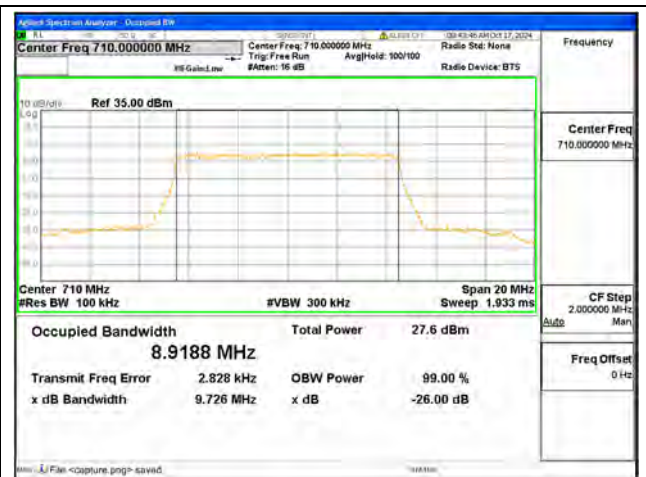
B17 / 10MHz / 16QAM/ Mid CH
