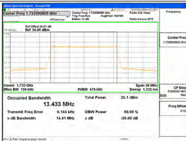
B4 / 15MHz / 16QAM/ Mid CH
