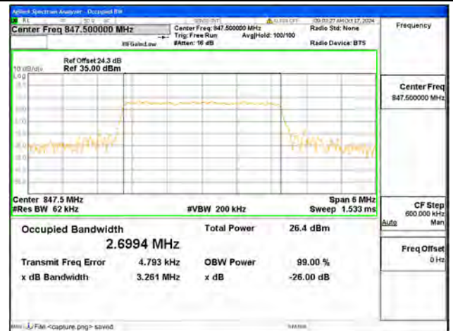
B5 / 3MHz / 64QAM/ High CH
