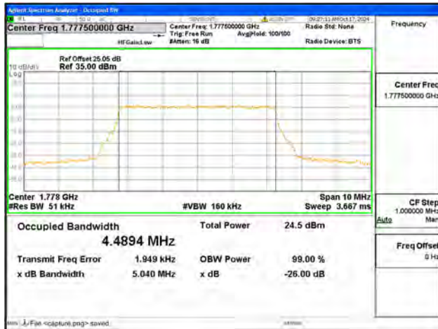
B66 / 5MHz / 64QAM/ High CH
