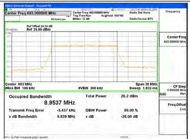
B71 / 10MHz / 64QAM/ High CH
