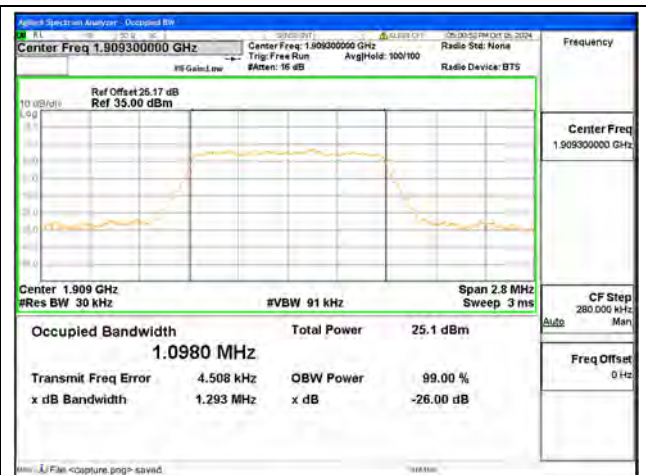
B2 / 1.4MHz / 16QAM/ High CH
