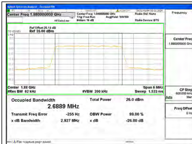
B2 / 3MHz / QPSK/ Mid CH
