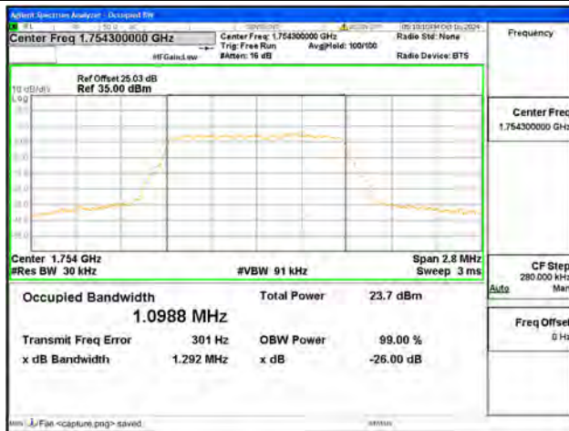
B4 / 1.4MHz / 64QAM/ High CH
