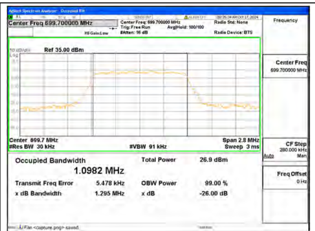
B12 / 1.4MHz / 16QAM/ Low CH
