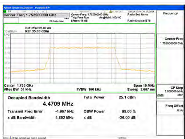
B4 / 5MHz / 16QAM/ High CH
