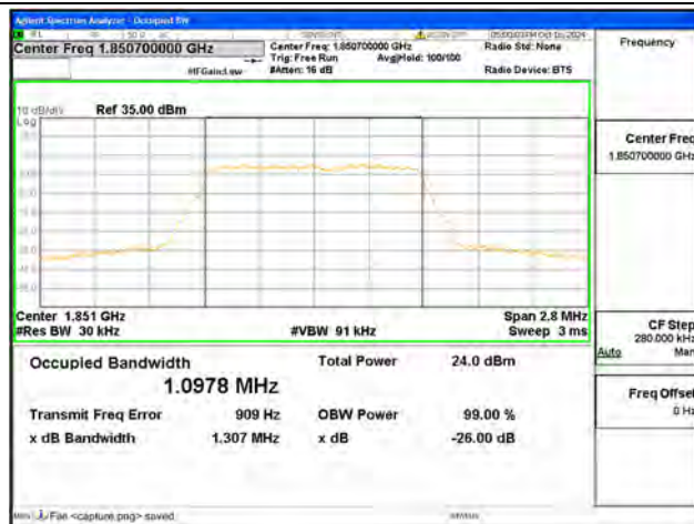
B2 / 1.4MHz / 64QAM/ Low CH
