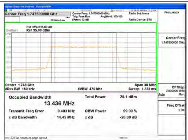
B4 / 15MHz / 16QAM/ High CH
