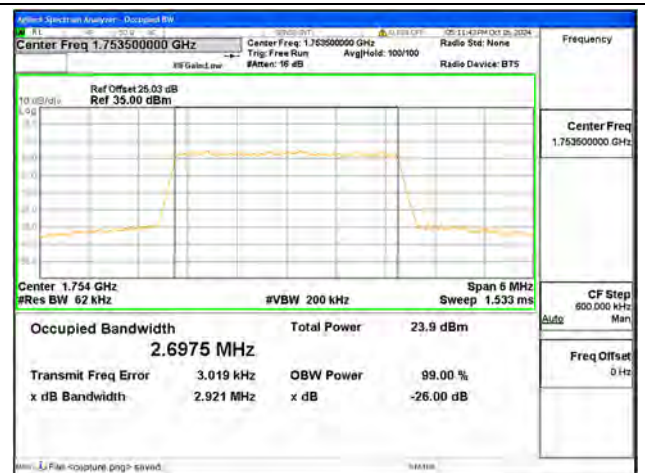
B4 / 3MHz / 64QAM/ High CH
