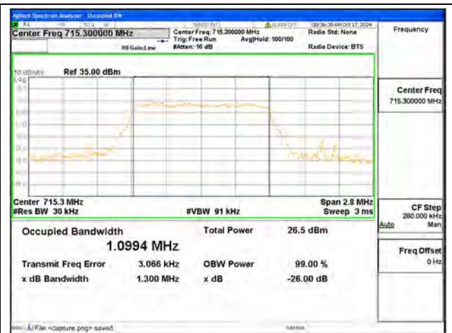
B12 / 1.4MHz / 16QAM/ High CH
