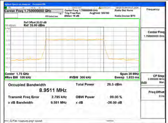
B4 / 10MHz / QPSK/ High CH
