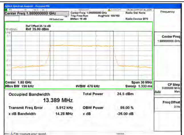
B2 / 15MHz / 64QAM/ Mid CH
