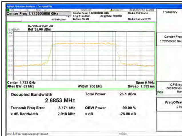
B4 / 3MHz / QPSK/ Mid CH
