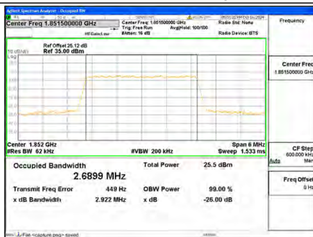
B2 / 3MHz / 16QAM/ Low CH
