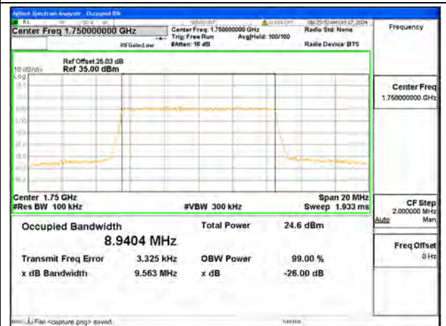
B4 / 10MHz / 64QAM/ High CH
