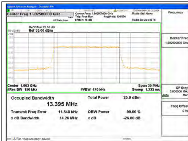
B2 / 15MHz / QPSK/ High CH
