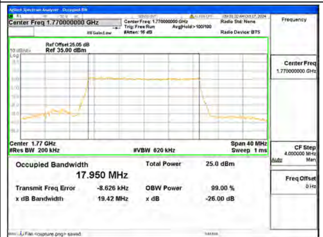
B66 / 20MHz / 64QAM/ High CH
