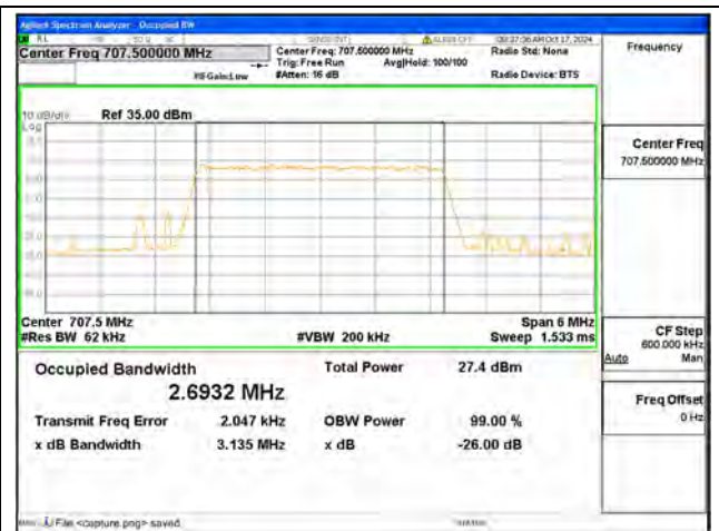
B12 / 3MHz / 16QAM/ Mid CH
