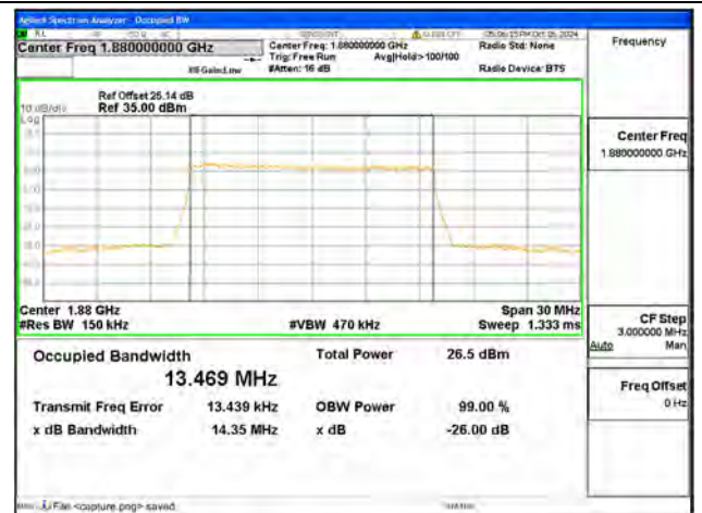
B2 / 15MHz / QPSK/ Mid CH
