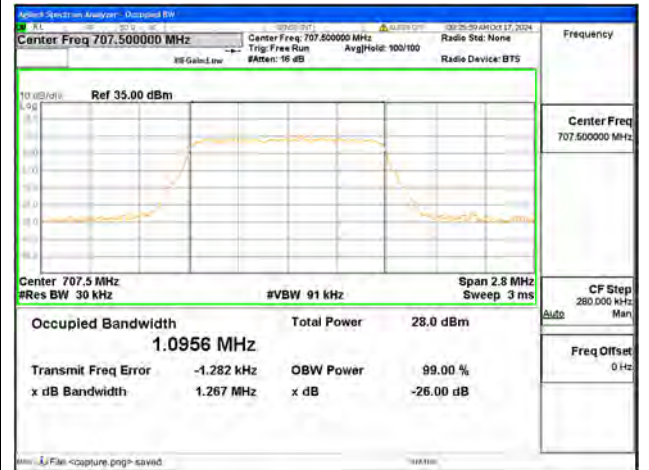
B12 / 1.4MHz / QPSK/ Mid CH
