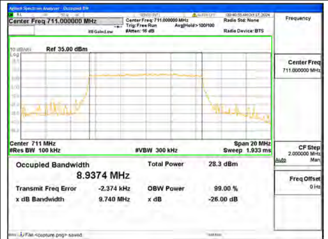
B12 / 10MHz / QPSK/ High CH
