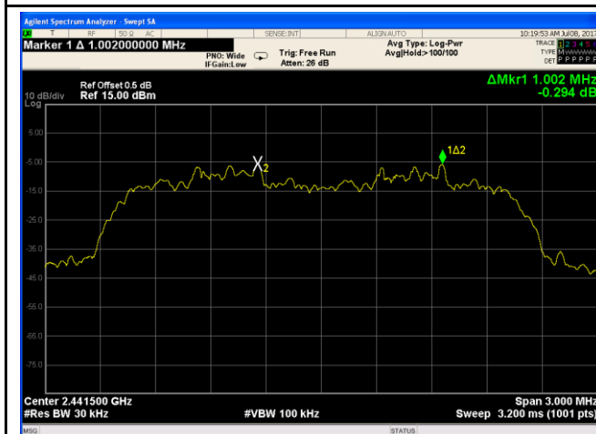
\pi/4 DQPSK - Middle Channel
