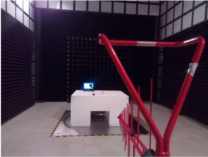
Radiated Emissions – Front View (Below 1 GHz)
