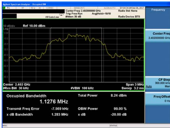
20dB Bandwidth plot on channel 39 (3Mbps)
