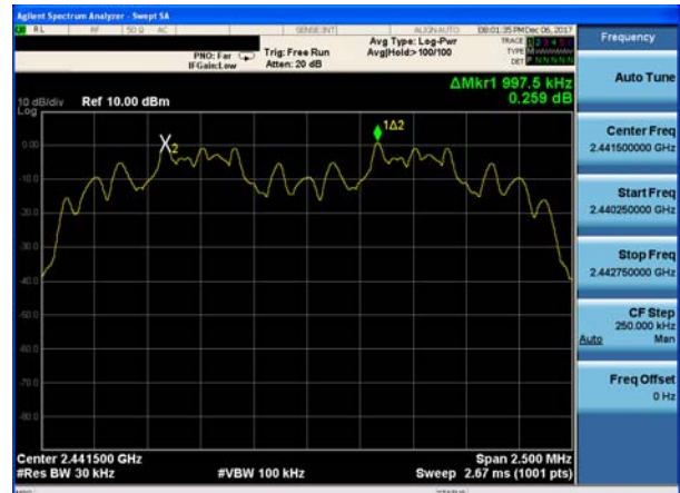
(2Mbps) Channel Separation plot on channel 77-78
