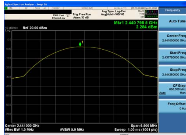
Peak output Power plot on channel 78 (2Mbps)
