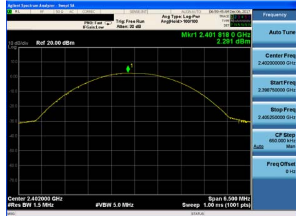
Peak output Power plot on channel 39 (2Mbps)
