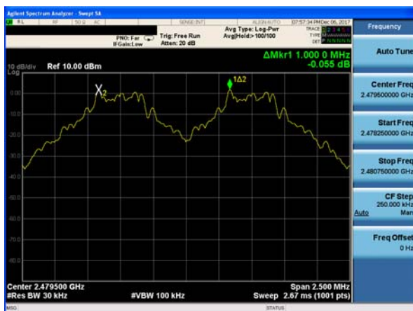
(1Mbps) Channel Separation plot on channel 77-78
