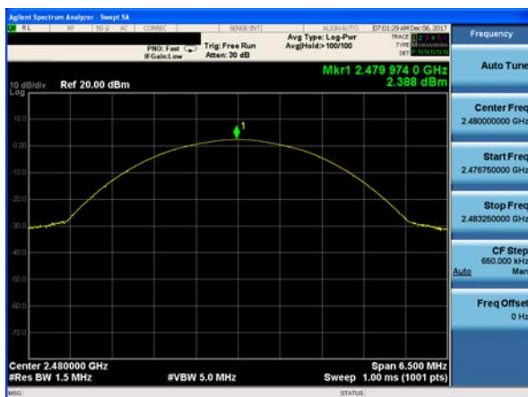
Peak output Power plot on channel 78 (3Mbps)
