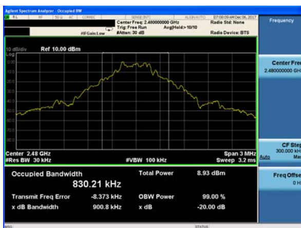
20dB Bandwidth plot on channel 78 (1Mbps)
