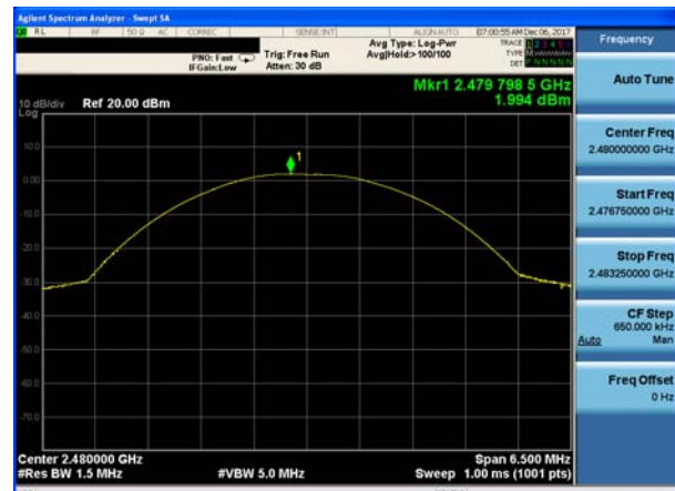
Peak output Power plot on channel 78 (2Mbps)
