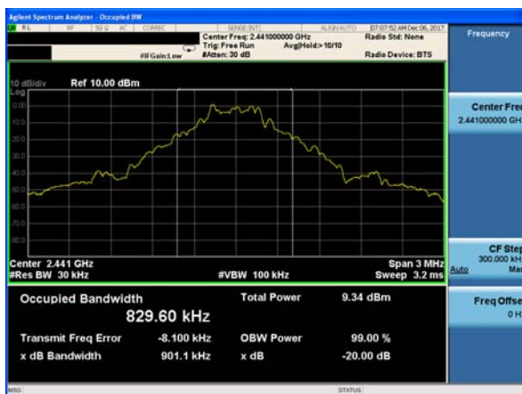
20dB Bandwidth plot on channel 78 (1Mbps)
