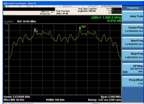
(2Mbps) Channel Separation plot on channel 77-78
