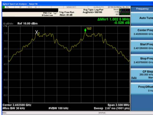
(1Mbps) Channel Separation plot on channel 39-40
