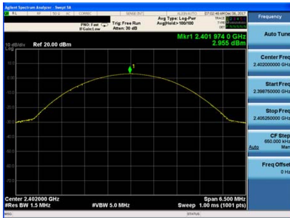
Peak output Power plot on channel 39 (3Mbps)
