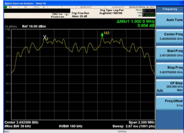
(2Mbps) Channel Separation plot on channel 39-40
