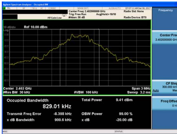
20dB Bandwidth plot on channel 39 (1Mbps)
