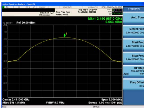
Peak output Power plot on channel 78 (3Mbps)
