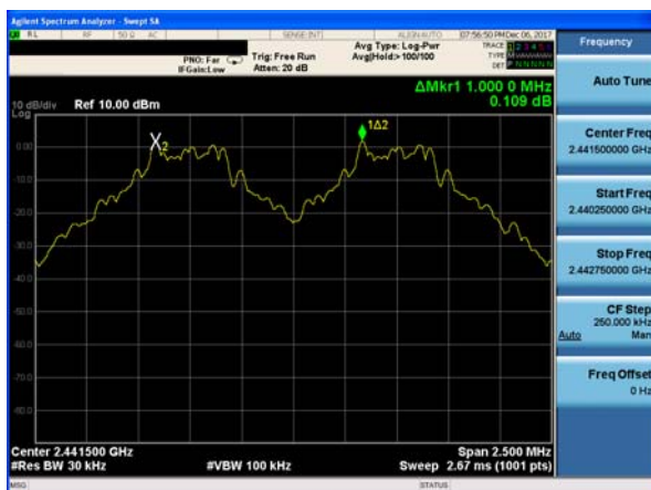
(1Mbps) Channel Separation plot on channel 77-78
