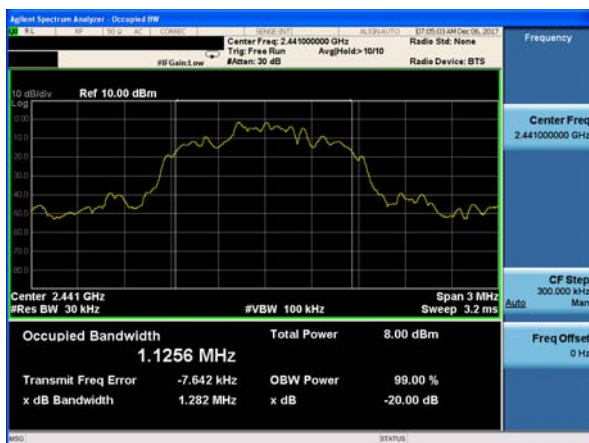
20dB Bandwidth plot on channel 78 (3Mbps)
