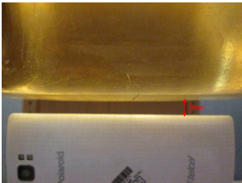
Body-worn Left Setup Photo (10mm)
