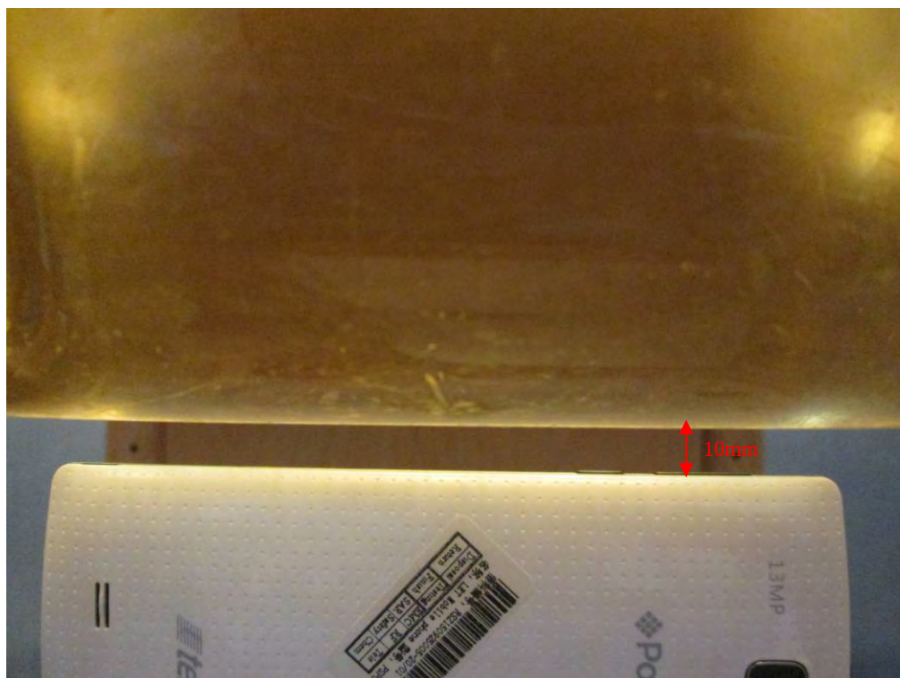
Body-worn Left Setup Photo (10mm)
