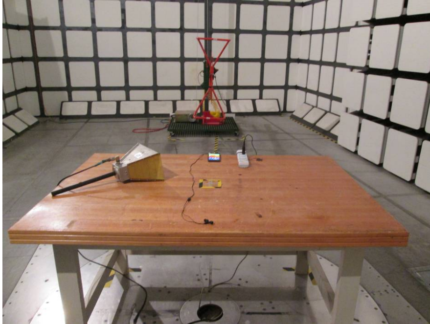
Radiated Emissions –Front View (30-1000 MHz)
