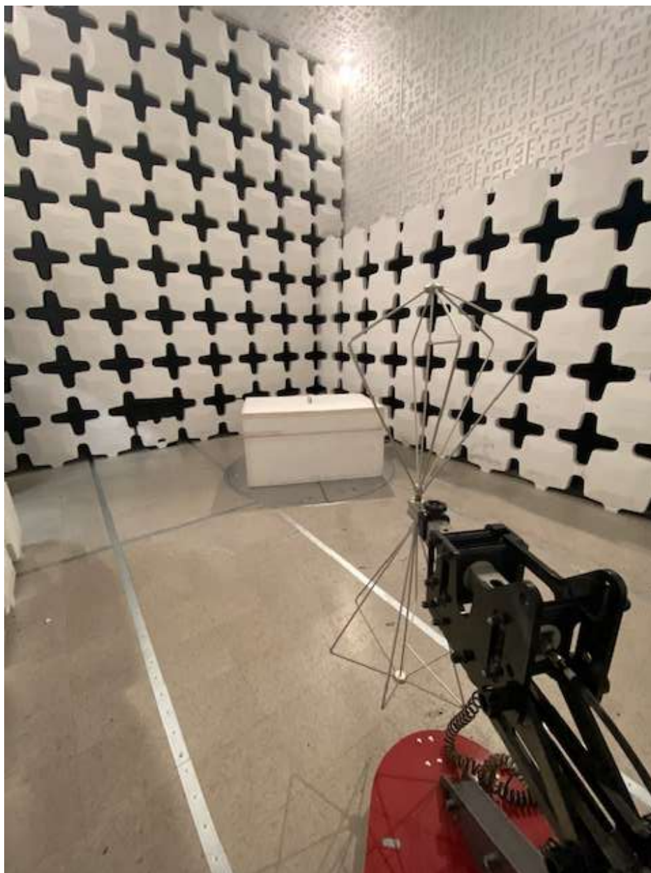
Figure 3. Radiated Emissions Test Setup, 30 MHz to 200 MHz
