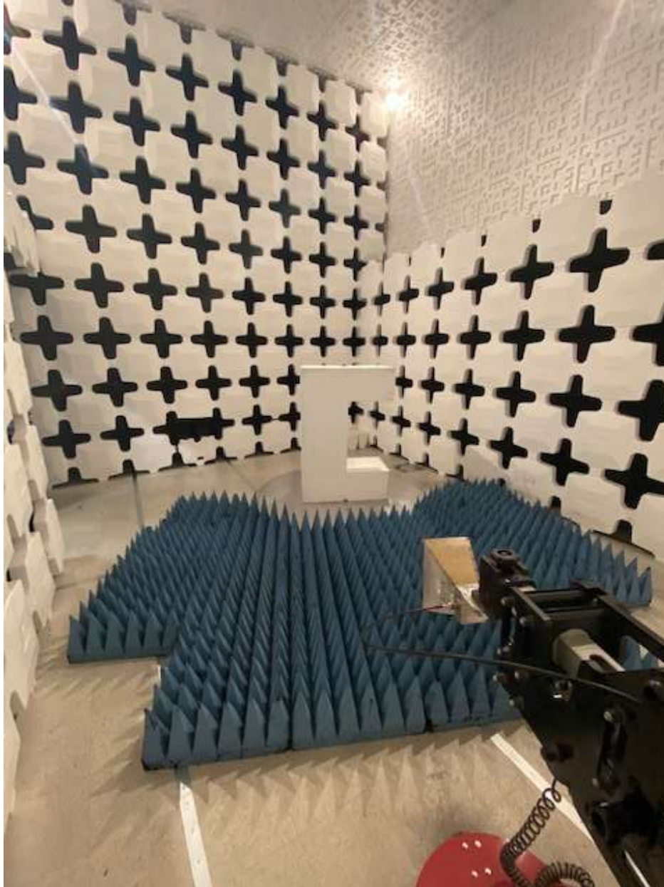
Figure 5. Radiated Emission Test Setup, above 1 GHz
