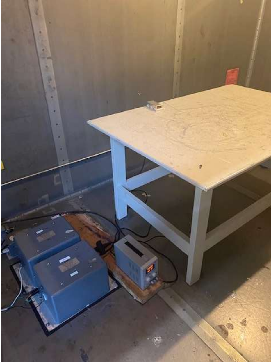
Figure 6. Conducted Emissions Test Setup
