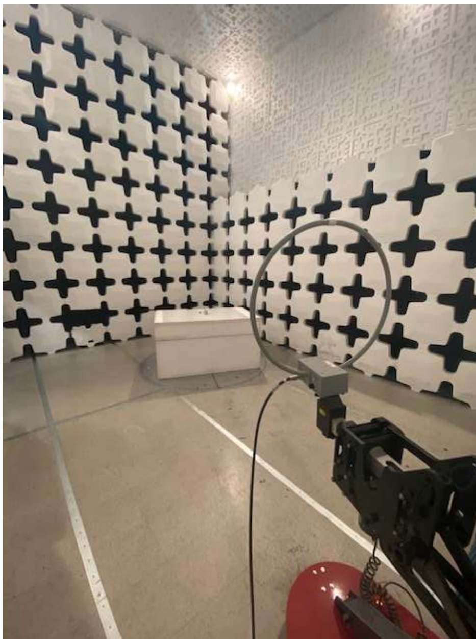
Figure 2. Radiated Emissions Test Setup, 150 kHz to 30 MHz
