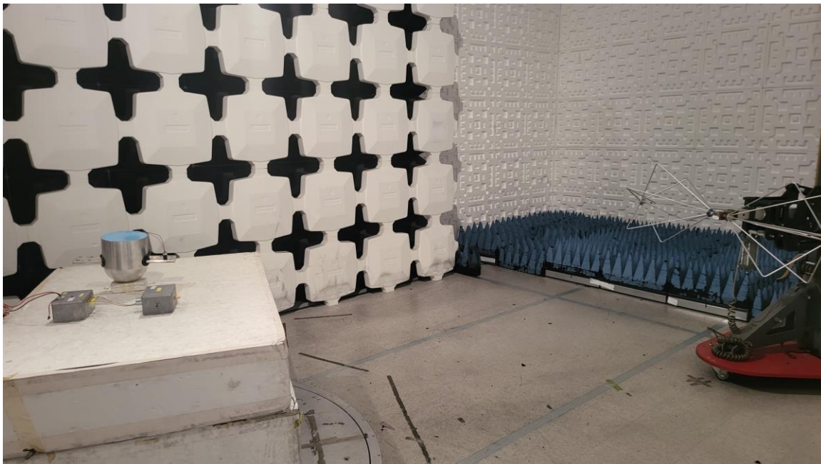
Figure 3. Radiated Emissions Test Setup, 30 MHz to 200 MHz
