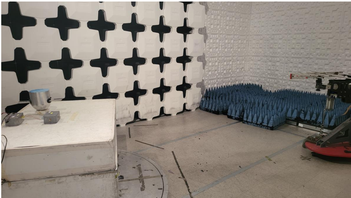
Figure 4. Radiated Emissions Test Setup, 200 MHz to 1GHz
